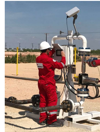
Emerging New Technology - MultiPhase Flow Meter (MPFM)
