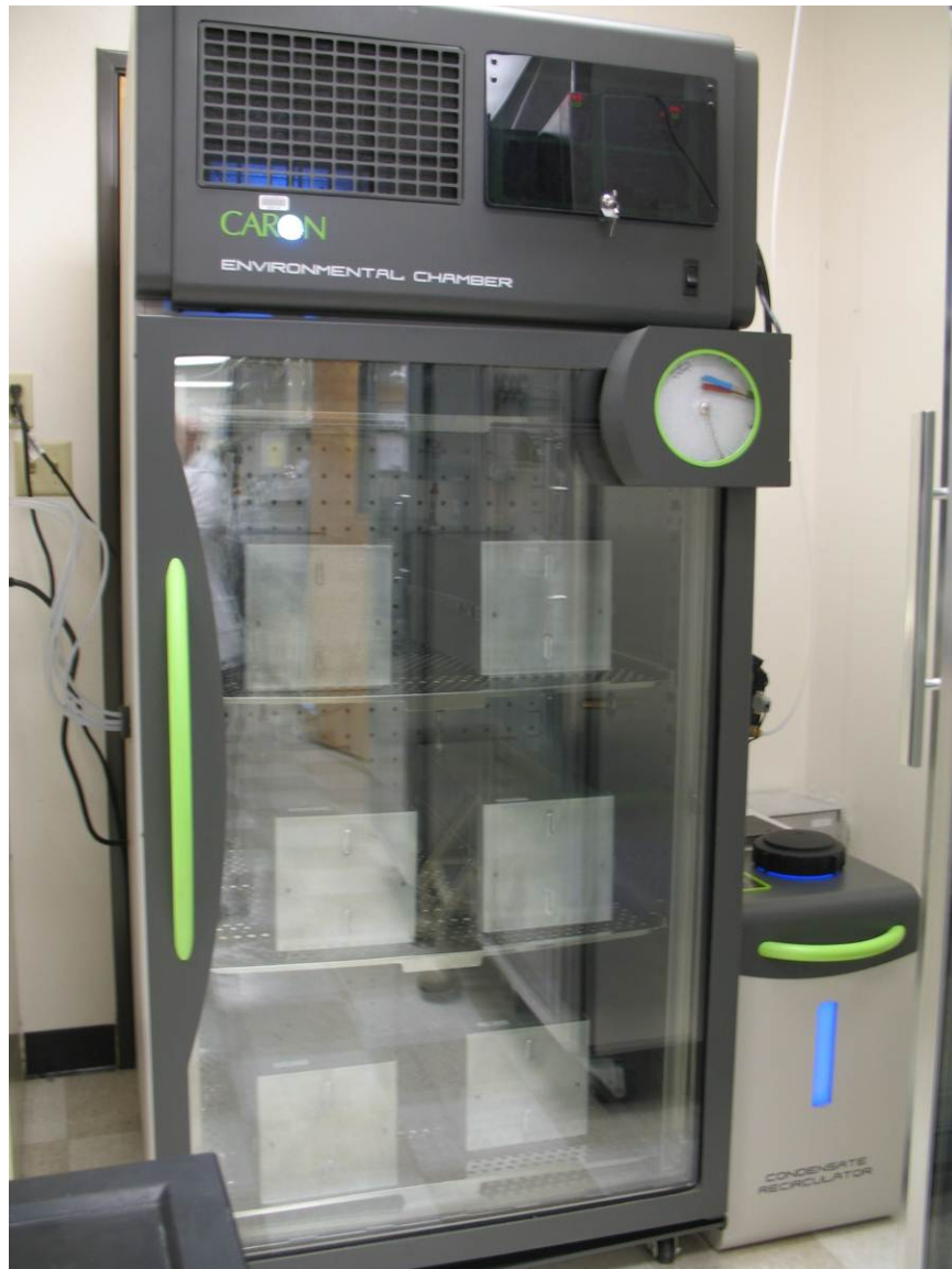
Figure 1.5 Environmental Chamber with Small Sampling Chambers Inside
