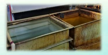
Stripping tanks – remove old chrome layer off of parts, concentration of chrome can increase over time, some tanks are electrolytic
