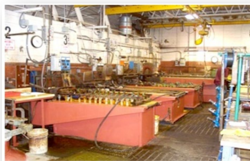
Hard chrome electroplating baths. (Photo courtesy of NIOSH).
