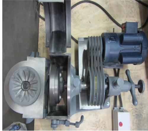
B. Plate grinder for pulverization.
