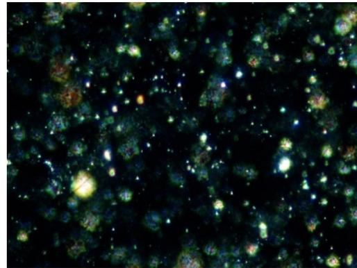
B. Pulverized salt matrix and chalk (bright particles) after mixing. 100X mag, PLM, crossed polars.
