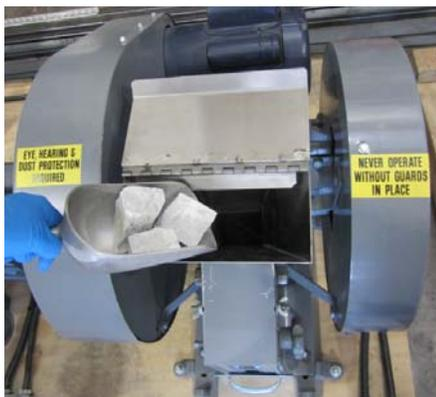
**Figure E-2. Lift out the feeder plate.**
