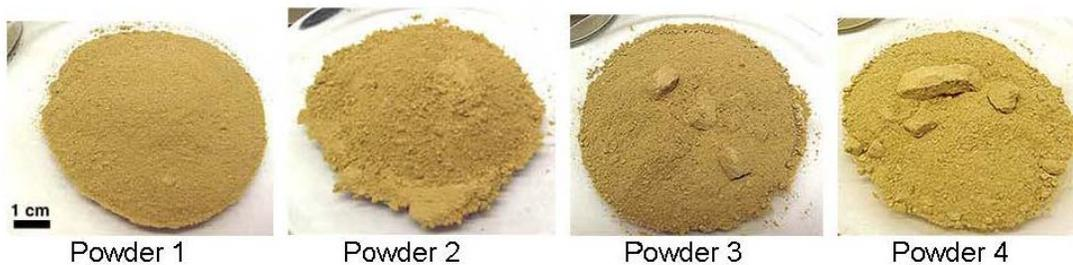
The analysis of the particle size distribution showed differences among the powders in the weight percentages of different particle size fractions. The particle size distribution of powders prepared by the four laboratories is shown in Figure B-8. The data presented are the averages of three replicate aliquots from each of the powders produced by the four laboratories.
