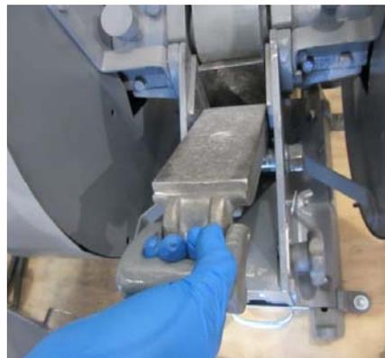
**Figure E-3. Loosen debris with brush.**
