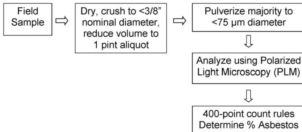
ARB staff supervised the field material preparation prior to distribution to the laboratories (Figure B-2). The sample was dried in a constant-temperature oven for
