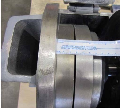
Figure F-2. Loosen the locking handle.
