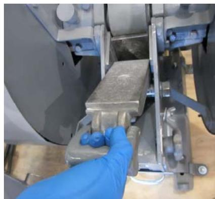
**Figure E-3. Loosen debris with brush.**
