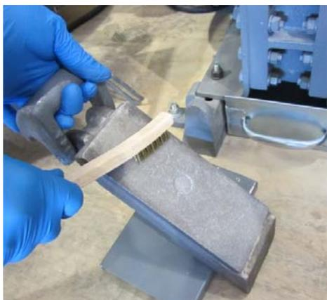
**Figure E-4. Wipe down the crusher.**
