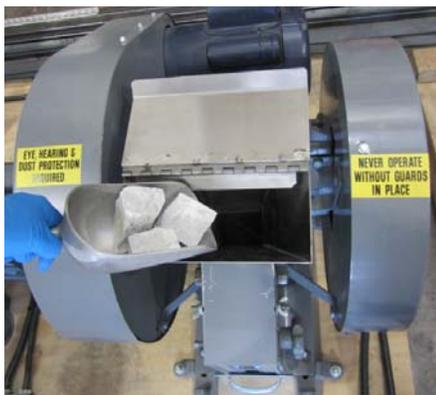
**Figure E-2. Lift out the feeder plate.**
