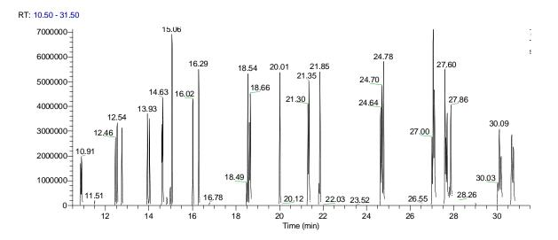
Figure 4. The Extracted Ion Chromatogram (EIC) of the Calibration Standard PAHs
