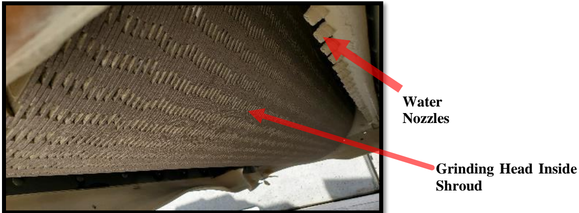
Fig. 2-5: Water Nozzles on Texture Planer
