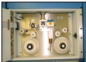
Beta attenuation monitor
