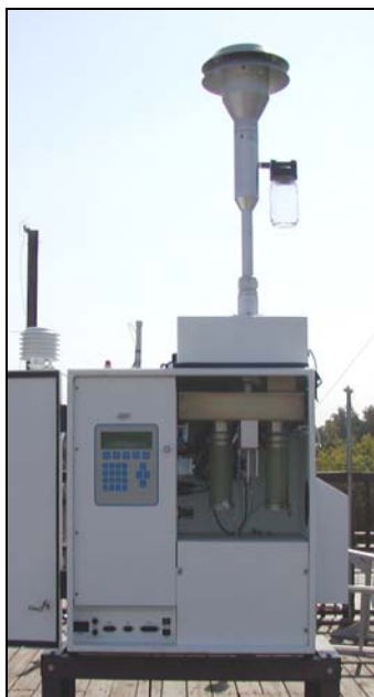
Federal reference method monitor
