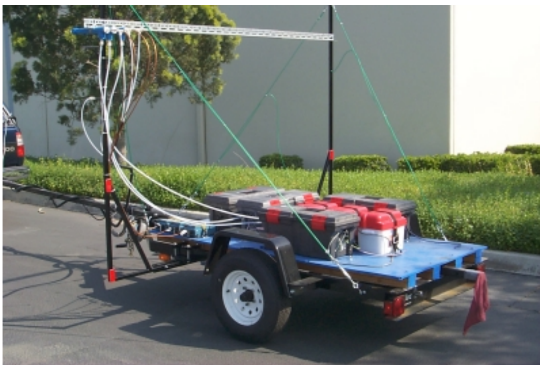
Figure 2-4. Photo of the trailer used to mount the isokinetic sampling probes and the DustTrak PM sensors.
