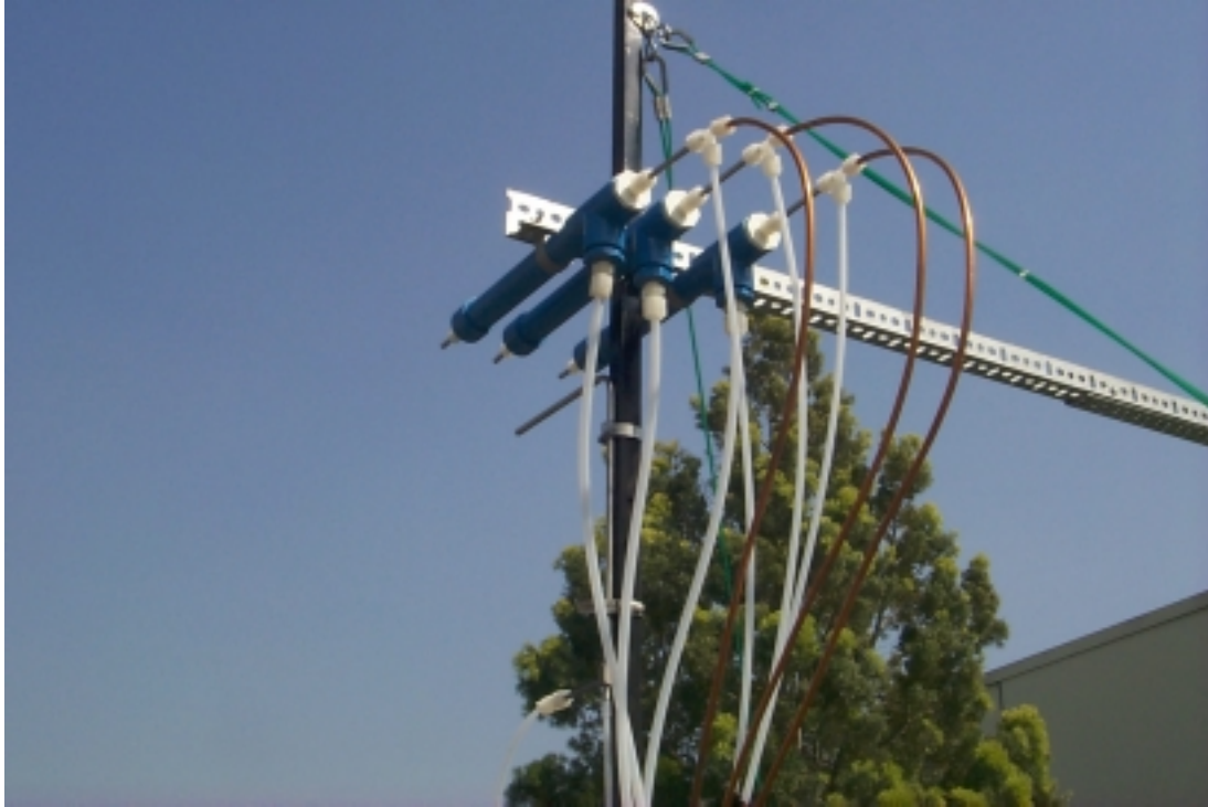
Figure 2-5. Close-up photograph of the isokinetic sampling probes.
