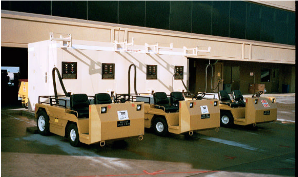
Photo of SuperCharge™ Station with three TUG M3A Electric Baggage Tractors connected for charge.
