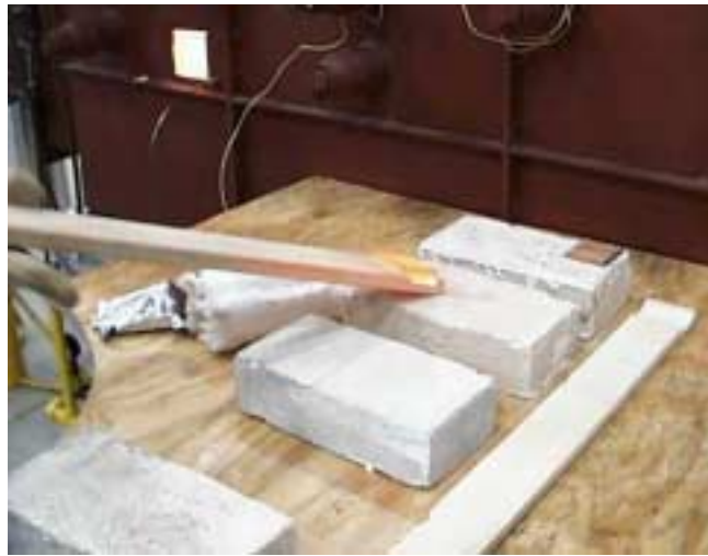
Figure 12. METAL SAMPLE AFTER REMOVAL FROM FURNACE (Trial test with steel surrogate sample pictured; ceramic fiber insulating blanket and aluminum tape is seen behind the fire bricks)
