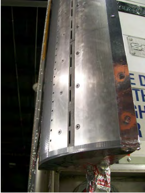
Figure 12. TAU Device Viewed from Rear of Trailer Looking Upward
