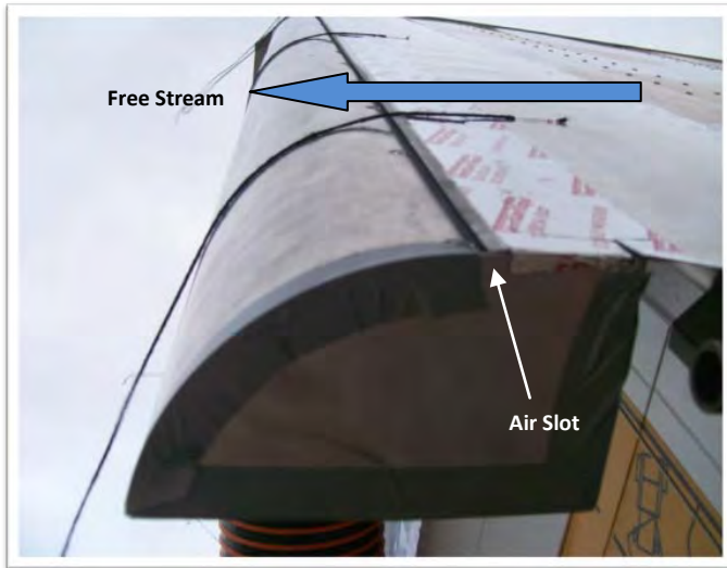
Figure 3. GTRI Device Viewed from Side of Trailer Looking Upward
