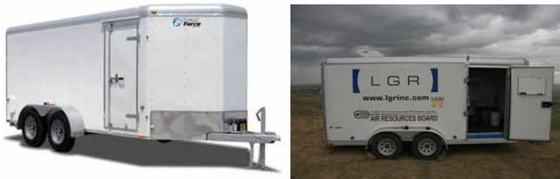
Figure 1. Trailer (Cargo Wagon; 7' wide) - contains several LGR Gas Analyzers and assorted metrology equipment to serve as the Mobile Emissions Laboratory.
