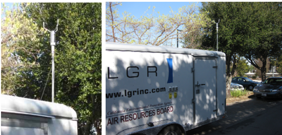
Figure 8. Sonic anemometer mounted on top of the Mobile Emissions Laboratory for measurements of wind direction and velocity.
