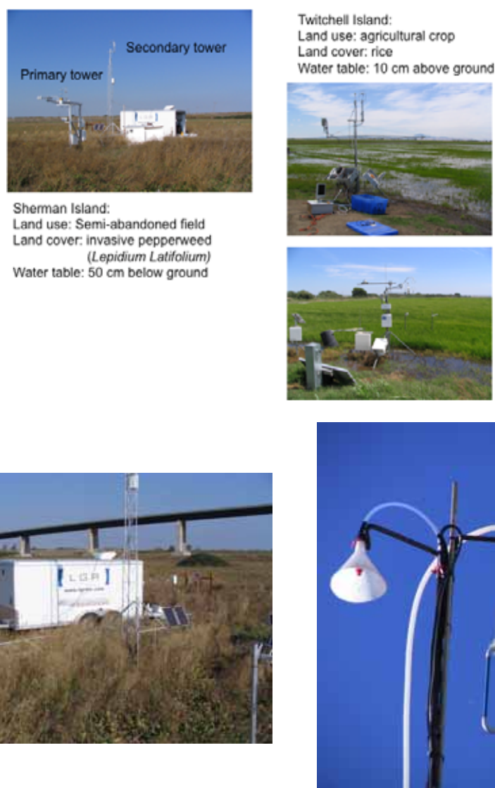
Figure 27. Setup for measurements of methane, carbon dioxide and water vapor at multiple sites (Twitchell Island and Sherman Island) in the Sacramento-San Joaquin Delta recorded with the Mobile Emissions Laboratory (Fast Greenhouse Gas Analyzer, Dry Scroll Vacuum Pump, sonic anemometers). Note that for these measurements, the dual flux tower setup was supplied by UC Berkeley. The site at Twitchell Island was selected to investigate fluxes near rice paddies whereas the site near Sherman Island was a semi-abandoned field near invasive pepperweed.
