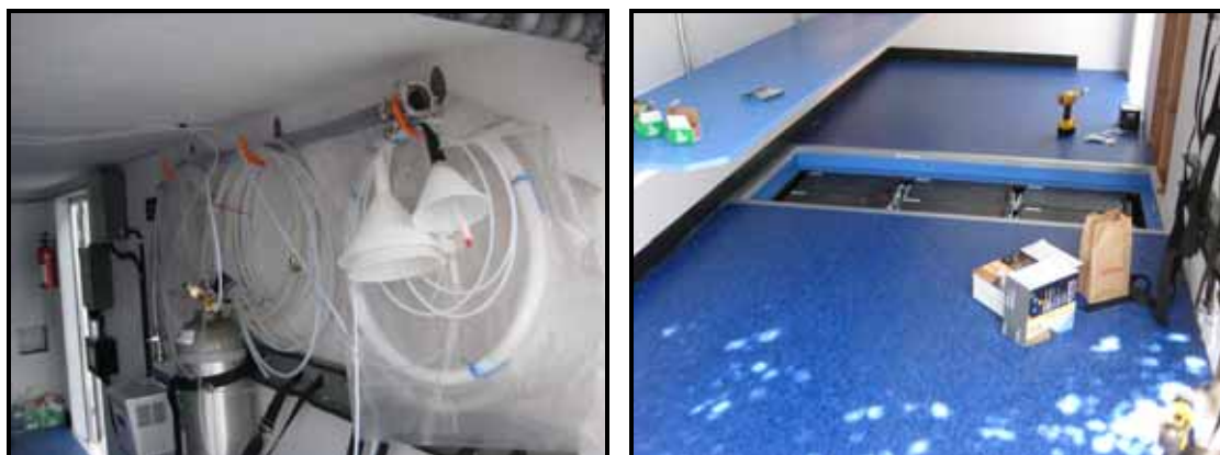
Figure 6. LGR's Multiport Inlet Unit (MIU) combined with long-length inlet lines (left) allow for measurements at multiple locations and at various distances (50 meters or longer) from the trailer.
