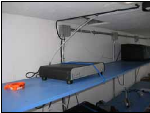
Figure 7. LGR's Multiport Input Unit (MIU) provides capability for 16 gas inputs to the Analyzer.
