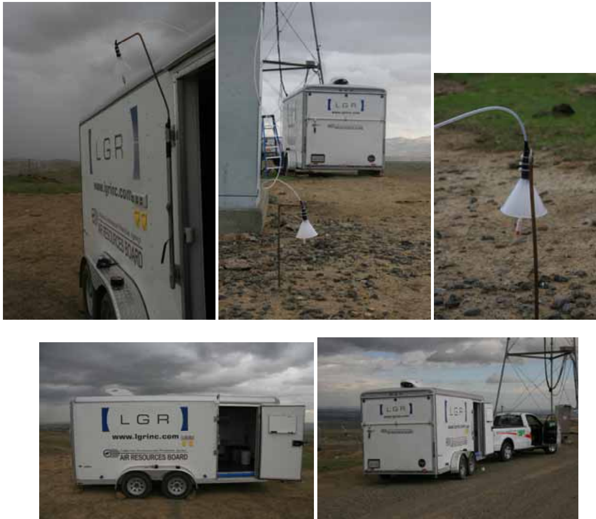
Figure 38. Mobile Emissions Laboratory deployment at the Altamont Landfill site to characterize fugitive methane emissions and quantify the flux of acetylene tracers.
