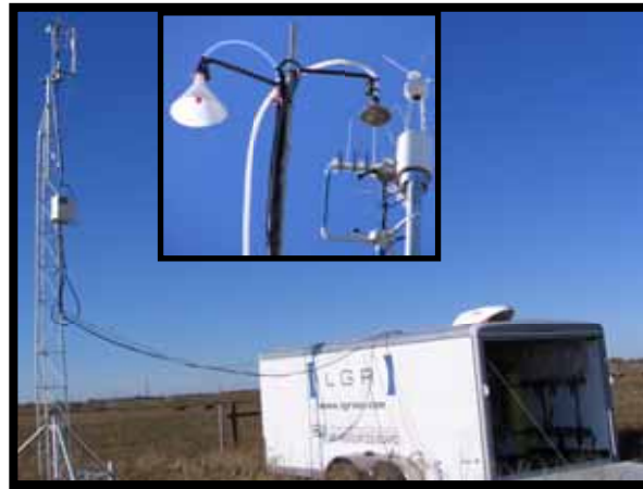
Figure 31. Water Vapor Isotope Analyzer and Water Vapor Isotope Standard Source deployed at Sherman Island, California, for continuous, unattended, automatic measurements of water isotopes.
