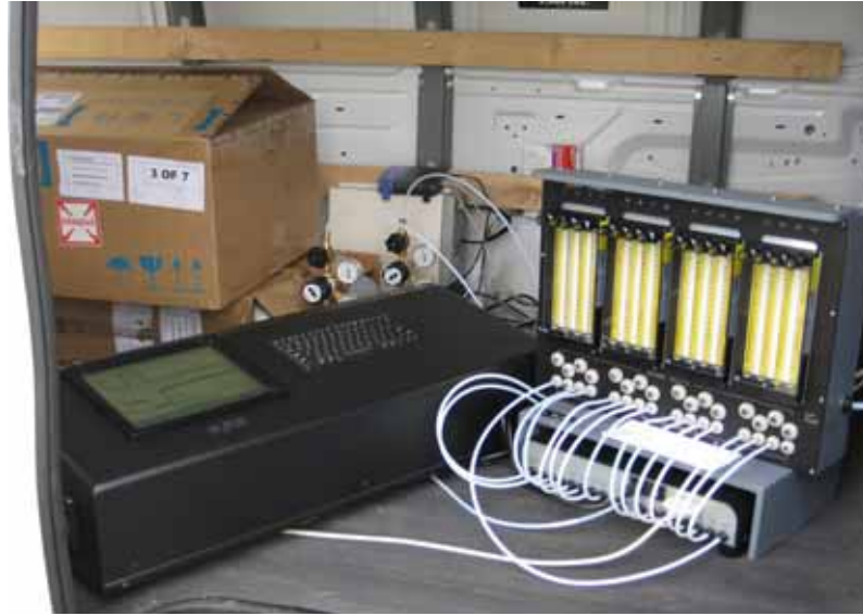
Figure 35. Carbon Dioxide Isotope Analyzer, Inlet manifold, and Multiport Input Unit (MIU) used to sample from multiple inlets automatically using a single analyzer.
