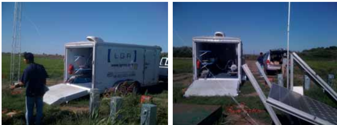
Figure 26. LGR Mobile Emissions Lab deployed with (UC Berkeley) Professors Goldstein and Baldocchi for simultaneous methane, carbon dioxide and water vapor flux measurements at Twitchell Island.
