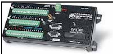
Figure 10. Data logger (CR1000-ST-SW-NC Campbell Scientific) provides centralized data collection of all monitored parameters inside the Mobile Emissions Laboratory.
