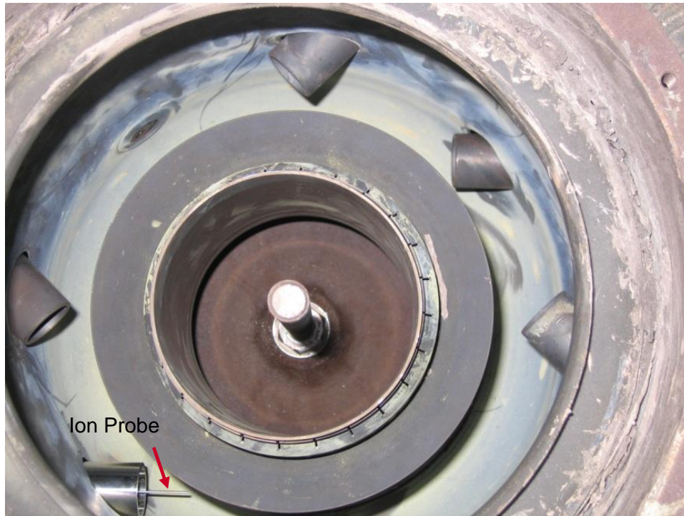
Figure 12 - Ion Probe positioned inside atmospheric combustor.
