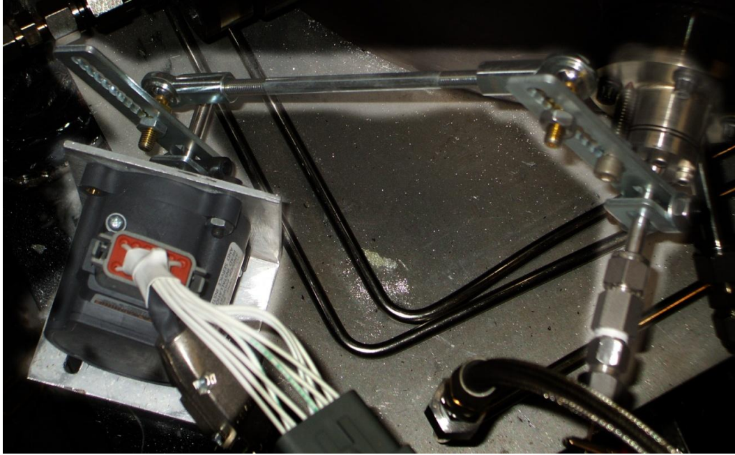
Figure 8 - Actuator linkage installed on atmospheric combustor.
