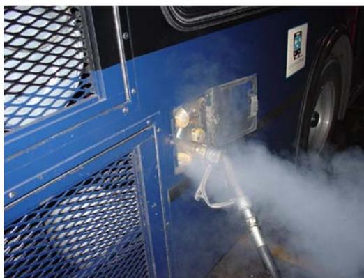
**Figure 2: LP Gas Emissions from Bus Tank Outage Gauge**
