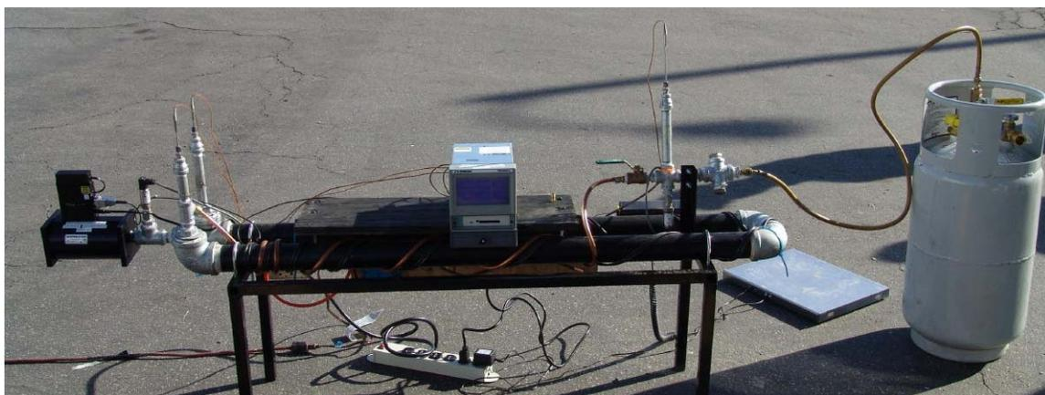
**Figure 23: Emissions Test Equipment Setup**
