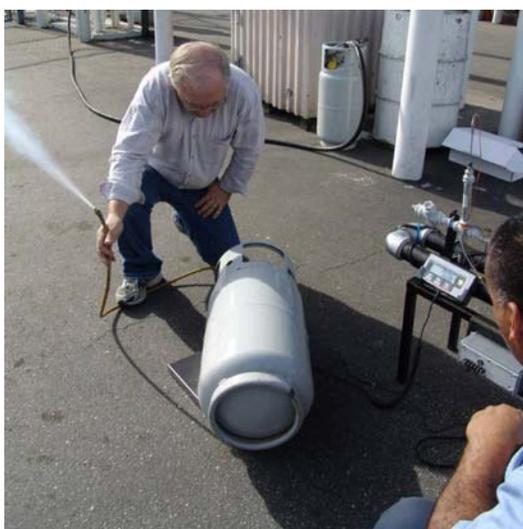
**Figure 26: Liquid phase emissions measurement using scale**
