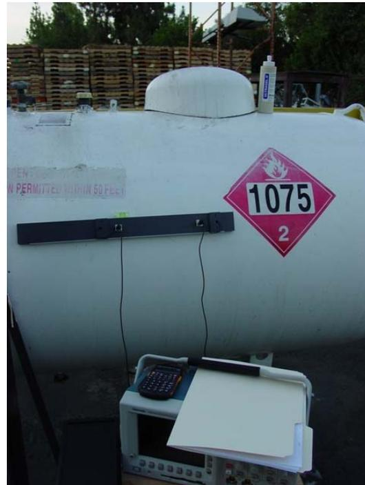
Figure 12: Field Tests of Beta-Prototype Maximus™ SFI Incorporating New Sensing Methods
