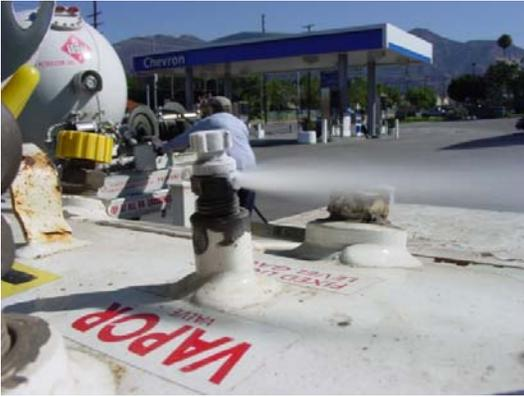
**Figure 13: Field Test of Pre-Manufacture Maximus™ SFI Showing Outage Gauge Emissions**
