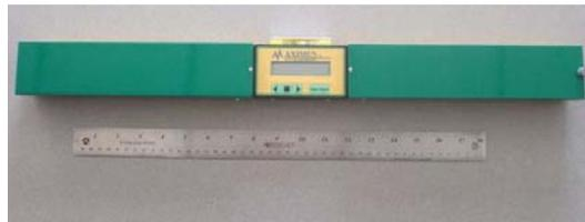
**Figure 16: Front View of Revised Pre-Manufacture Maximus™ SFI Prototype Showing New User Interface**
