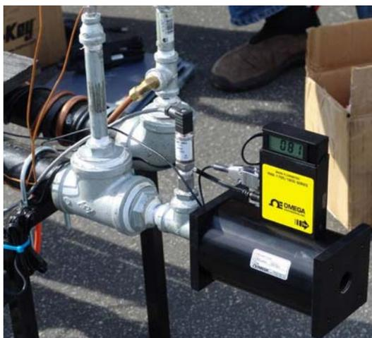
Figure 24: Flow, temperature, & pressure sensors mounted at expansion pipe outlet
