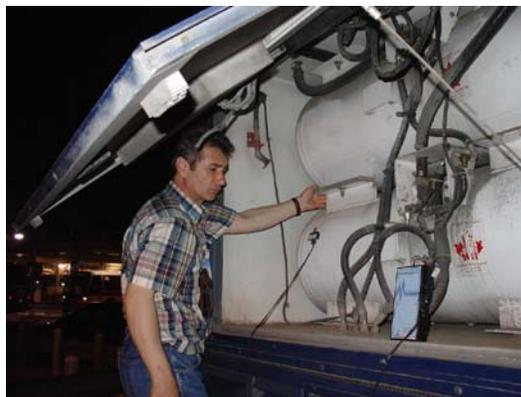
**Figure 4: Testing of Maximus™ Acoustic Sensing on Bus Tanks**
