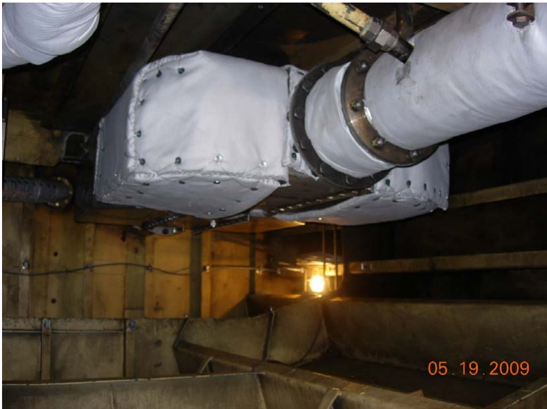
Figure 12: SCR and DPF assemblies for the Starboard main engine, in situ , viewed from the aft (downstream) end with lagging partially removed
