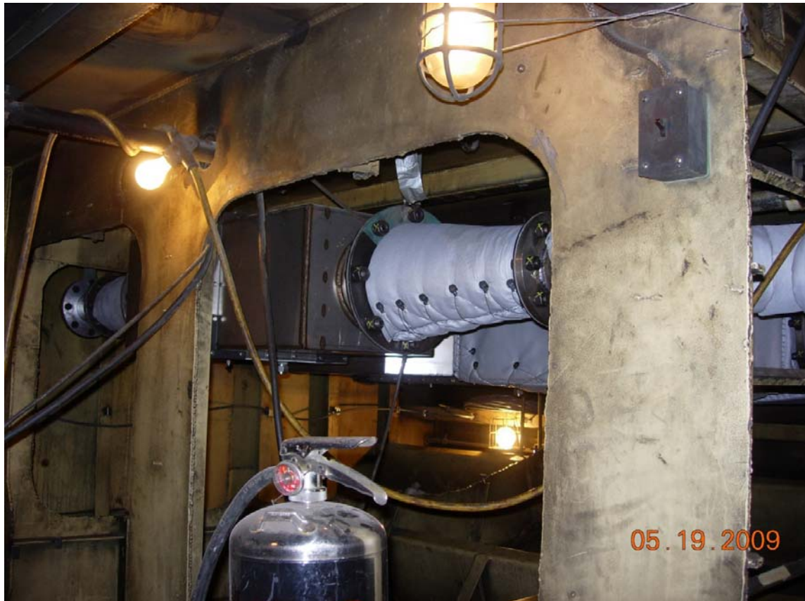
Figure 13: Combined DPF and SCR catalyst assembly for the Starboard generator, in situ with lagging partially removed
