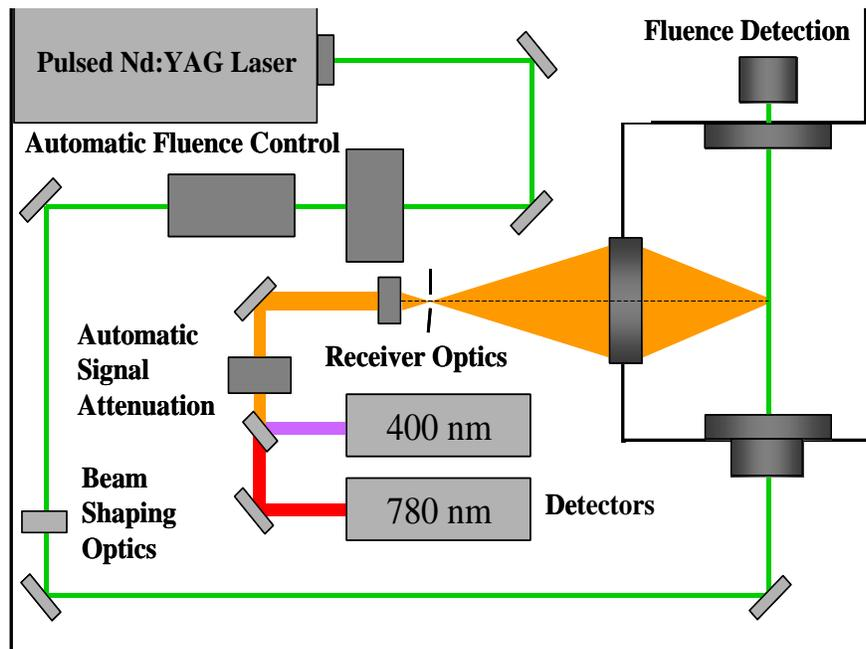
**Figure 2:** Optical schematic of the LII 200.
