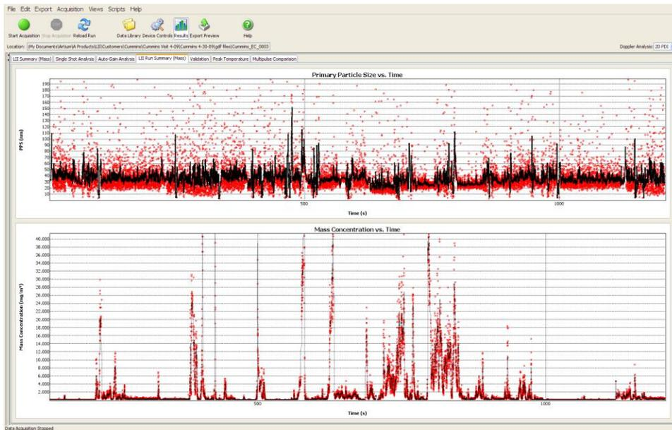
**Figure 31:** A closer observation of a section of the FTP cycle shows that the LII measurements consistently rise and fall shot to shot indicating that there were no individual spikes in the data. This implies that there are no large particles in the sample and so the results should agree with gravimetric.
