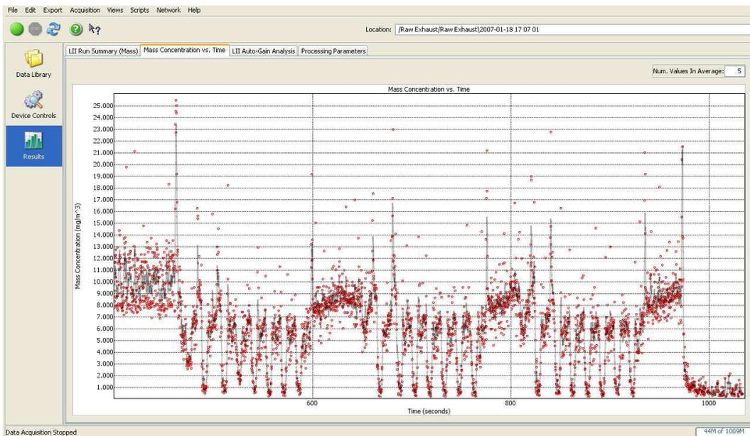
**Figure 16:** Preliminary data obtained with the LII 200 HS by sampling raw exhaust in a Cummins test cell.
