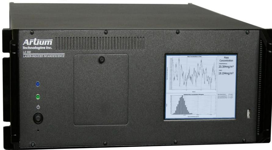
**Figure 4:** Photograph of the Artium LII 300. The footprint is significantly reduced compared to the LII 200.
