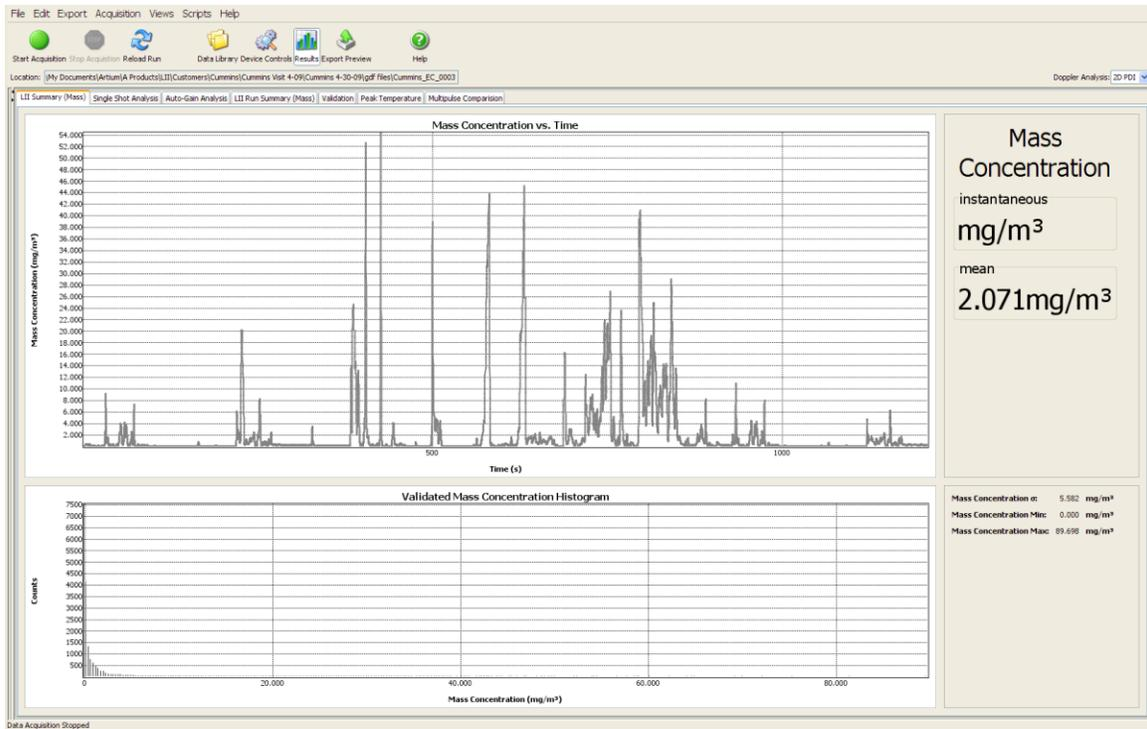
**Figure 30:** In this test, the sampling was essentially ideal in the sense that there were no large spikes indicating the presence of large particles. The CVS and sampling system appeared to be clean and the LII signals were very consistent with very low variations shot to shot except for changes in engine cycles.
