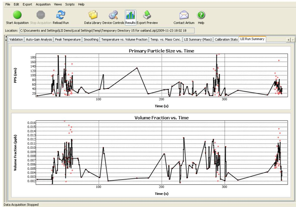
**Figure 39:** Plot showing variation of primary particle size and soot volume fraction with time.
