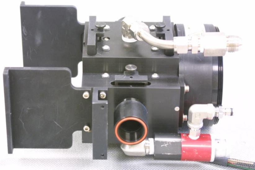
**Figure 8:** Photograph of the sample cell that incorporates the retro-reflecting spherical mirror for increased signal strength.
