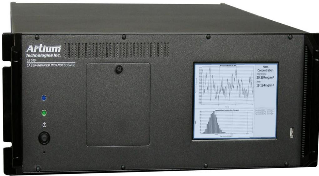
**Figure 15:** The LII 300 system with integrated pneumatics, optics, sample cell, control computer and touch-screen monitor.
