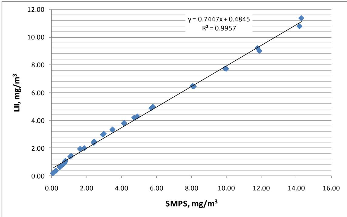
**Figure 27:** NASA Glenn measurements of soot generated by the mini-CAST burner and compared to the TSI SMPS measurements.
