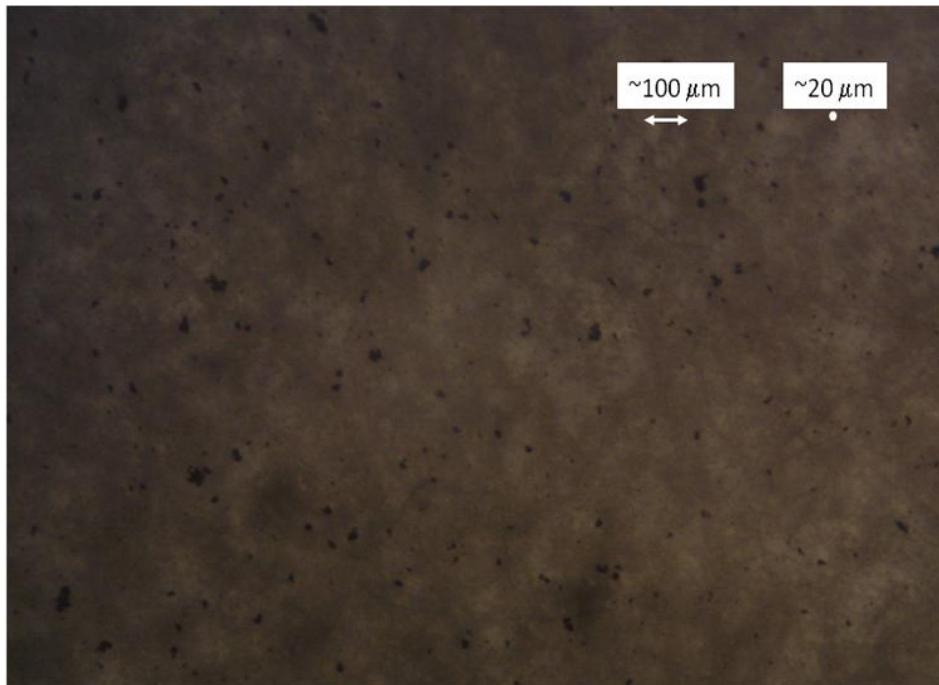
**Figure 29:** Optical microscope images of soot filters obtained April 28, 2009. Filter data was obtained downstream of a cyclone separator supposedly able to cut off particles larger than 2.5  $\mu\text{m}$ . Note that there are particles as large as 50  $\mu\text{m}$  in these images. The filters were contained in the Petri dishes and were not contaminated during the observation process.
