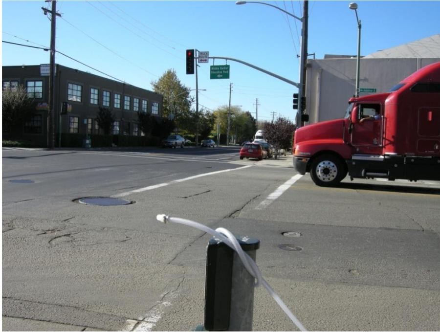
**Figure 36:** Sampling line to sniff the air for soot particles when trucks pass by.
