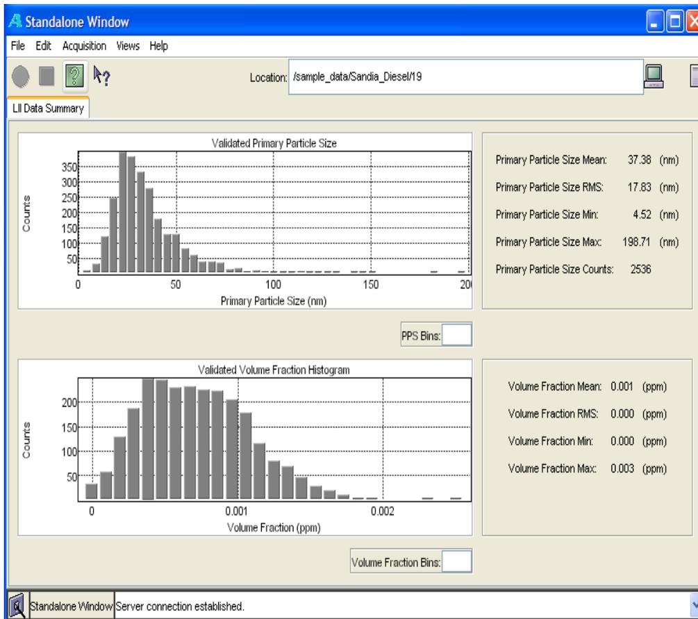
**Figure 3:** Typical primary particle size and soot concentration histograms displayed by the Artium LII 200 software.
