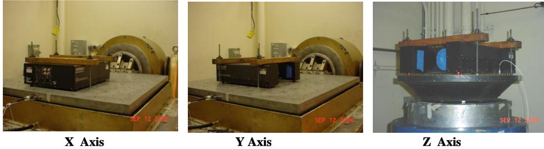
**Figure 9:** Setup used for the shock studies.
