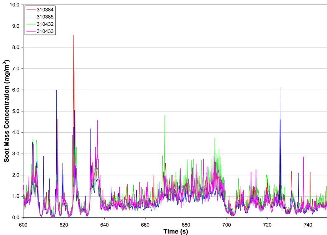
**Figure 18:** Dilution Tunnel (time segment from 600-750s – four repeats).
