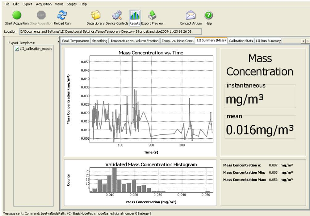
**Figure 38:** Plot showing measurement of soot mass concentration in air.
