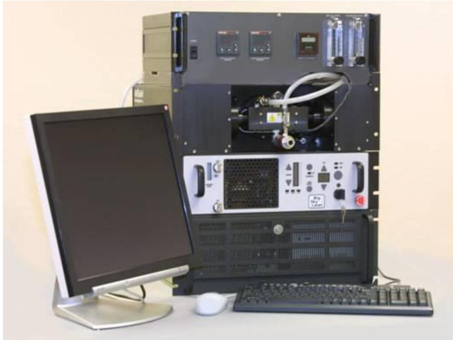
**Figure 1:** Photograph of the Artium LII 200 system including computer, laser controller, and dilution flow controller. This is how the instrument looked before the ICAT project started.
