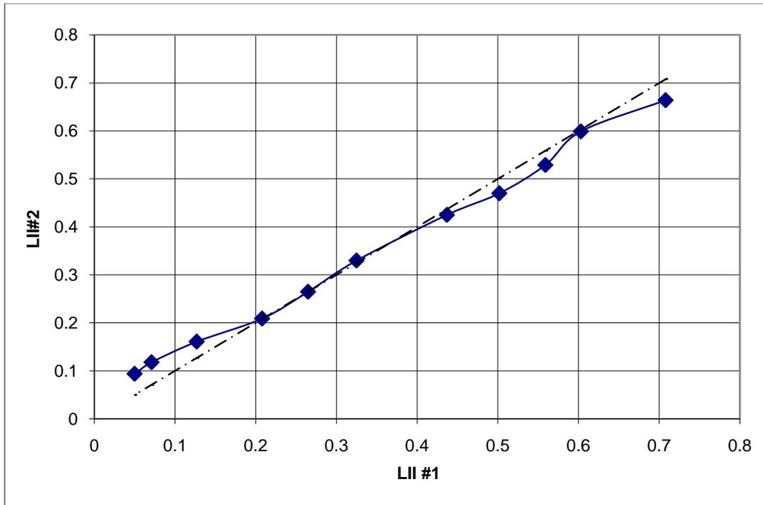
**Figure 7:** Comparative data expanded around the low end of the soot volume fraction end of the distribution.
