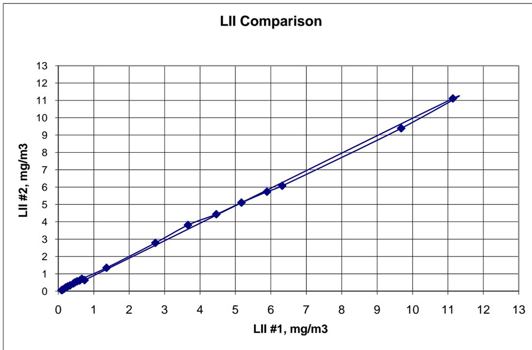
**Figure 6:** Comparison of the data obtained between the two identical LII instruments measuring a wide range of soot concentration.
