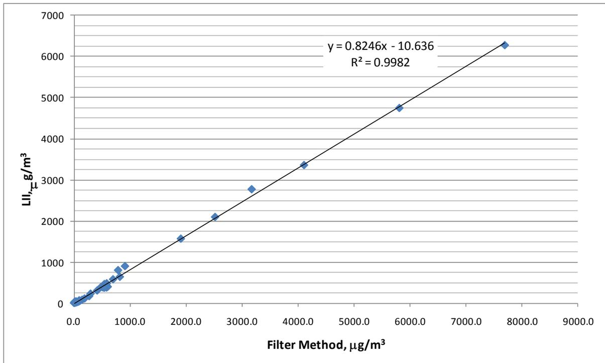
**Figure 26:** NASA Glenn Research Center tests conducted on soot from a mini-CAST burner in December 2009 prior to measuring gas turbine particulate emissions.
