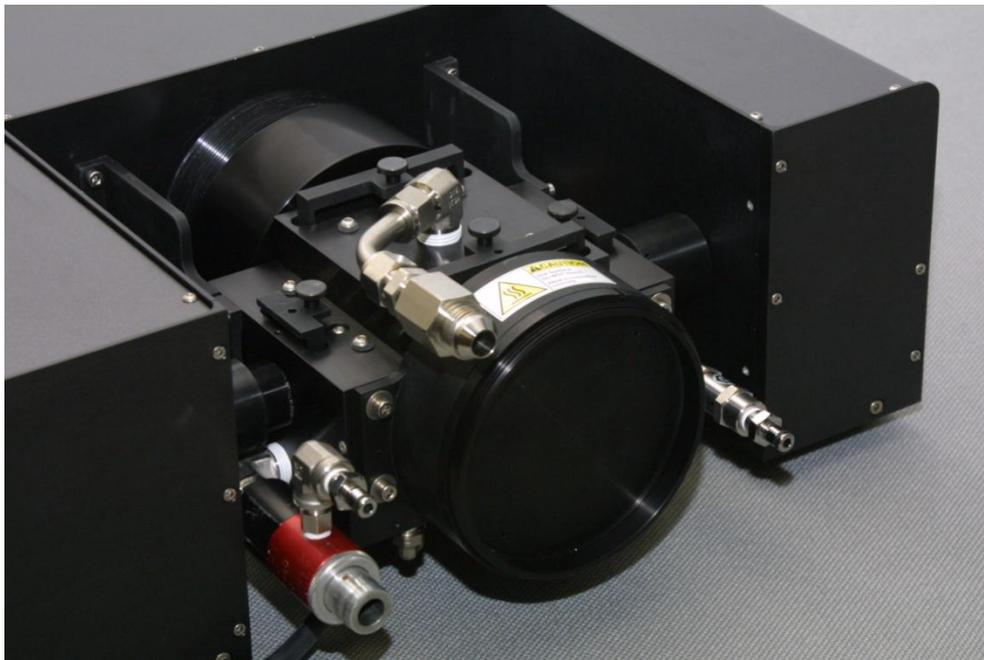
**Figure 12:** Close up shot of the sampling cell used in the LII 200.
