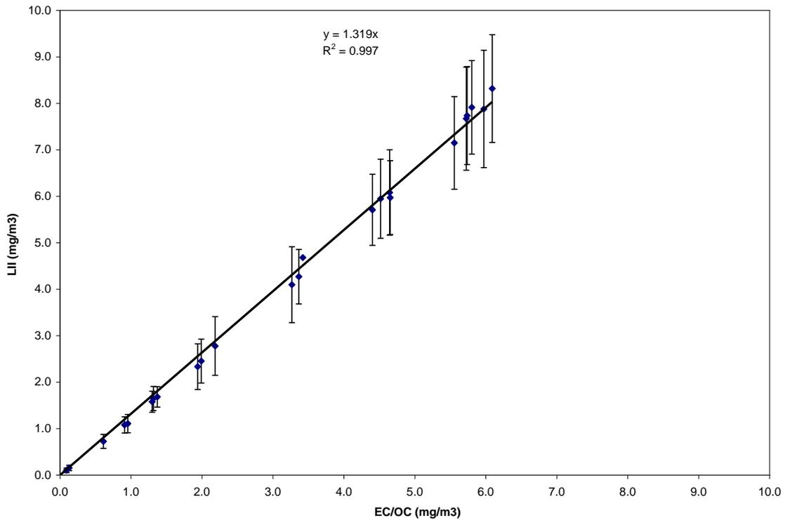
**Figure 25:** Comparison of LII and EC/OC soot concentration measurements.
