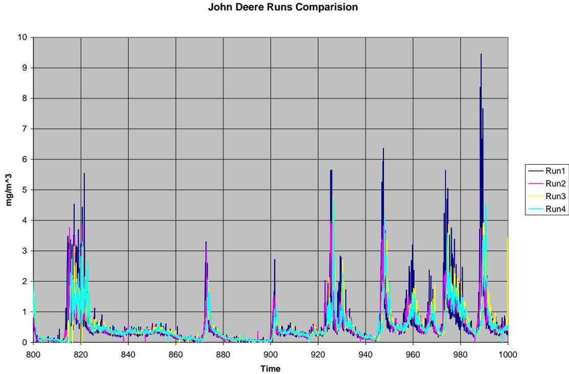
**Figure 24:** Raw exhaust data comparison.
