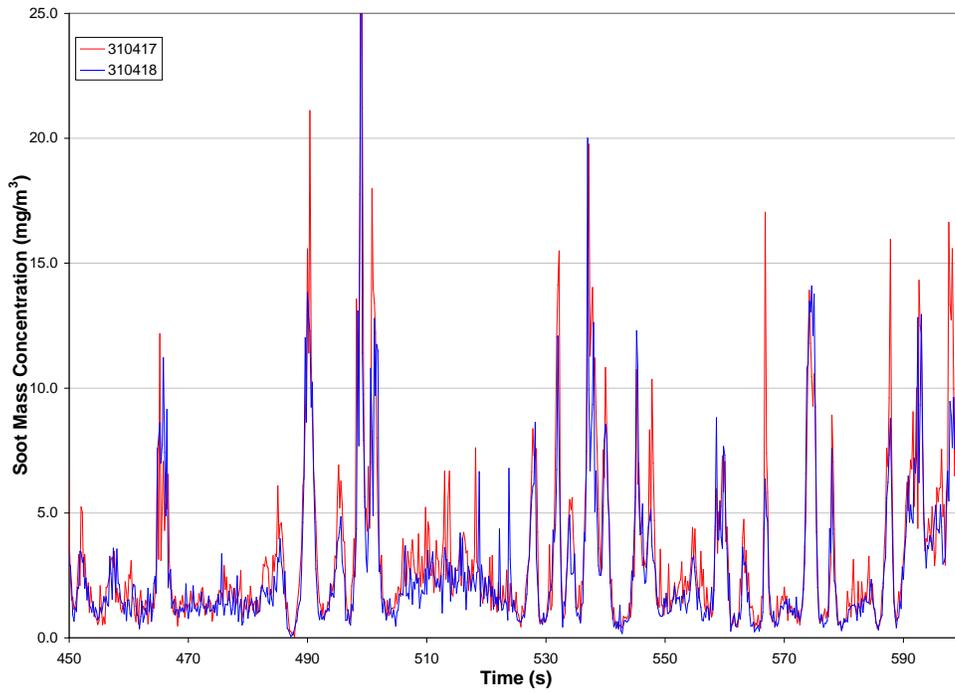
**Figure 20:** Raw Exhaust (time segment from 450-600s – two repeats).
