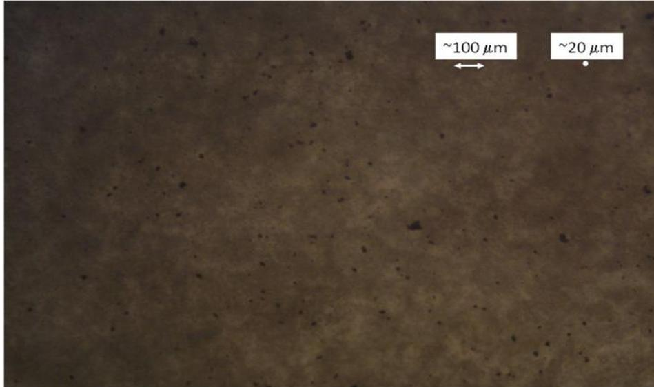
**Figure 28:** Optical microscope images of soot filters obtained April 28, 2009. Filter data was obtained downstream of a cyclone separator supposedly able to cut off particles larger than 2.5  $\mu\text{m}$ . The scale shown in the image is approximate and is provided for a rough reference for particle size estimation.
