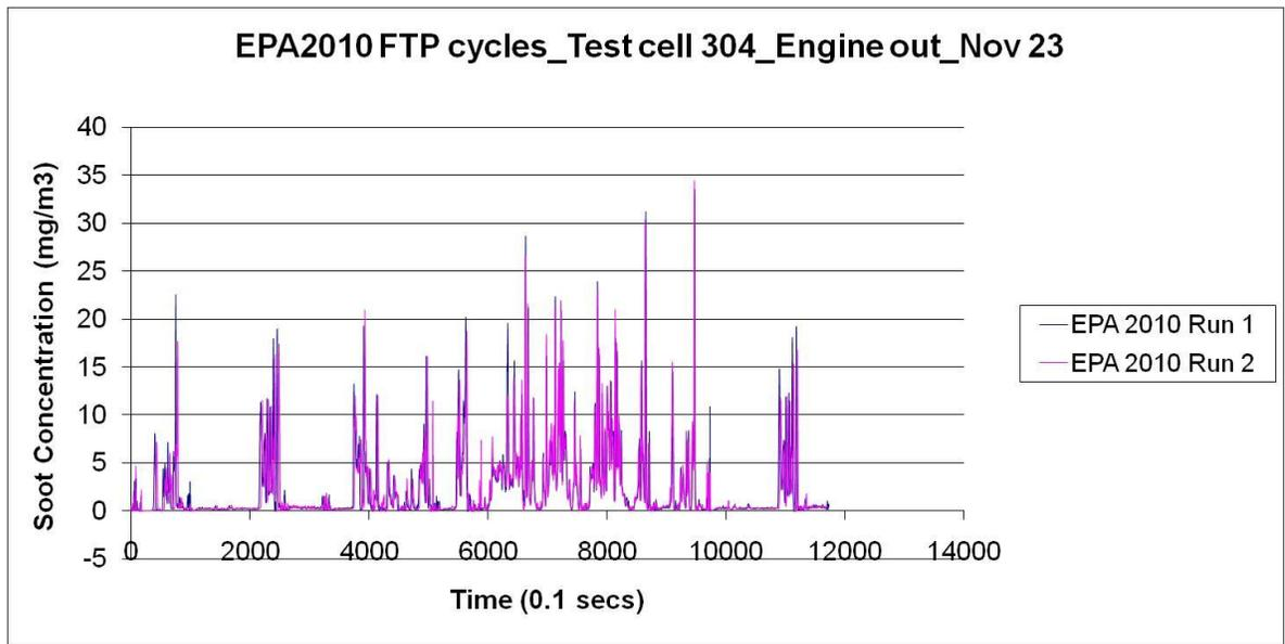
**Figure 33:** Repeatability of LII 300 runs at Cummins.
