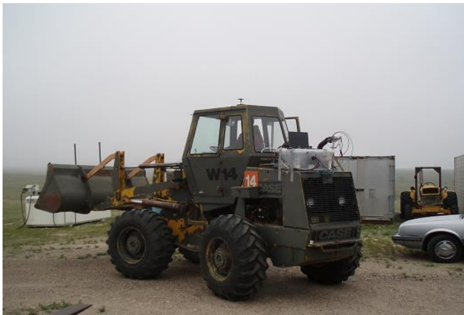
Figure 2.1 shows the ETaPS mounted on a diesel Caterpillar front loader. As in all installations power was provided from an on-board 110V generator grounded to the vehicle
