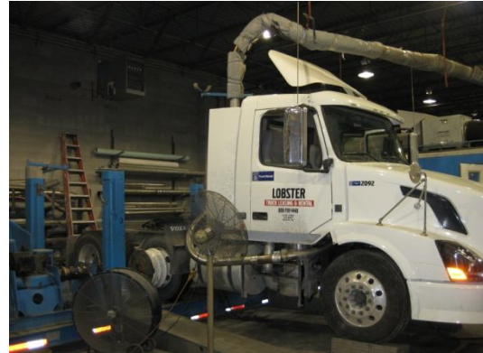
2008 Volvo day cab on dynamometer with insulated pipe.
