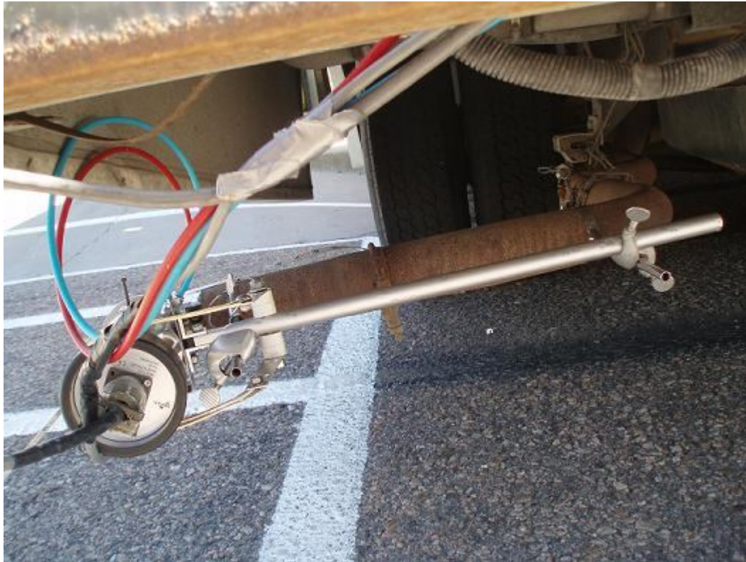
Figure 2.3 ETaPS mounted so as to observe the particles exiting the exhaust of a gasoline powered 1996 Winnebago Itasca motor home powered by a GM 454 cu.in. V8 engine.
