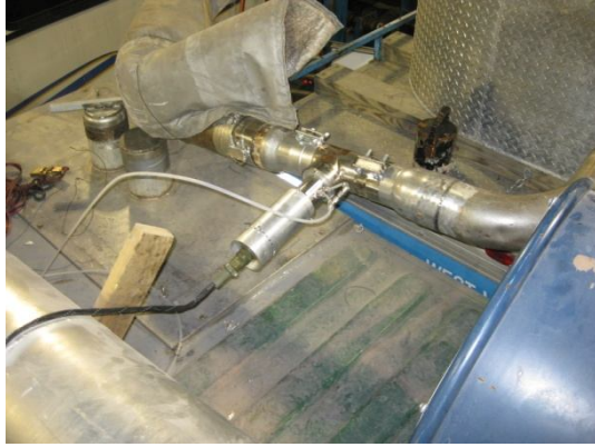
ETaPS in hot, raw exhaust before CVS dilution tunnel.
