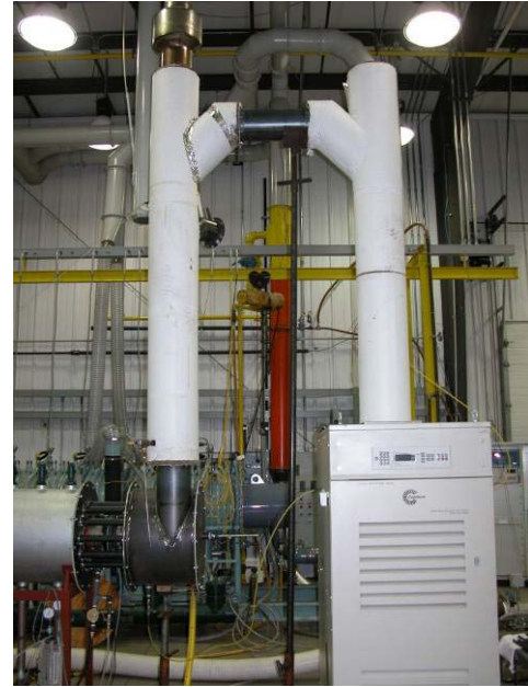
Figure 2. Layout of Microturbine Supplemental ULN Burner
