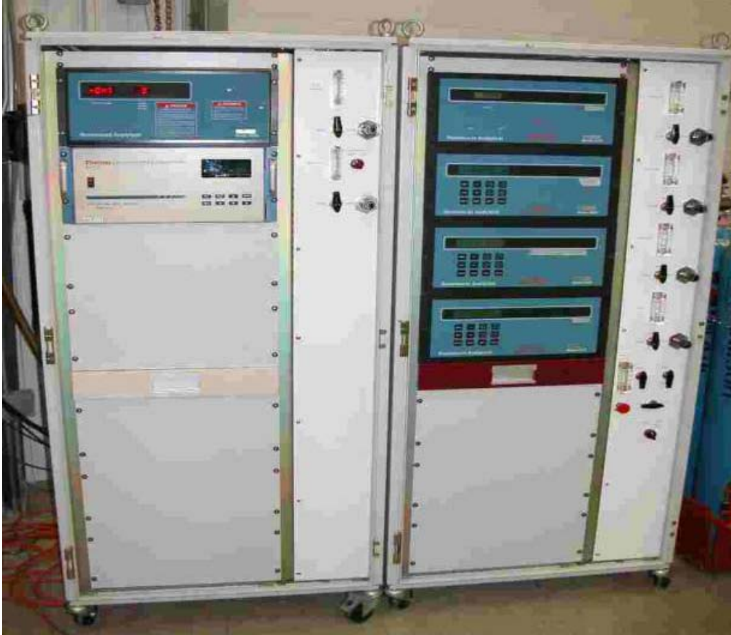
Figure 6. Panel Mounted Emissions Monitors
