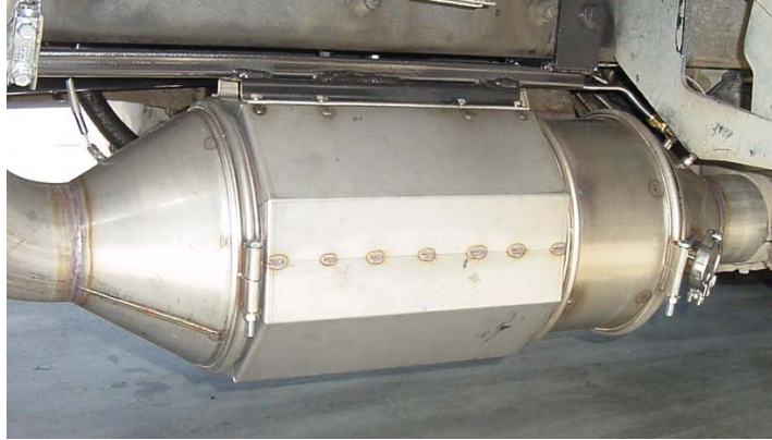
Figure 6. Horizon EPF installed on test vehicle.
