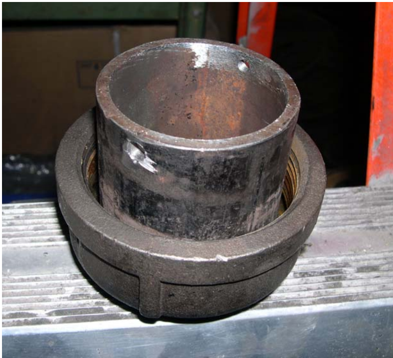
Figure 20 Modified Pipe Cap for Holding Filter and Providing Sensor Access
