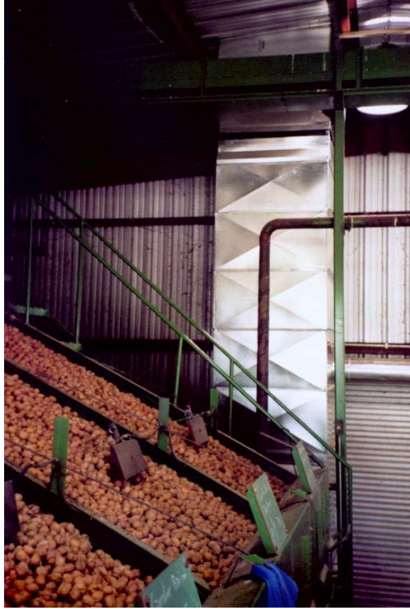
Figure 8: Duct from solar panels on roof connect to walnut dryer
