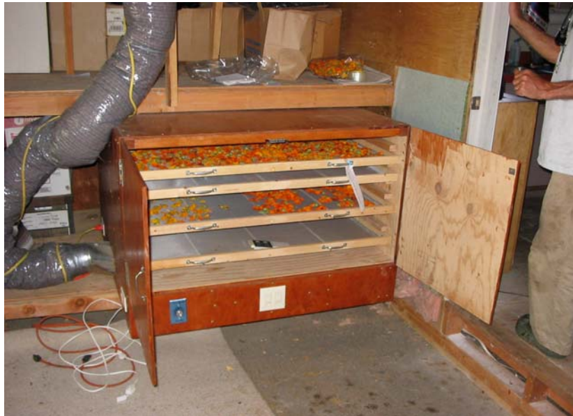
Figure 16: Batch herb dryer with sliding trays (doors closed when drying)
