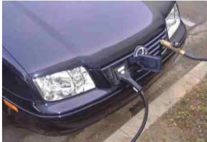
Figure 12. Hookups for AC Power and Natural Gas Fuel
