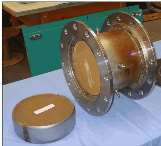
**Figure 45. Catalyst Honeycomb Substrate and Catalyst Installed in System**
