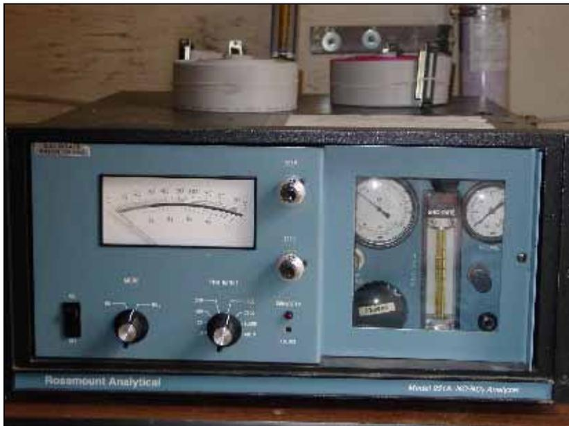
**Figure 42. NO/NOx Analyzer Instrumentation.**
