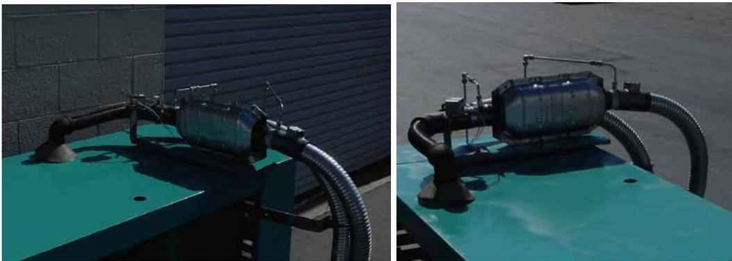
**Figure 27. 20 kW Natural Gas Generator With Test Converter.**
