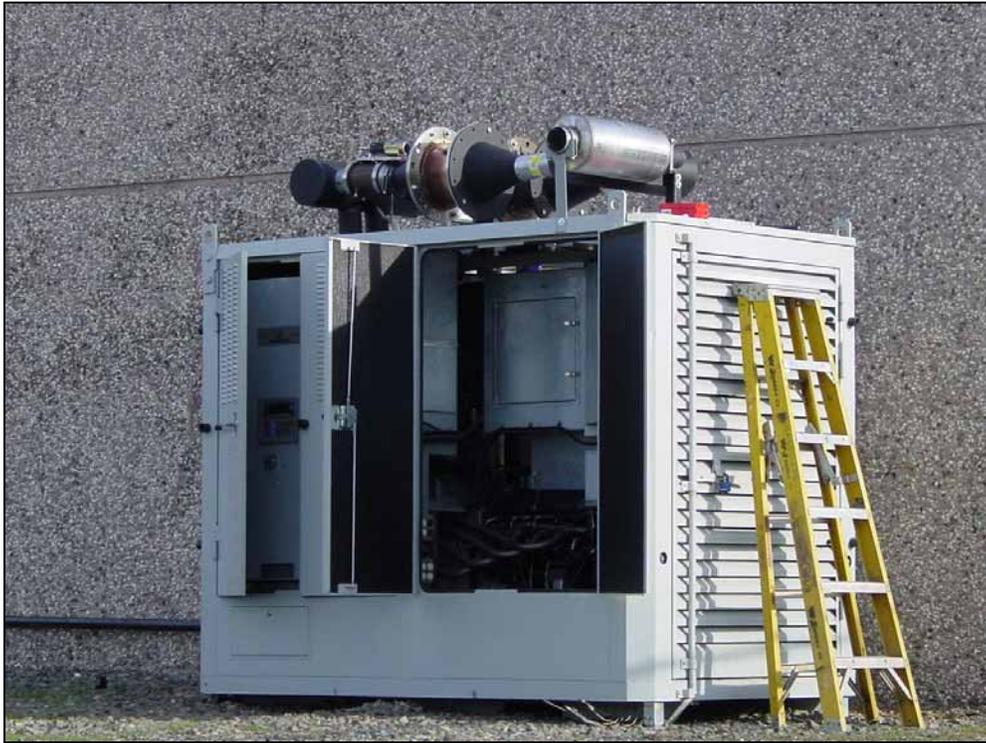
**Figure 29. 100 kW Natural Gas Generator Set and MicroNOx Exhaust System For Field Testing**
