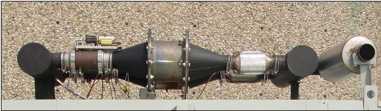
**Figure 44. MicroNOx Exhaust System Field Installation.**
