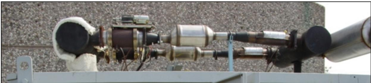
**Figure 56. MicroNOx Exhaust System with Secondary Treatment System.**
