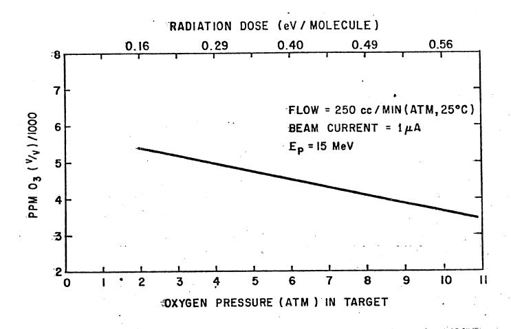
Figure 6. Relationship of ozone concentration to oxygen pressure in the target system.
