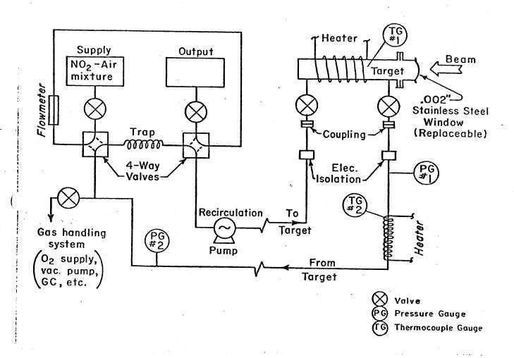
Figure 8. Schematic diagram of the experimental system used to synthesize and collect radioactive nitrogen dioxide  $(^{13}\text{NO}_2)$ .
