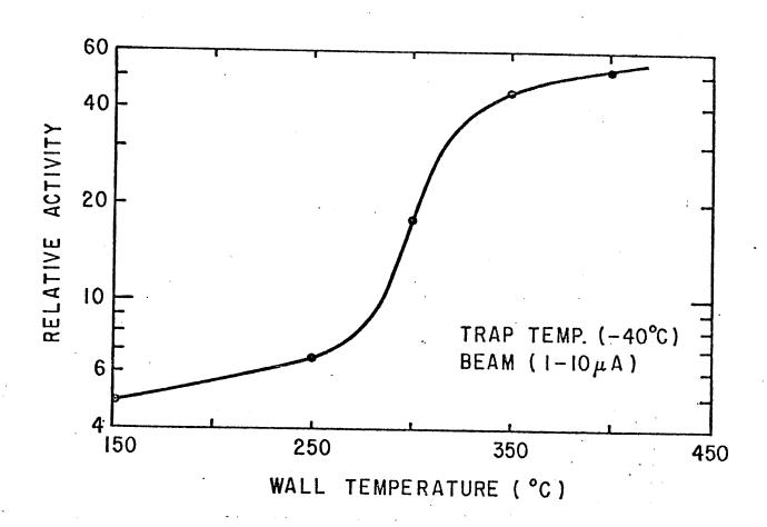
Figure 7. Increases in reactive  $^{13}{\rm N}$  radioactivity as a function of temperature of the target wall.
