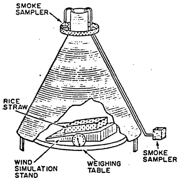
Fig. II-5. Deployment of smoke samplers about the U.C., Riverside, burning tower.
