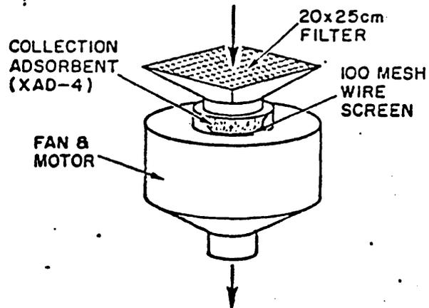
Fig. II-1. Hivol sampler with filter and XAD-4 resin.
