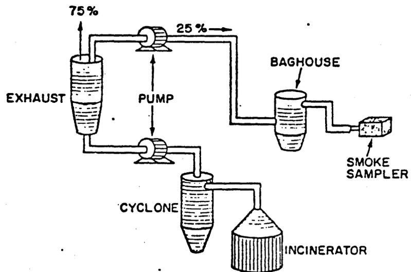
Fig. II-7. Sampling of smoke from the commercial incineration of rice straw.
