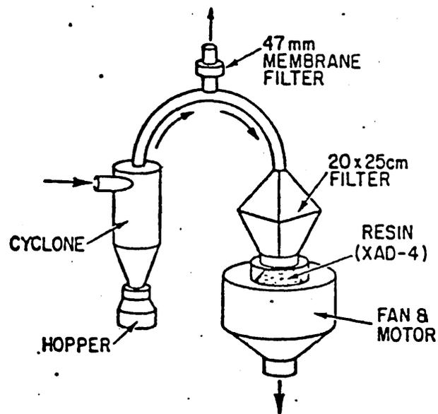
Fig. II-2. Hivol sampler configuration for respirable fraction of rice straw smoke.
