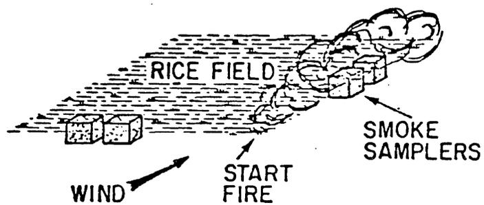
Fig. II-4. A typical deployment of Hivol samplers about a burning rice field.
