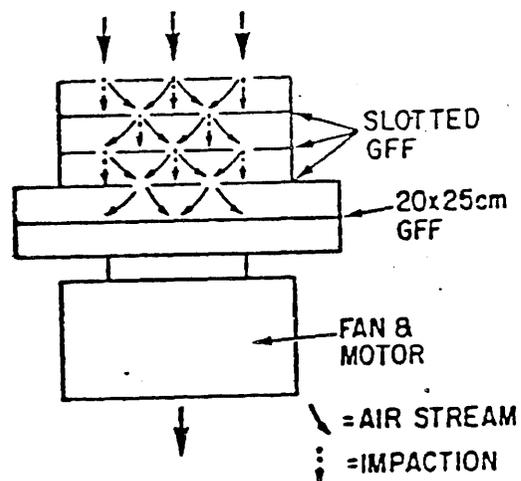
Fig. II-3. Hivol cascade impactor for size fractionation of rice smoke particles.
