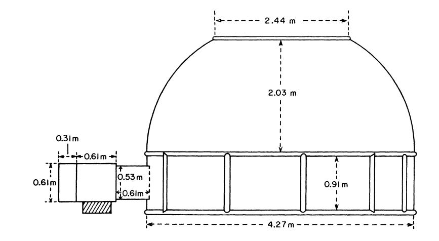
Figure 1. Diagram of orange tree exposure chamber.
