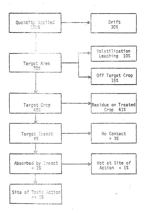
Figure 8-1. Percentage Distribution of Typical Losses of Pesticides between Spray Nozzle and Site of Toxic Action. 90
