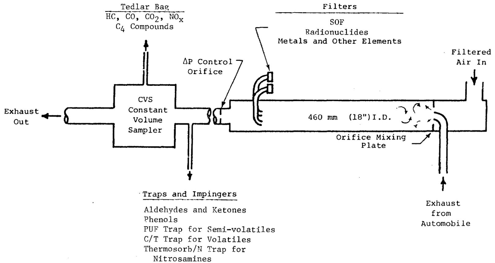
**FIGURE 3. EMISSIONS SAMPLING SYSTEM**
