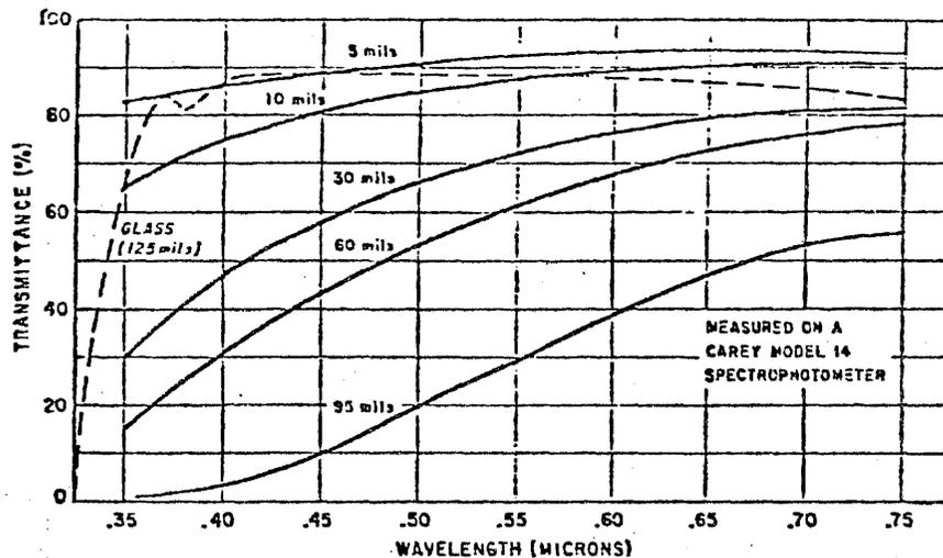
Figure 4. LIGHT TRANSMISSION VS. THICKNESS—"TEFLON" FEP FILM
