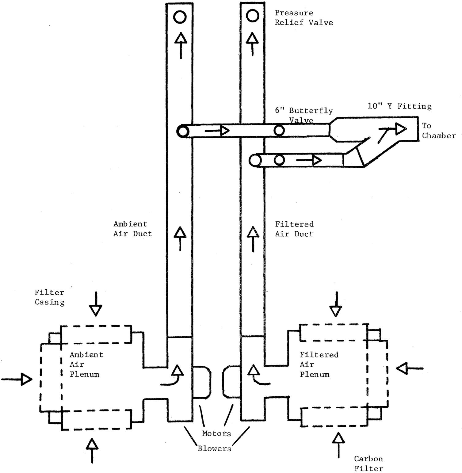
Figure 3. Diagram of chamber showing structural components. Chamber dimensions are 7' x 7'.
