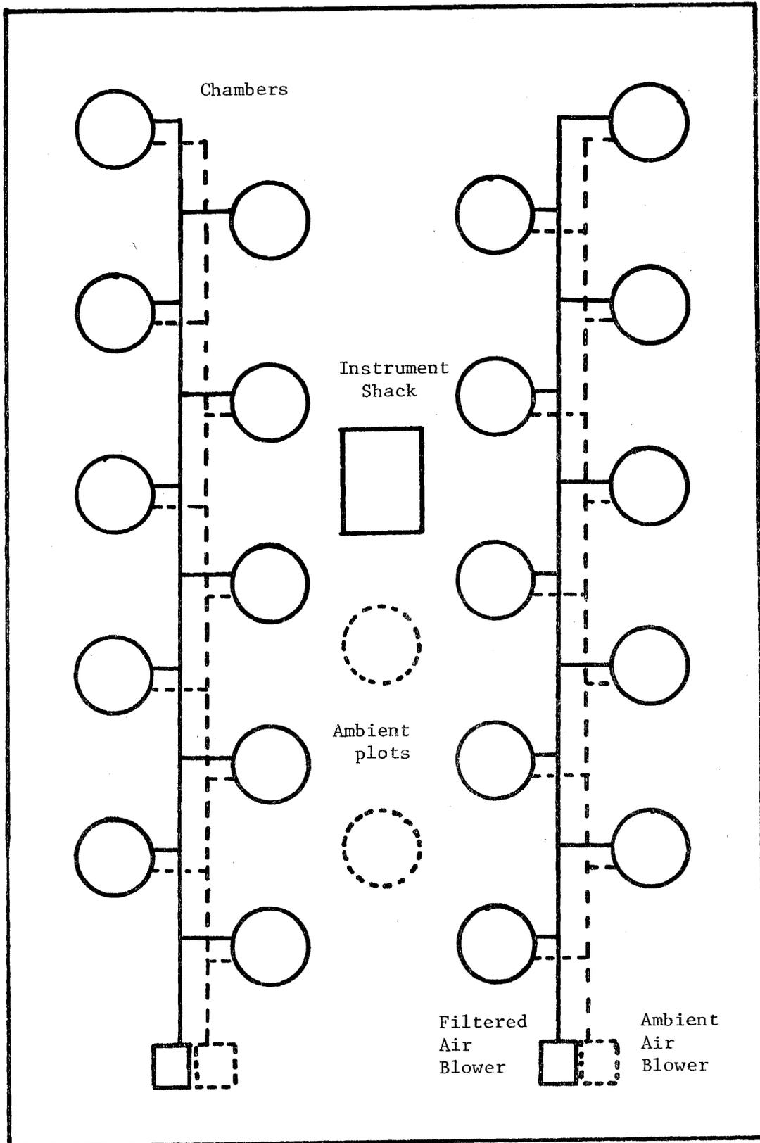
Figure 2. Detail of air handling system for fumigation chambers.
