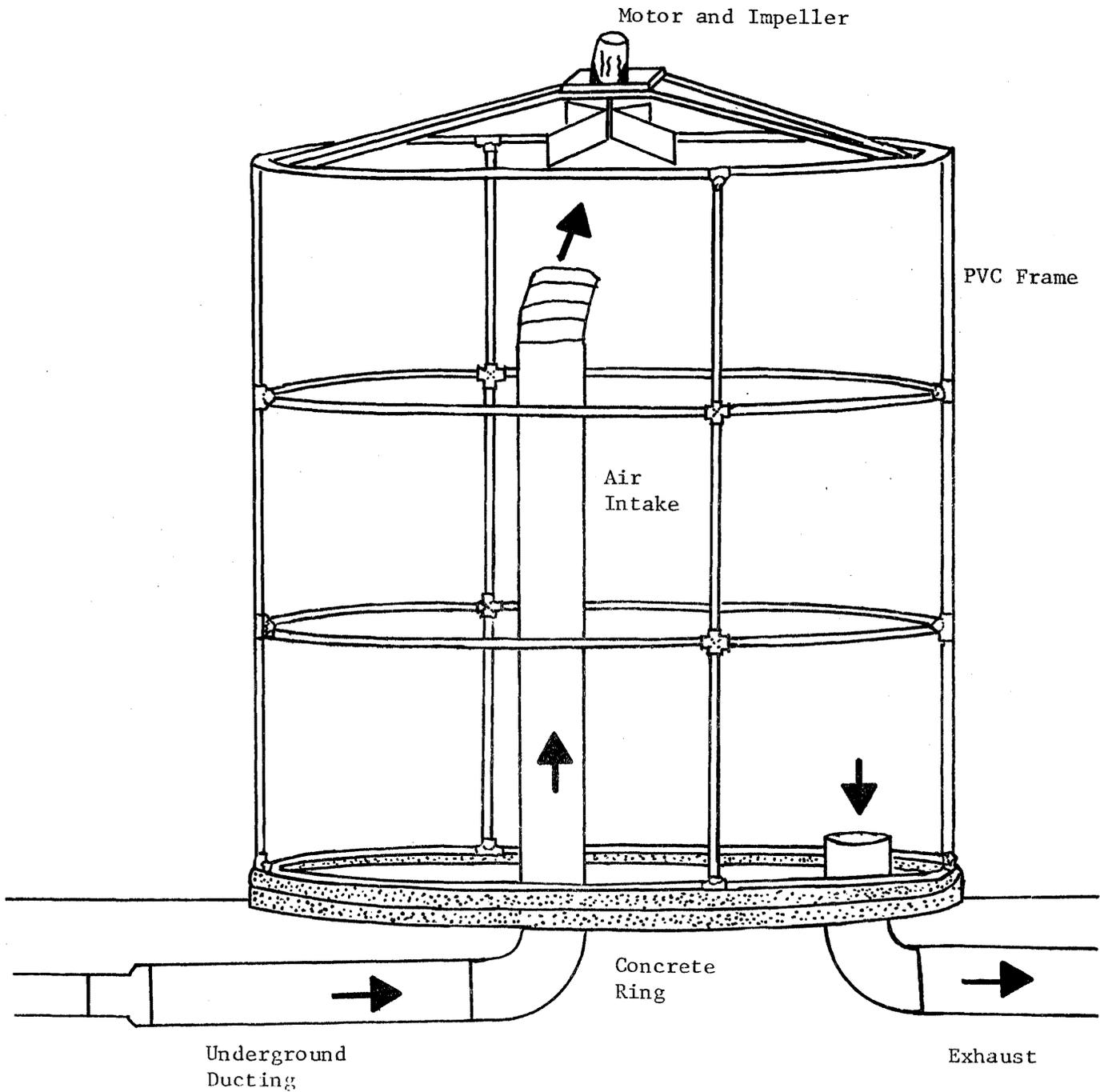
frame and anchors the uppermost portion of the Teflon envelope. An extension shaft from the motor protrudes through the Teflon envelope and supports a 6-blade impeller which rotates at 60 rpm. The mixture of filtered and nonfiltered air enters the chamber via a 10" PVS underground duct which then extends 5 ft vertically and directs the air stream directly at the impeller. Chamber exhaust is vented through a 10" PVS "U" tube directly into the atmosphere.
