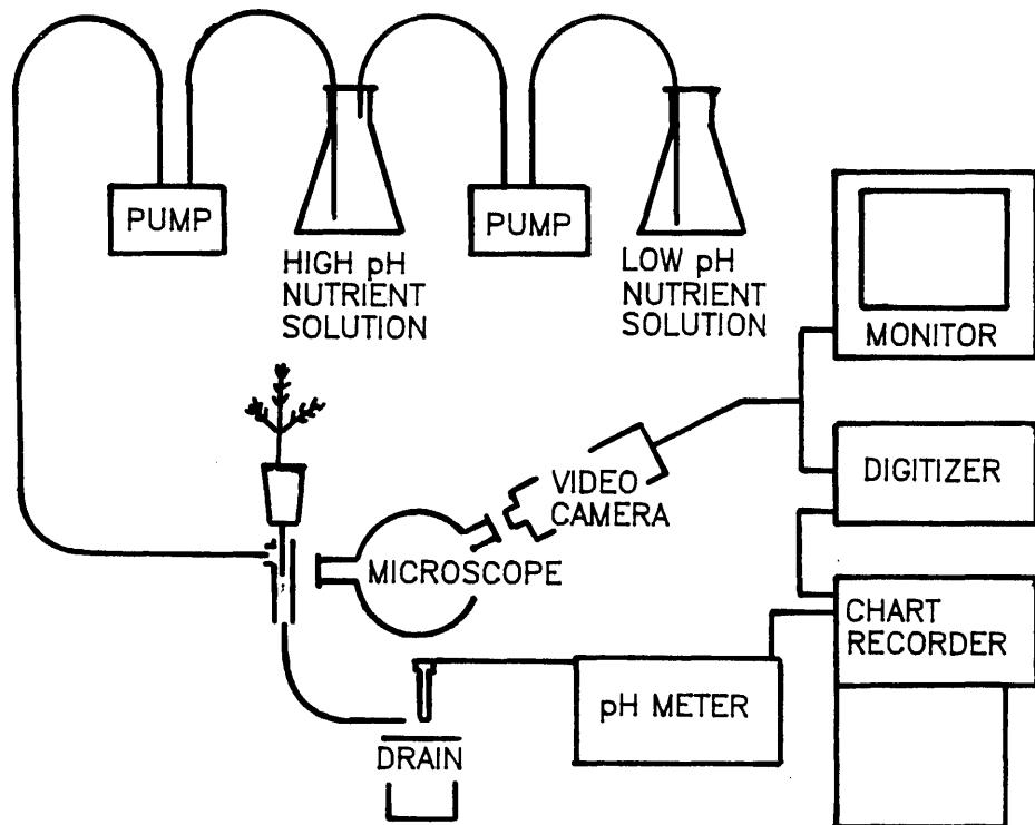
Figure 3. Diagram of rhizotron used for monitoring and recording root elongation.
