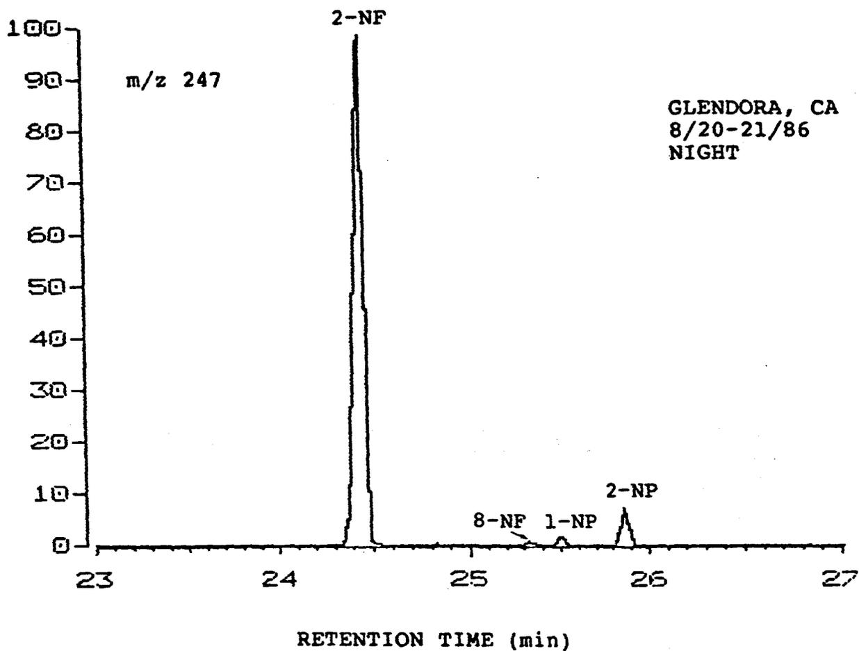
Figure VI-14. GC/MS-MID trace showing the molecular ion of the nitrofluoranthenes (NF) and nitropyrenes (NP) analyzed in an ambient POM sample collected at Citrus College, Glendora, August 20-21, 1986, from 2000-0800 PDT.
