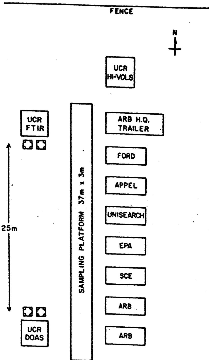
Figure III-2. Positions of the longpath FT-IR and DOAS systems and UCR Hi-vols relative to the instruments of the other participants in the Carbonaceous Aerosol Study on the Citrus College campus, August 1986.
