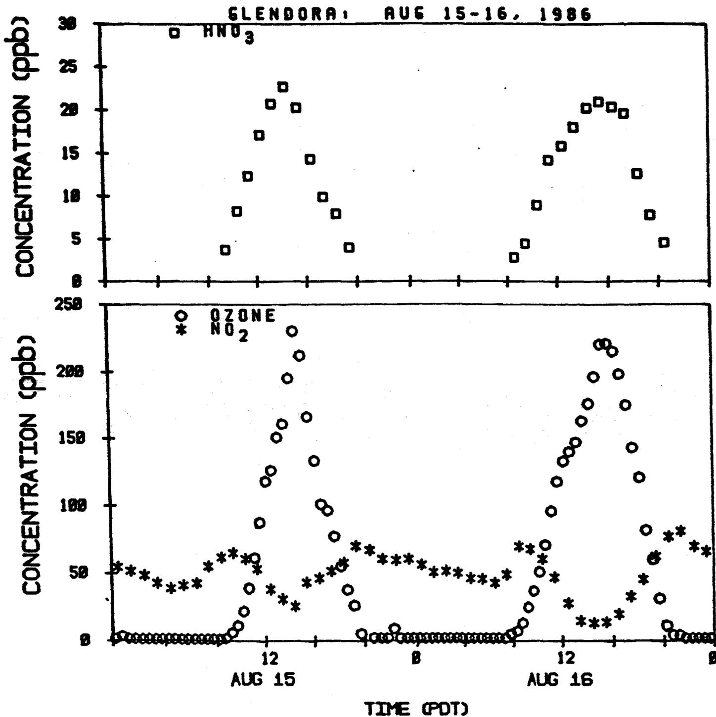
Figure V-7. Time-concentration plots of average  $\text{HNO}_3$  (FT-IR),  $\text{NO}_2$  (DOAS), and  $\text{O}_3$  (Dasibi monitor) at Citrus College for August 15-16, 1986.
