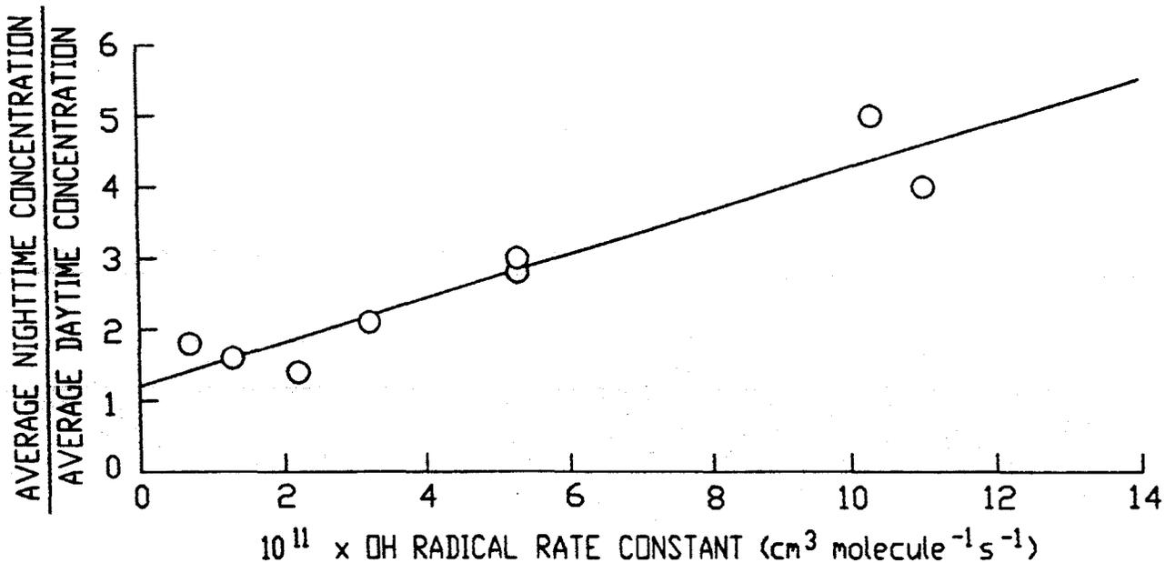
Figure VIII-1. Plot of the average nighttime/average daytime concentration ratio for the volatile PAH against the OH radical reaction rate constant.
