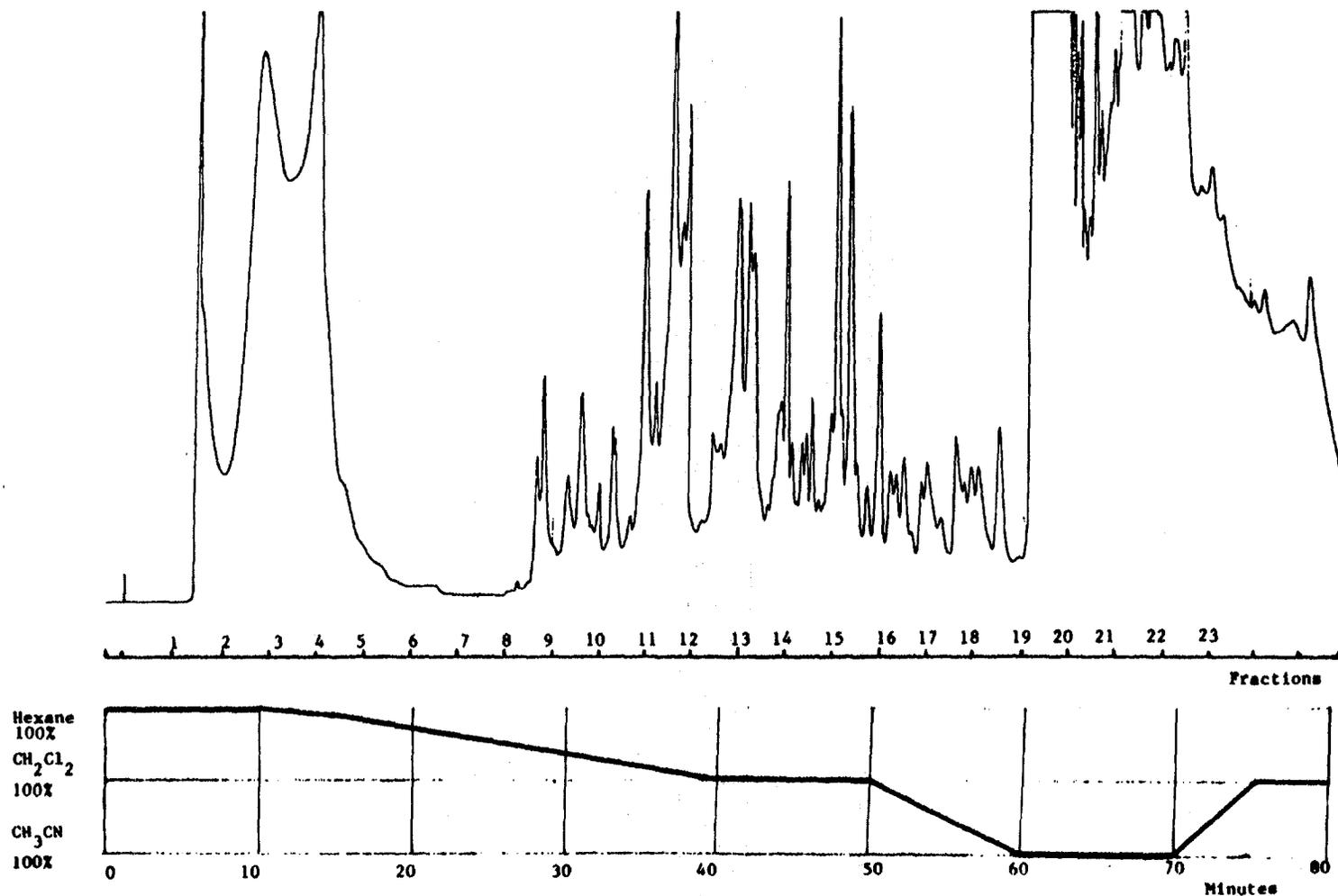
Figure VI-2. HPLC trace (254 nm) and gradient solvent program for separation of an ambient sample collected on PUF plug. Semi-preparative Ultrasphere Si column (1 cm x 25 cm), 3 mL min<sup>-1</sup>. HPLC fractions were combined as follows: #3-7, #8-11, #12, #13-15, #16-23.
