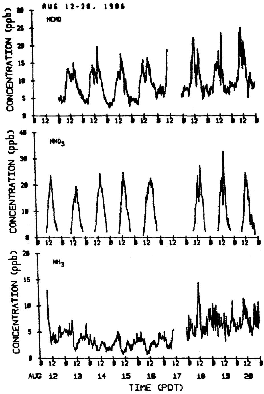
Figure V-6. Time-concentration profiles for formaldehyde, nitric acid and ammonia measured by long pathlength FT-IR spectroscopy during the 1986 Citrus College study.
