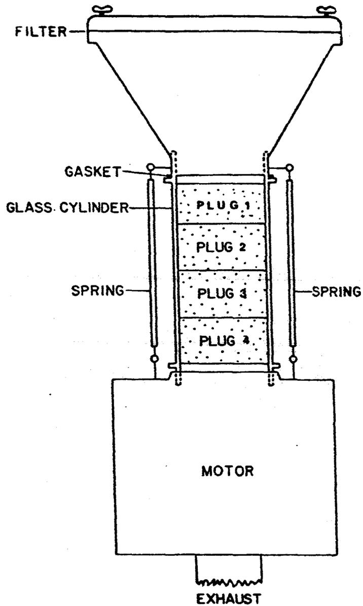
Figure VI-1. Schematic of modified Hi-vol sampler with PUF plugs underneath the filter to collect gas phase species and compounds "blown-off" the filter.
