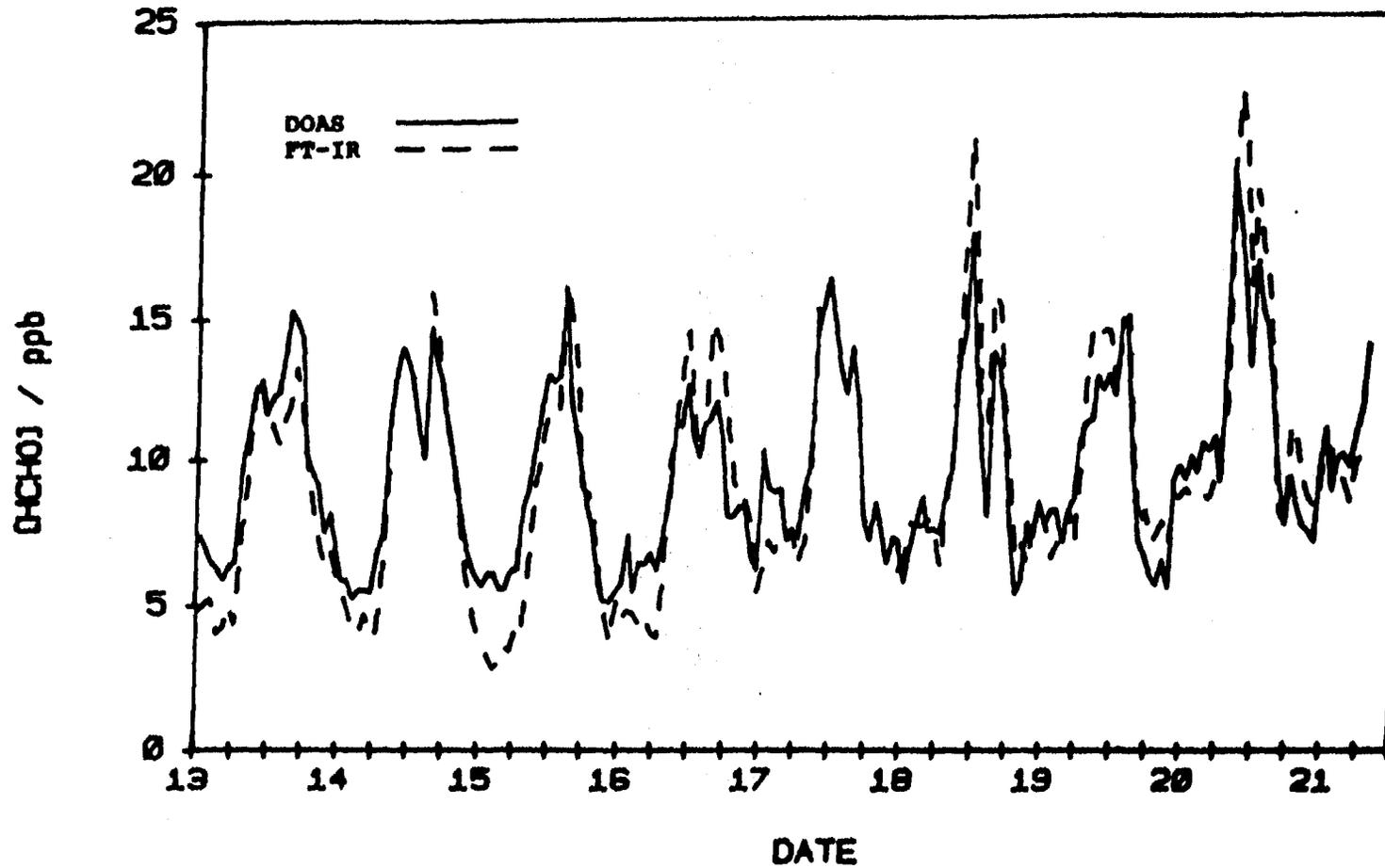
Figure IV-3. Time concentration profiles for formaldehyde measured by long pathlength DOAS and FT-IR spectrometers at Citrus College (Glendora) in August 1986.
