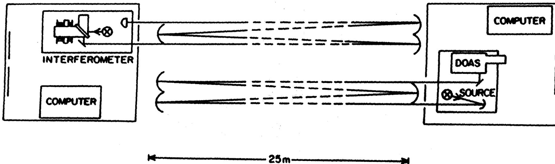
Figure V-1. Relative arrangement of the longpath FT-IR and DOAS systems.
