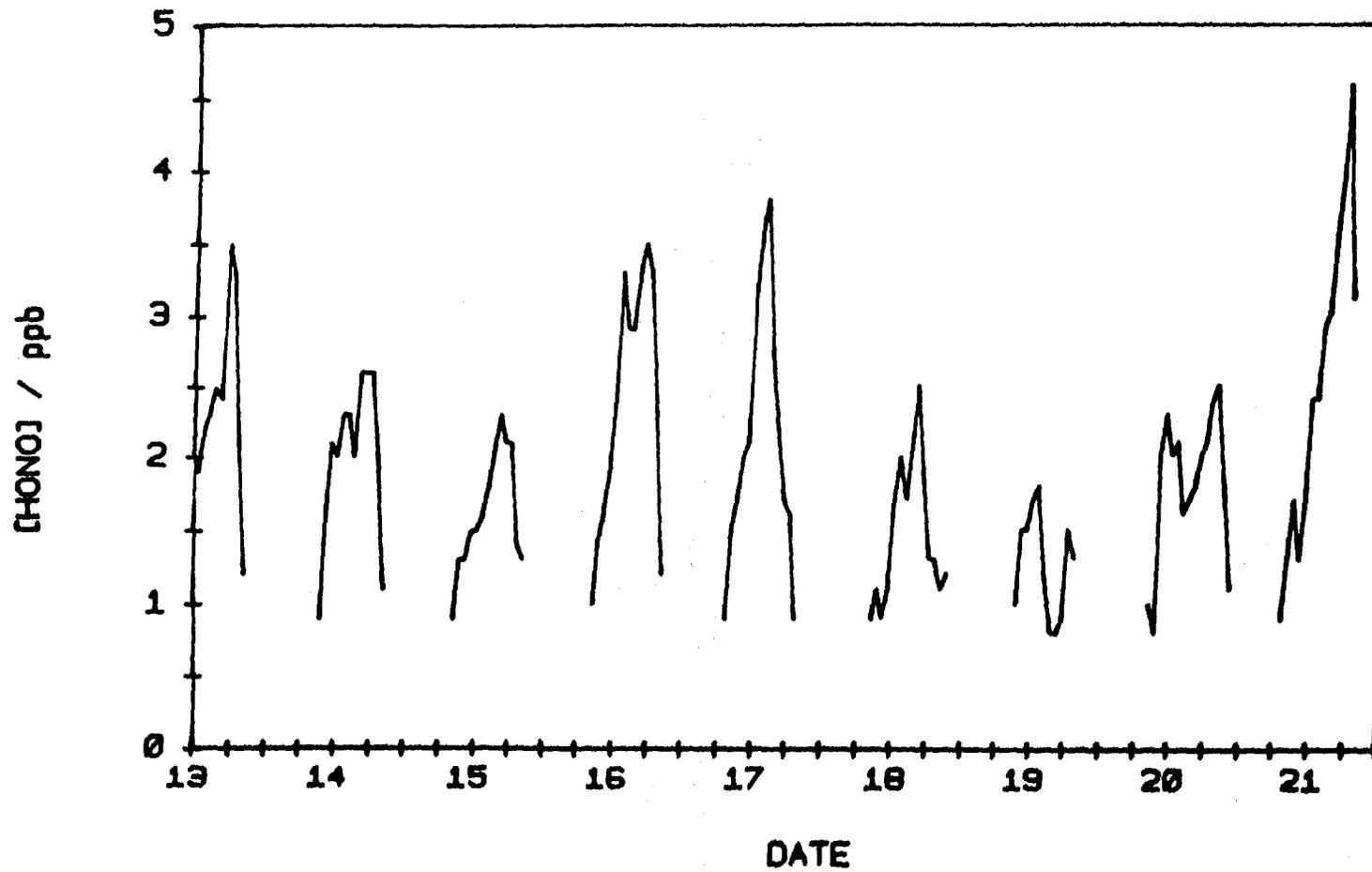
Figure I-2. Nitrous acid time-concentration profiles measured by long pathlength DOAS system at Citrus College (Glendora) in August 1986.
