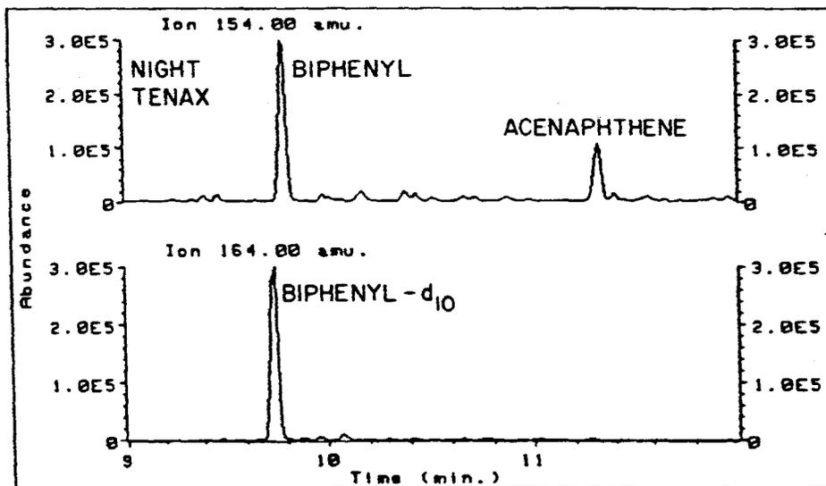
Figure VI-7. GC/MS-MID traces for the molecular ion of biphenyl and acenaphthene ( $m/z$  154) and the deuterated internal standard, biphenyl- $d_{10}$  ( $m/z$  164) from the analyses of a daytime (top) and nighttime (bottom) ambient air sample collected on Tenax-GC solid adsorbent at Citrus College, Glendora, CA.
