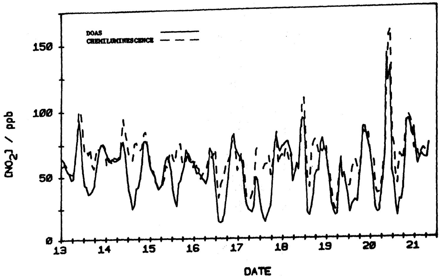
Figure IV-2. Time concentration profiles for nitrogen dioxide measured by DOAS and chemiluminescence (NO<sub>x</sub>-NO) at Citrus College (Glendora) in August 1986.
