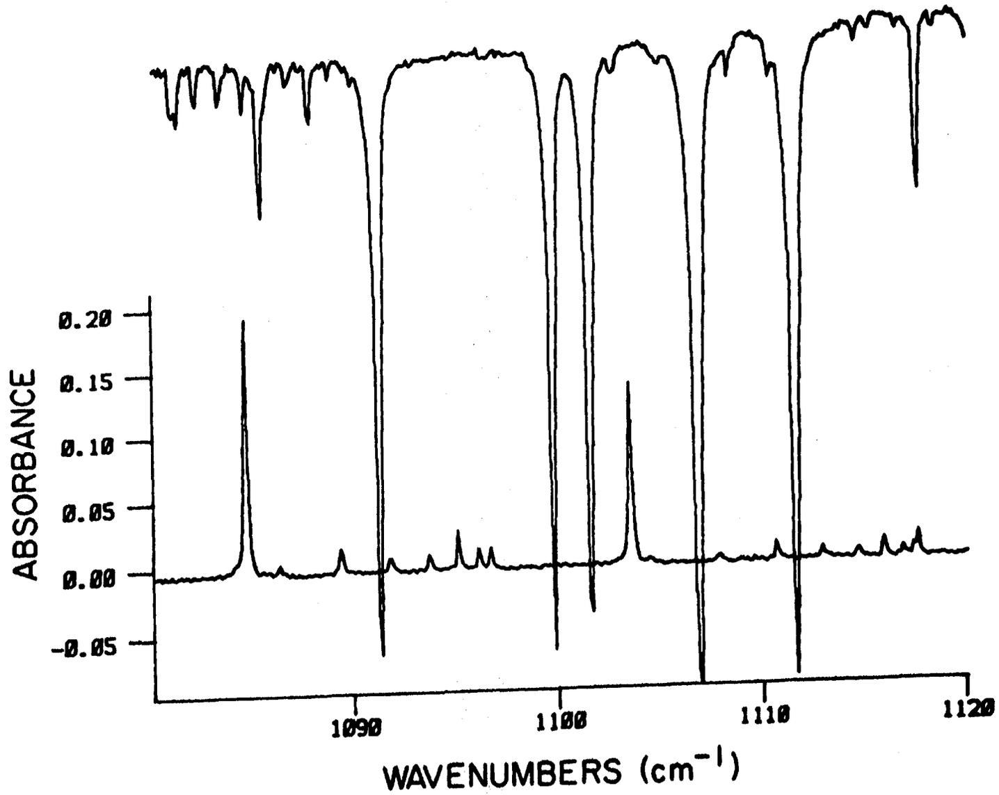
Figure V-5. Infrared absorption peaks of NH<sub>3</sub> (lower trace) relative to atmospheric H<sub>2</sub>O and CO<sub>2</sub> absorptions (upper trace) in the 1080-1120 cm<sup>-1</sup> region.
