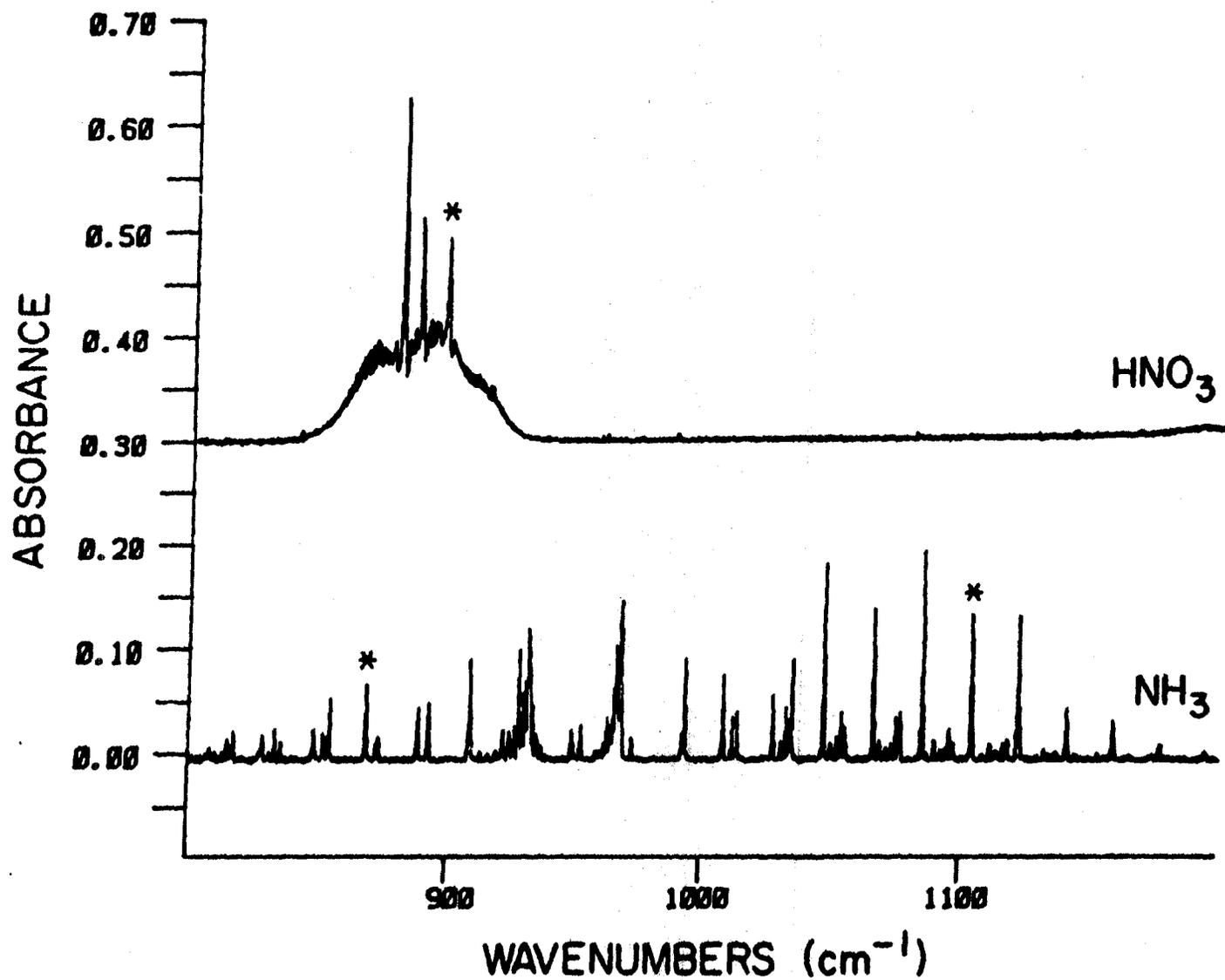
Figure V-3. Reference spectra of gaseous HNO<sub>3</sub> (0.61 torr) and NH<sub>3</sub> (0.23 torr) at spectral resolution of 0.125 cm<sup>-1</sup>, pathlength of 25 cm, total pressure with N<sub>2</sub> of 740 torr. The HNO<sub>3</sub> plot is offset by 0.30 absorbance (base 10) unit for clarity. Asterisks mark the absorption peaks used for analysis.
