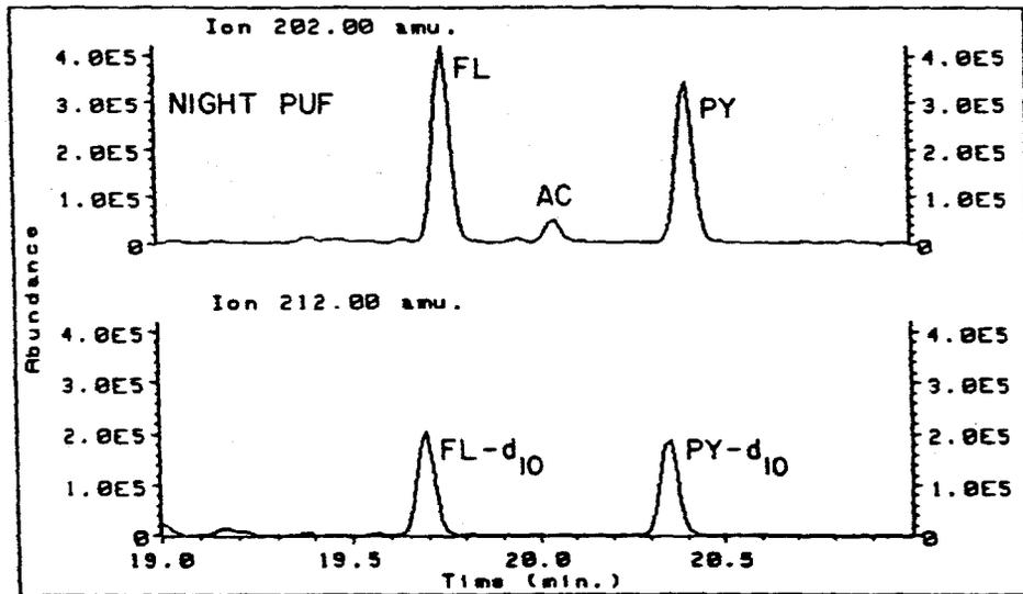
Figure VI-9. GC/MS-MID traces for the molecular ion of fluoranthene (FL), pyrene (PY) and acephenanthrylene (AC) [m/z 202] and the deuterated internal standards FL-d<sub>10</sub> and PY-d<sub>10</sub> (m/z 212) from the analyses of a daytime (top) and nighttime (bottom) ambient air sample collected on PUF plugs at Citrus College, Glendora, CA.
