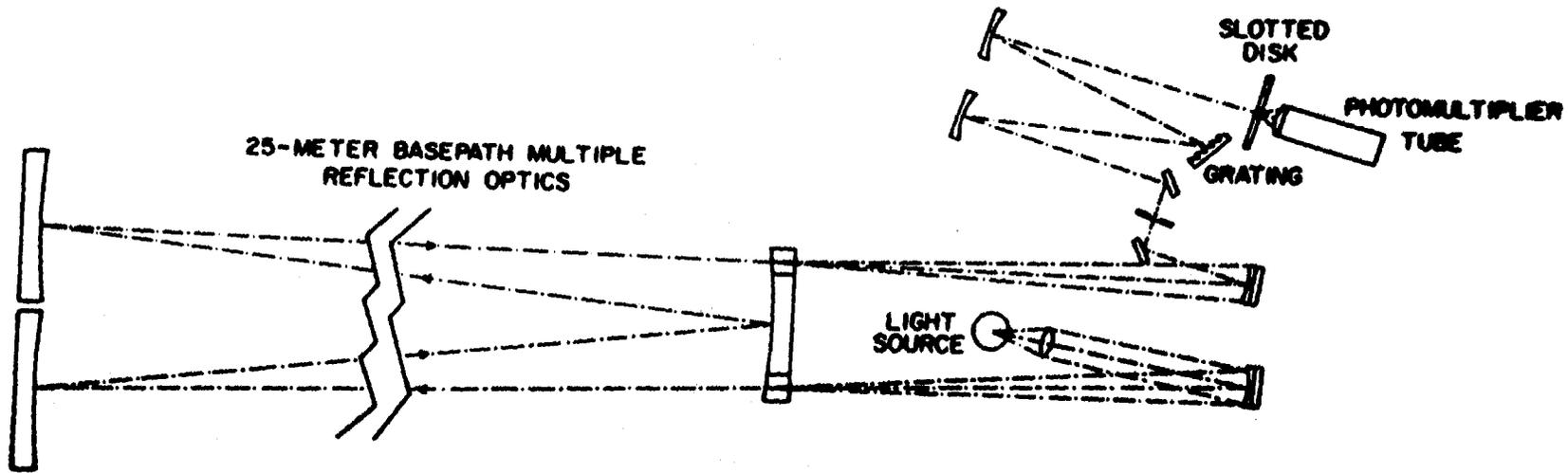
Figure IV-1. Schematic diagram of the longpath DOAS system.
