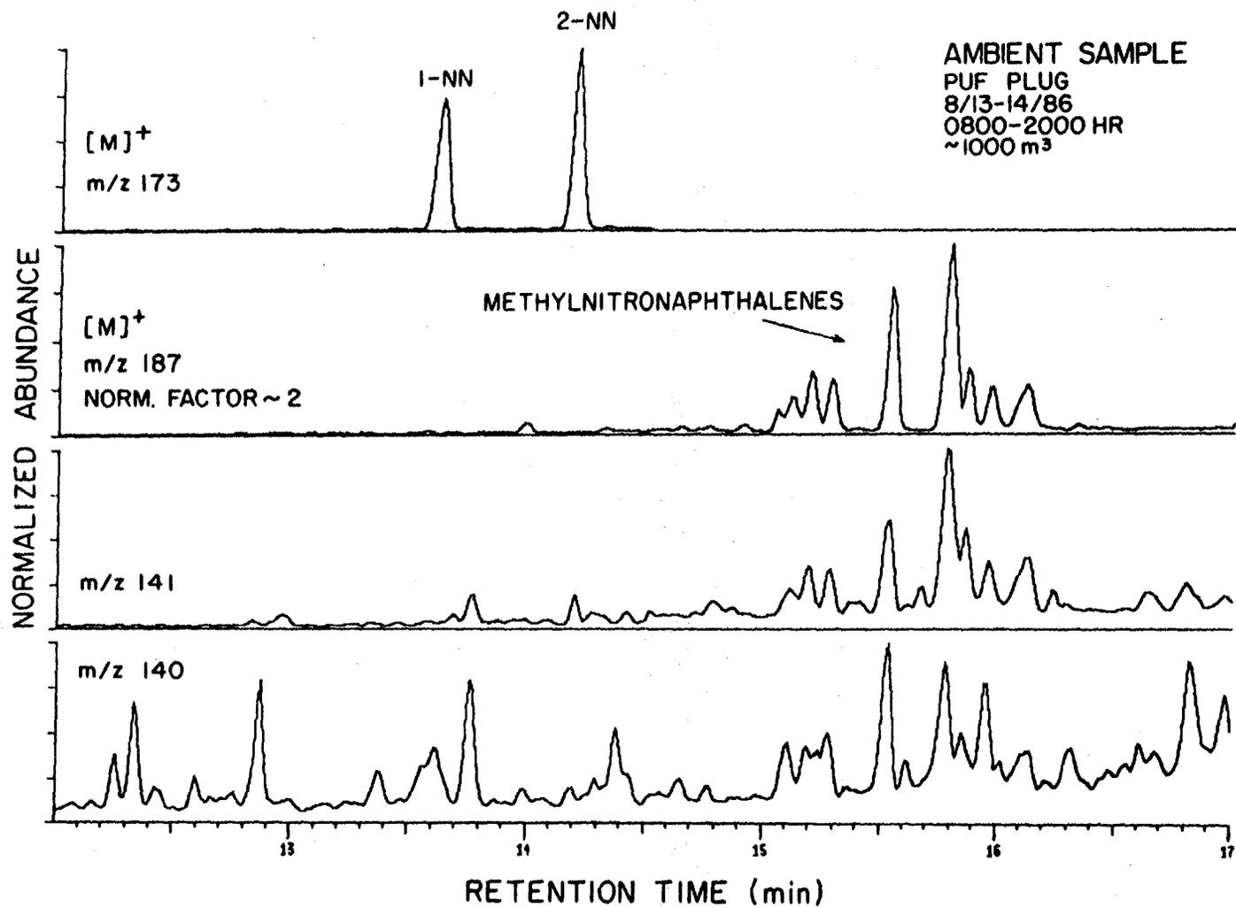
Figure VI-11. GC/MS-MID traces showing the presence of methylnitronaphthalenes in an ambient air sample collected on PUF plugs at Citrus College, Glendora, CA.
