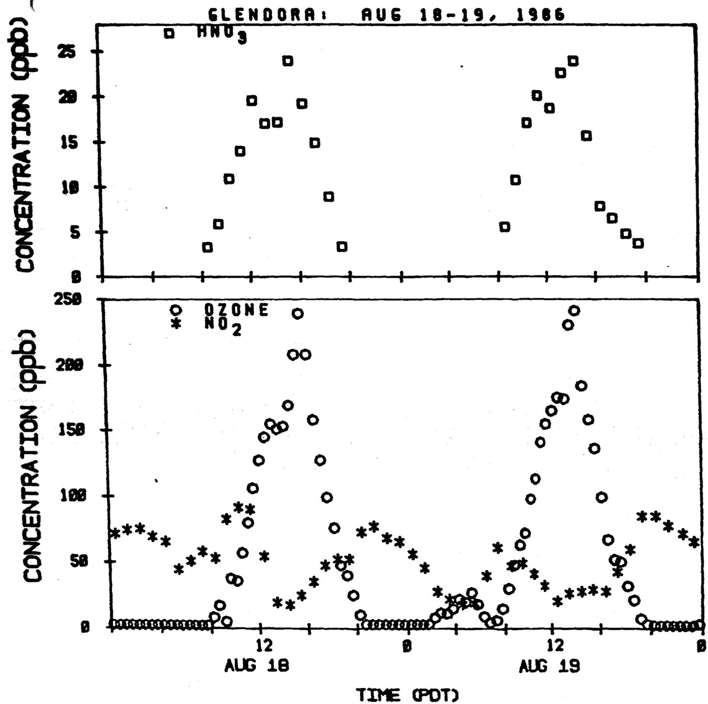
Figure V-8. Time-concentration plots of average HNO<sub>3</sub> (FT-IR), NO<sub>2</sub> (DOAS), and O<sub>3</sub> (Dasibi monitor) at Citrus College for August 18-19, 1986.
