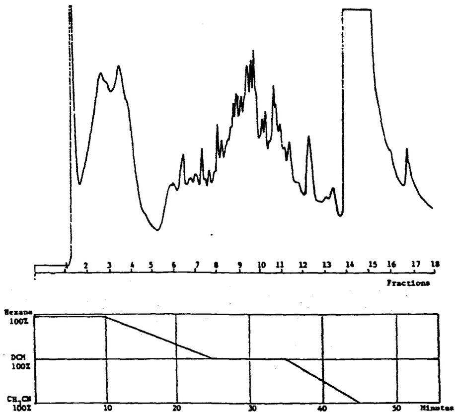
Figure VI-3. HPLC trace (254 nm) and gradient solvent program for separation of an ambient POM sample. Semi-preparative Ultrasphere Si column (1 cm x 25 cm), 3 mL min<sup>-1</sup>. HPLC fractions were combined as follows: #2-5, #6-7, #8, #9, #10-13, #14-18.
