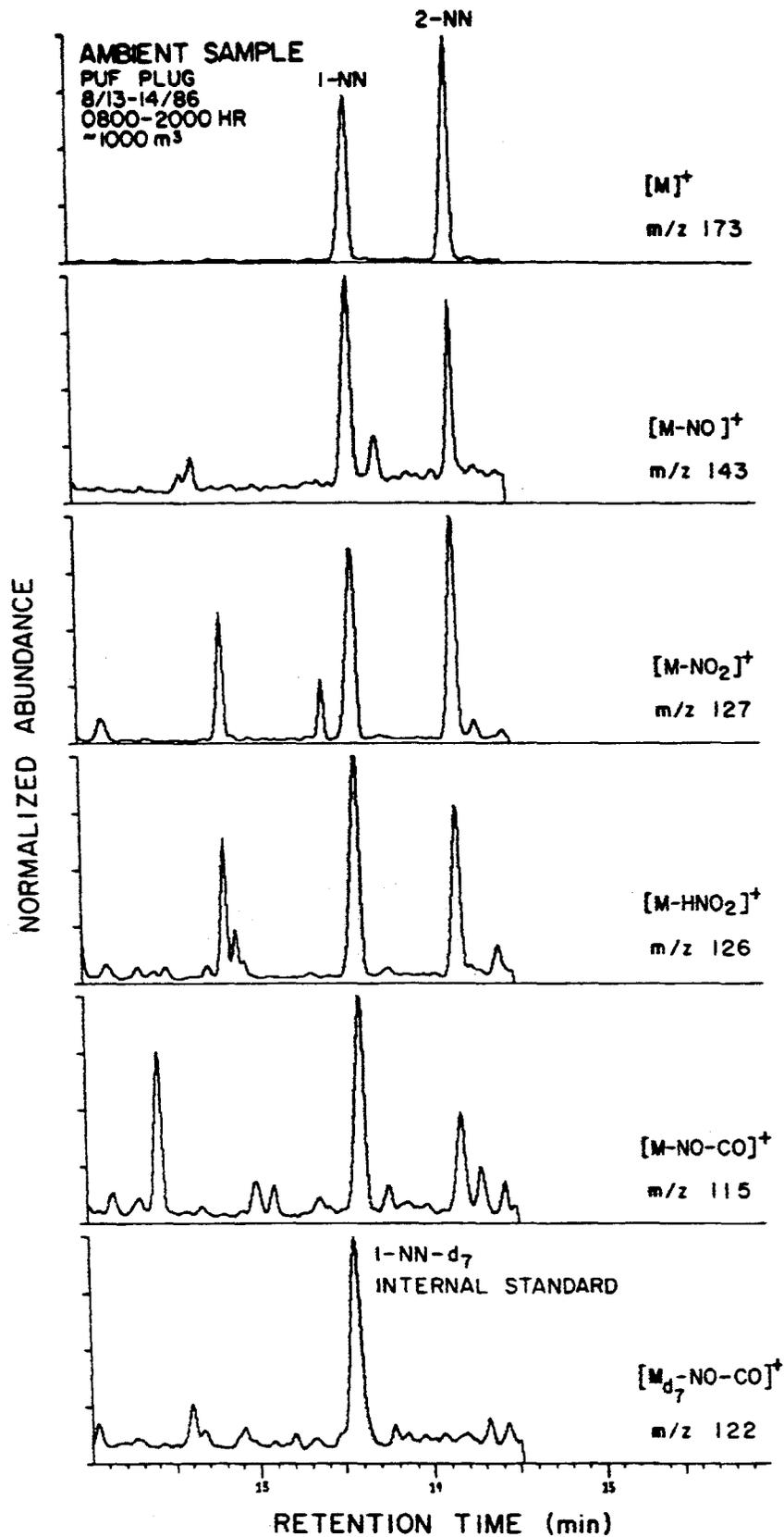
Figure VI-10. GC/MS-MID traces for the molecular ion ( $m/z$  173) and several characteristic fragment ions of 1- and 2-nitronaphthalene (NN) and an abundant fragment ion from the deuterated internal standard 1-NN-d<sub>7</sub> showing the presence of 1-NN and 2-NN in an ambient air sample collected on PUF plugs at Citrus College, Glendora, CA.
