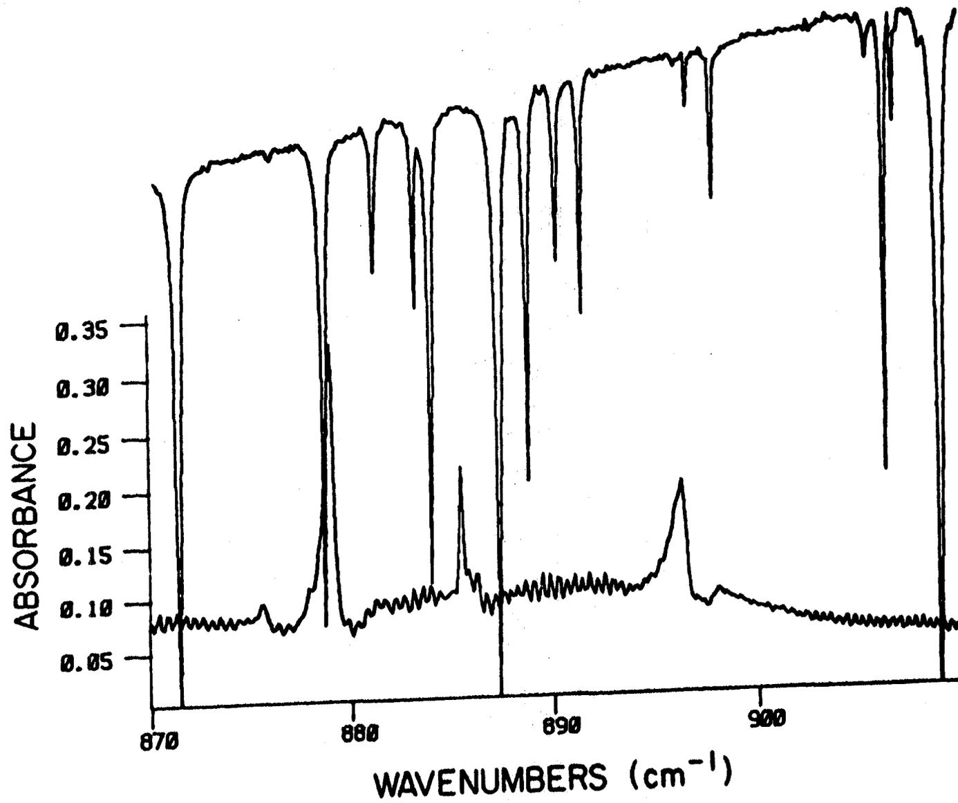
Figure V-4. Infrared absorption peaks of HNO<sub>3</sub> (lower trace) relative to atmospheric H<sub>2</sub>O absorptions (upper trace) in the 870-910 cm<sup>-1</sup> region.
