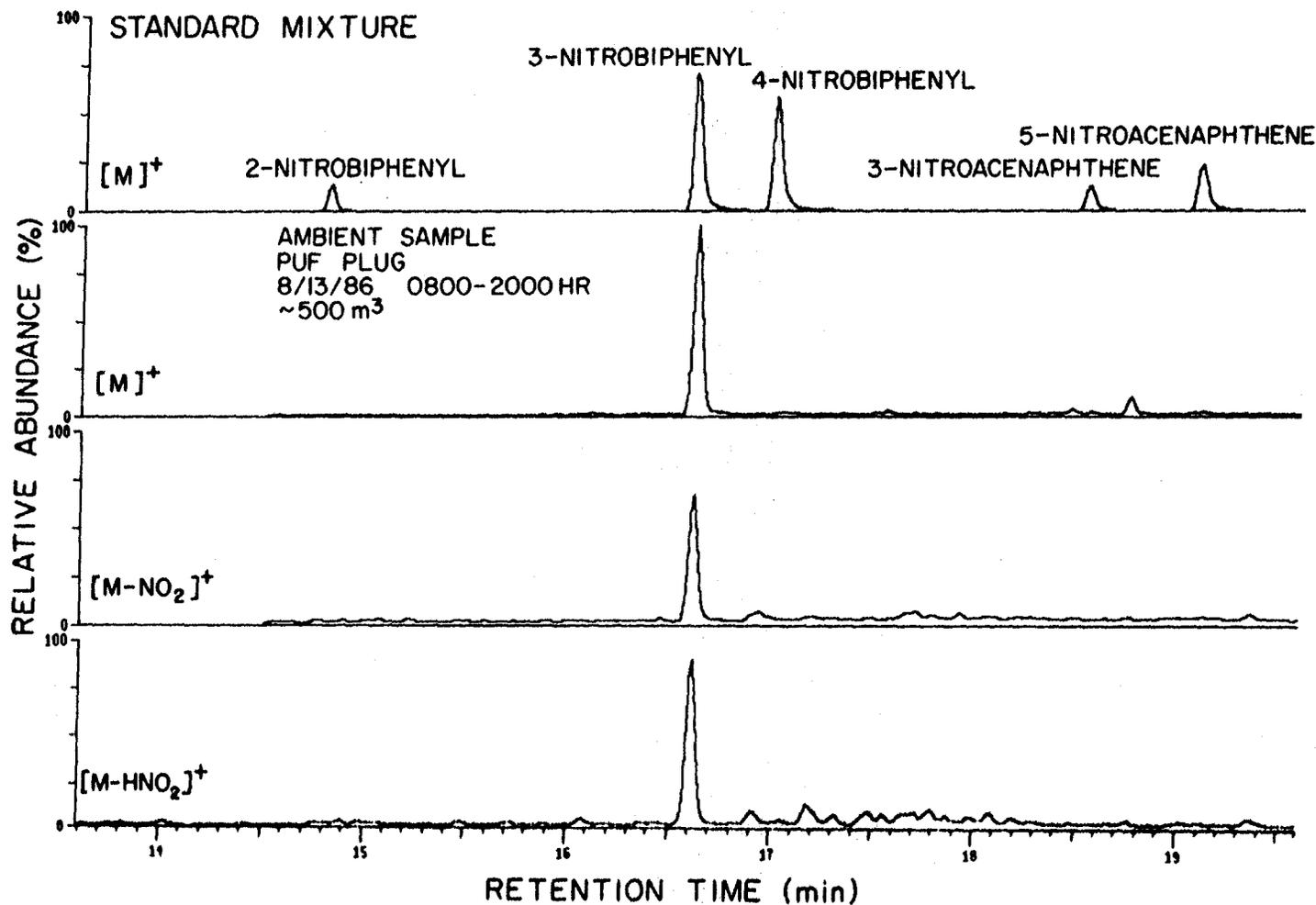
Figure VI-13. GC/MS-MID traces showing 3-nitrobiphenyl to be present in an ambient air sample collected on PUF plugs at Citrus College, Glendora, CA. The top trace repeats the molecular ion trace of the standard mixture (Figure VI-12) and it can be seen that the peak in the ambient sample (the molecular ion and two characteristic fragment ions shown) exactly matches 3-nitrobiphenyl in retention time.
