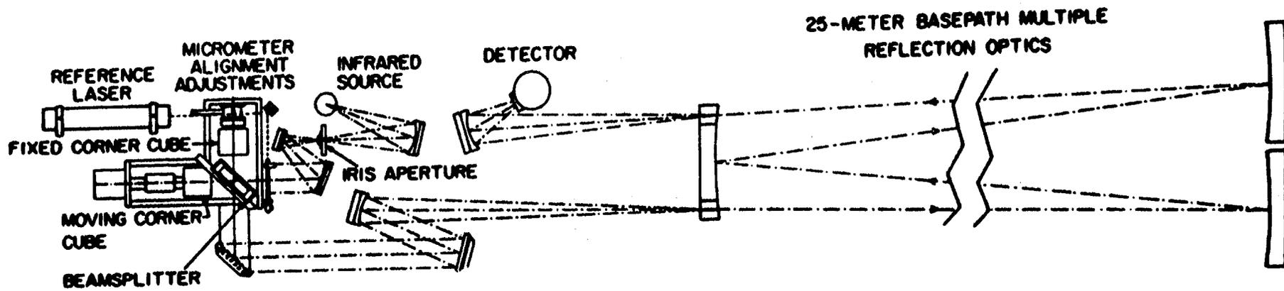
Figure V-2. Schematic optical diagram of the longpath FT-IR spectrometer.
