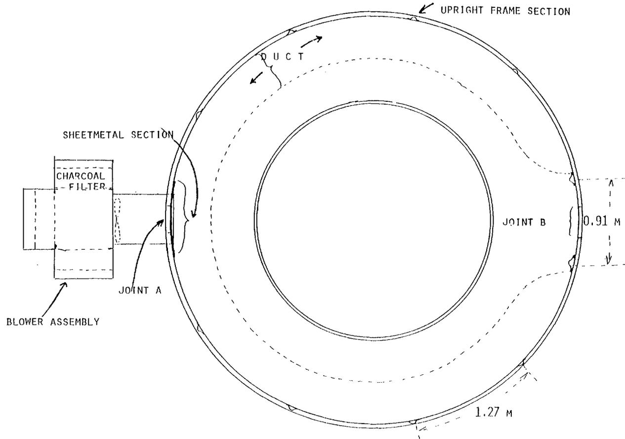
Figure A-3. Cross section of chamber and air handling system for orange open top field chamber.
