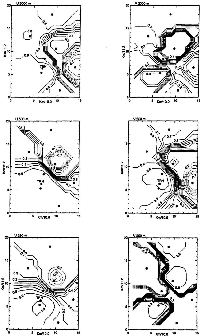
Figure 6.4. Spatial correlations between the TRN site and other grid points for  $u$ , (left panels) and  $v$ , (right panels) wind components. The correlations are for the morning average (0900-1100 PDT), for synoptic Case 1 at three levels. The dots show the profiler sites. The axes are multiplied by the same factors as in Fig. 6.1 to scale in kilometers.
