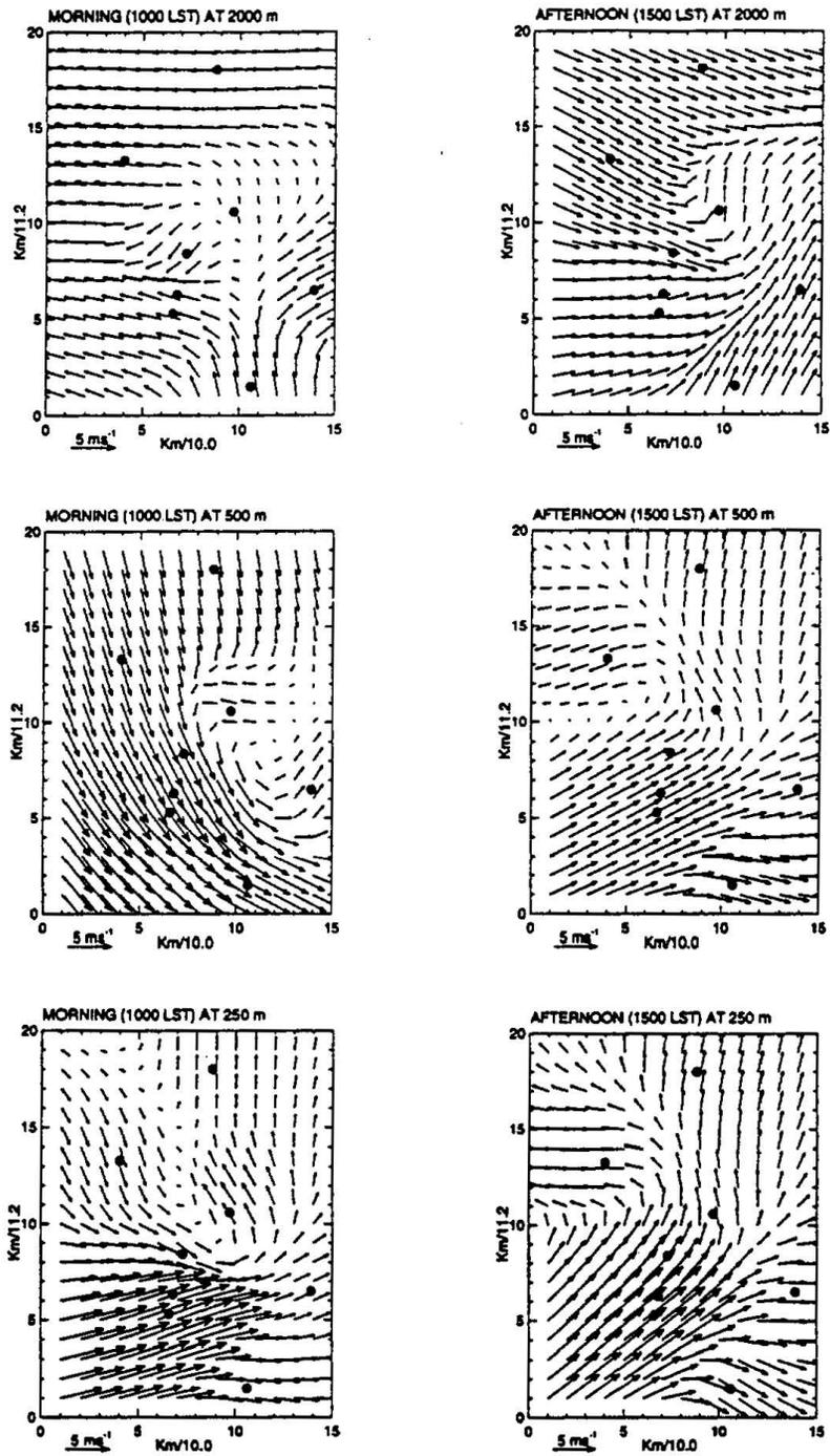
Figure 6.1 Wind speed and direction at three levels, for 1000 PDT (left panels) and 1500 PDT (right panels) for synoptic Case 1. The dots locate the wind profiler sites shown in Fig. 1. The east-west grid should be multiplied by 10 to scale in kilometers and the north-south axis by 11.2.
