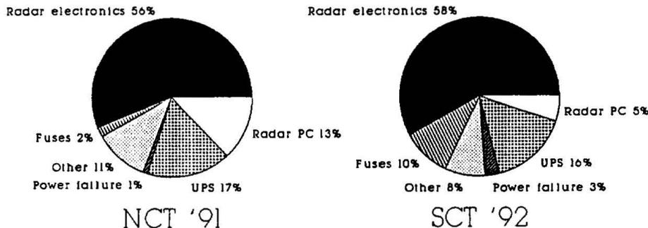
Figure 3. Causes of radar downtime during NCT'91 and SCT'92.
