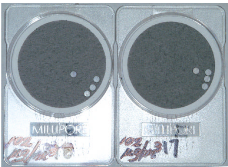
Figure 3. Pair of PM samples for carbon analysis collected simultaneously from each side of the chamber during exposure PM 40 on quartz fiber filters (QM-A, 47 mm diameter, Whatman, Inc., Clifton, NJ). Analysis of each filter resulted in identical concentrations of 102 \mu\text{g}/\text{m}^3 elemental carbon. Disks 3 mm in diameter were punched out of each filter for carbon analysis (Fung, 1990). Holes closer to the edge of a deposit were made to clean the punch mechanism before sample disks were removed.
