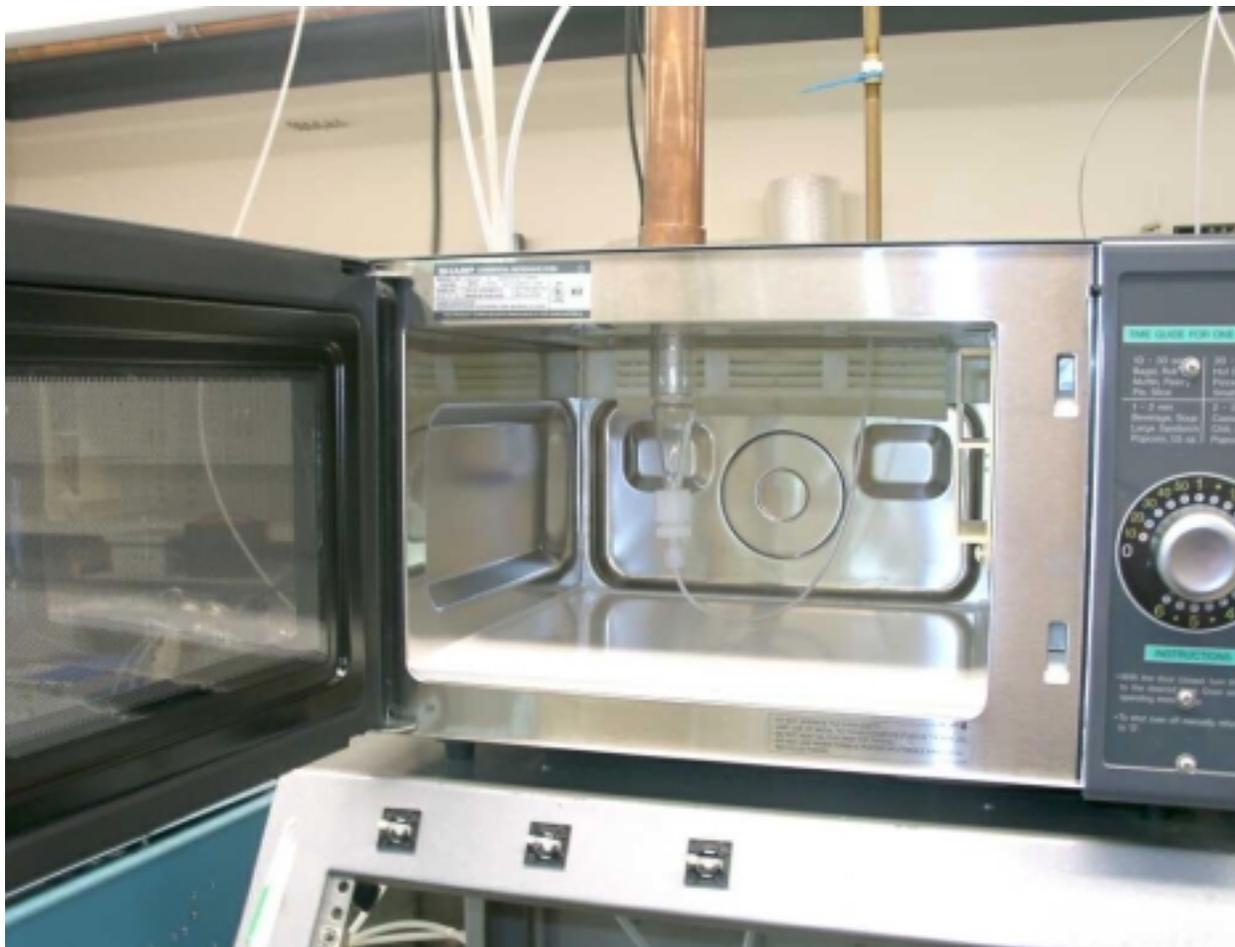
**Figure 2-4.** Microwave shielding tubes around the denuder assembly and sample line.
