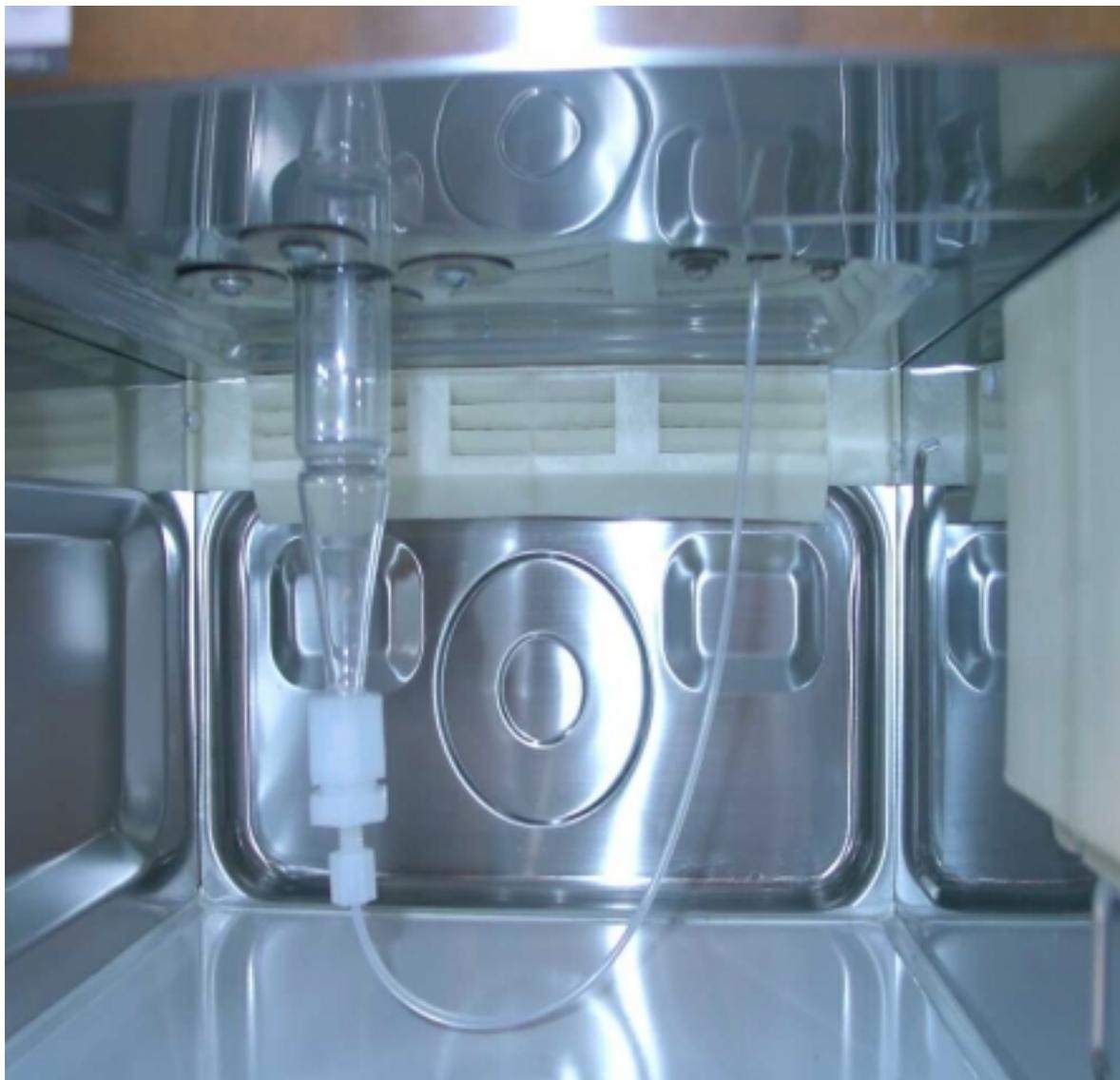
**Figure 2-3.** Interior of the microwave and the glass enclosure around the ceramic denuder.
