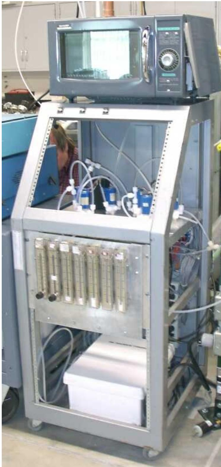
**Figure 3-2.** Photograph of the automated TED assembly.
