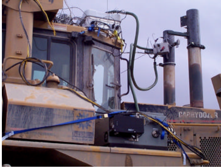
Figure 8 Caterpillar D-11R CD Track-Type Tractor Outfitted with WVU's Mobile Emissions Measurement System
