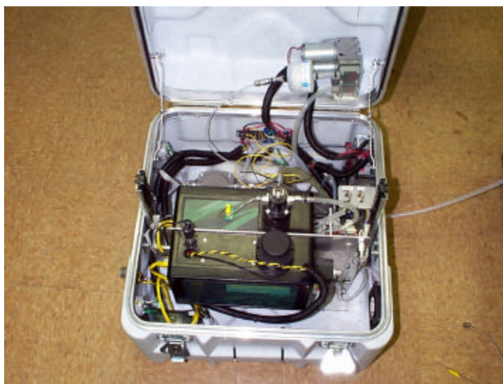
Figure 19 View of Internal Components of the MARI Real-Time Particulate Mass Monitor (RPM 100)
