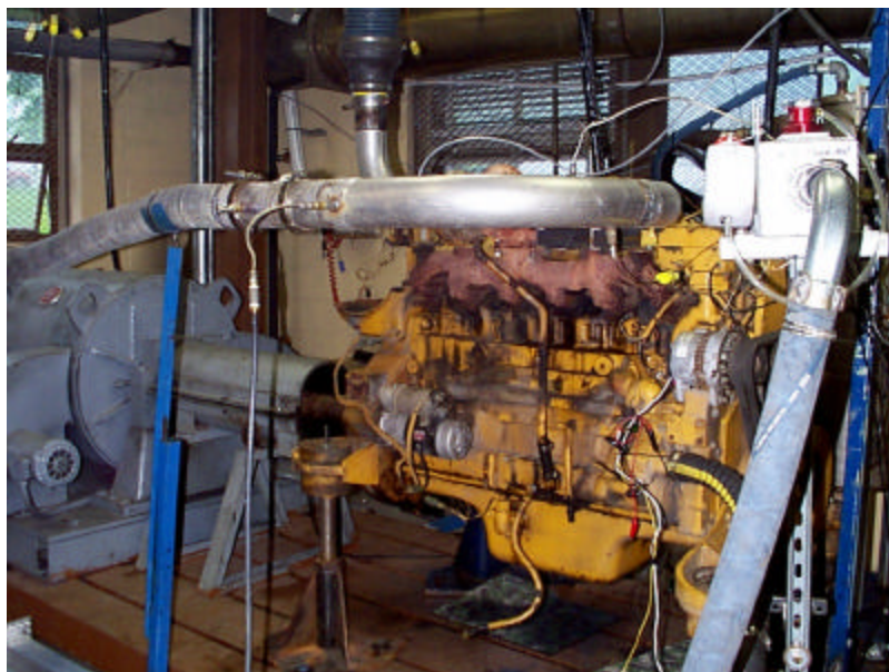
Figure 117 Komatsu S6D125-1 Engine mounted on GE DC Dynamometer test bed
