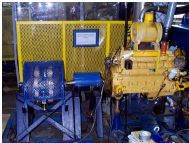
Figure 2 John Deere 6059D Engine on Eddy-Current Dynamometer Test Bed
