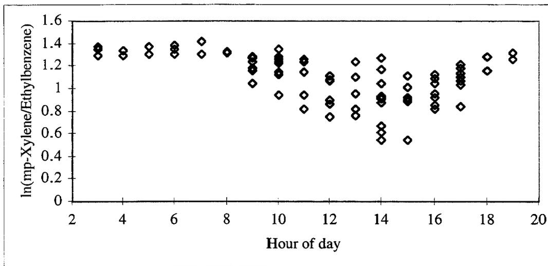
Figure 5-8: ln(m&p-xylene / ethylbenzene) versus hour of day.
