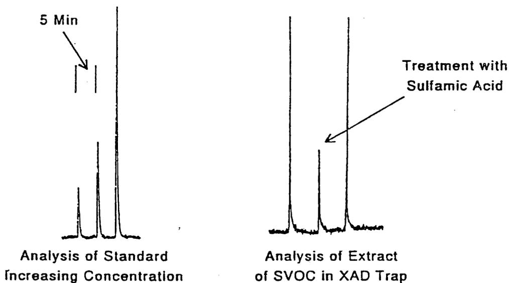
Figure 3. Repeat denitrosation analysis of an XAD extract of collected SVOC without and with treatment of the extract solution with sulfamic acid.
