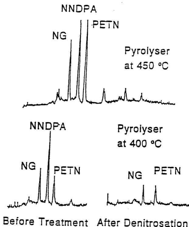
Figure 2. SFC chromatograms of a standard explosive mixture using chemiluminescence detection at a pyrolysis temperature of 450 and 400°C and at a pyrolysis temperature of 400°C after treatment of the sample with the acetic acid-HBr denitrosation reagent.
