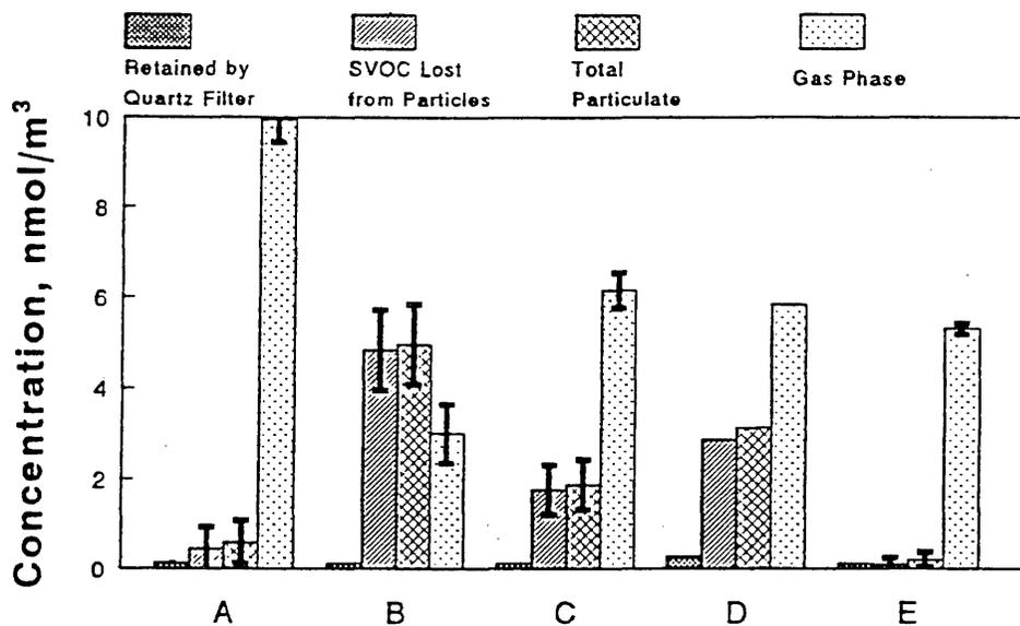
Figure 7. Concentration of nitrite material retained by particles on a quartz filter during sampling, lost from particles during sampling (SVOC Lost), and total particulate and gas phase nitrite material for each sample.
