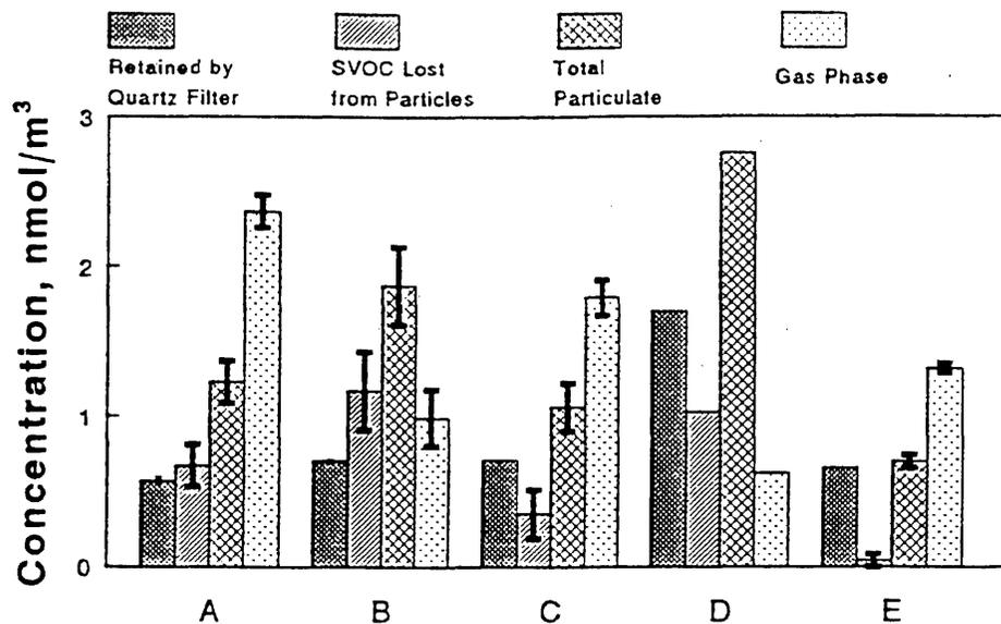
Figure 6. Concentration of N-nitroso material retained by particles on a quartz filter during sampling, lost from particles during sampling (SVOC Lost), and total particulate and gas phase N-nitroso material for each sample.
