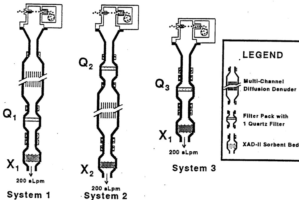
Figure 5. Schematic of the BOSS sampling system for the determination of gas and fine particulate N-nitroso and nitrite compounds.
