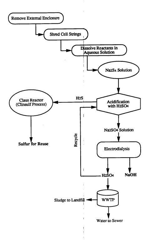
Figure 11. Silent power sodium-sulfur acidification process
