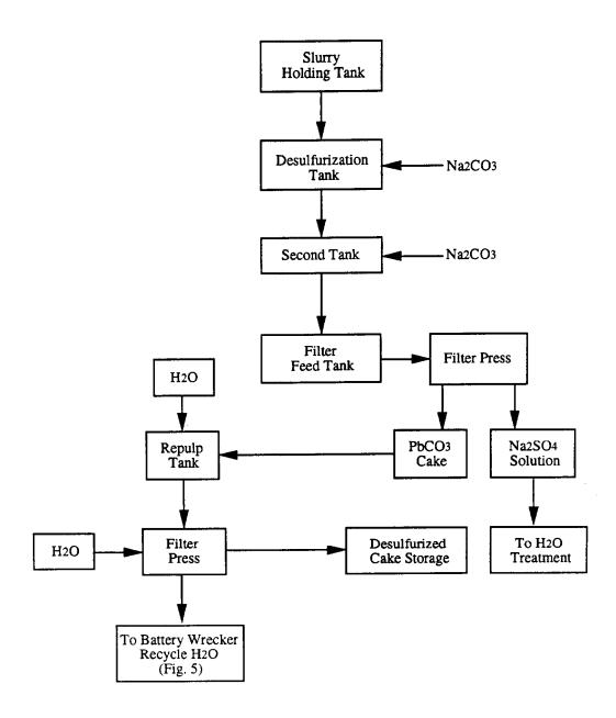
Figure 6. RSR's lead-acid battery paste desulfurization process (Reference 52)
