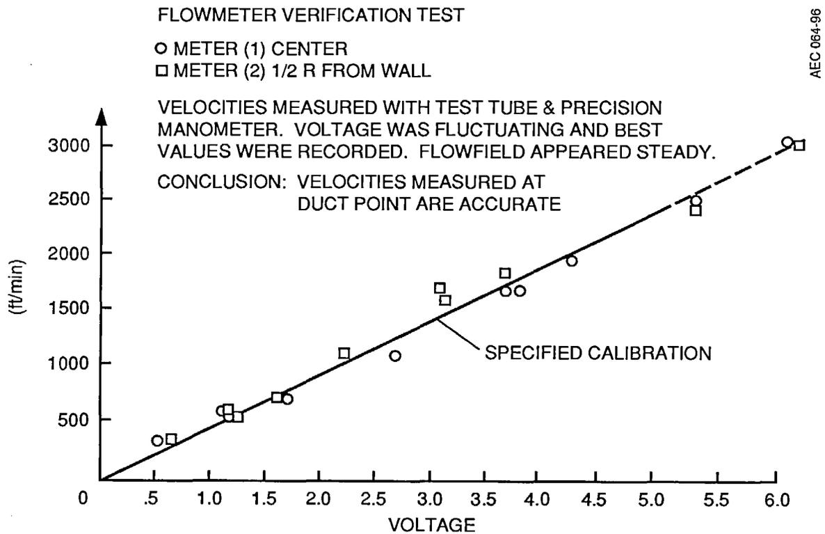
**Figure 3-10. Inlet air flow measurement test**
