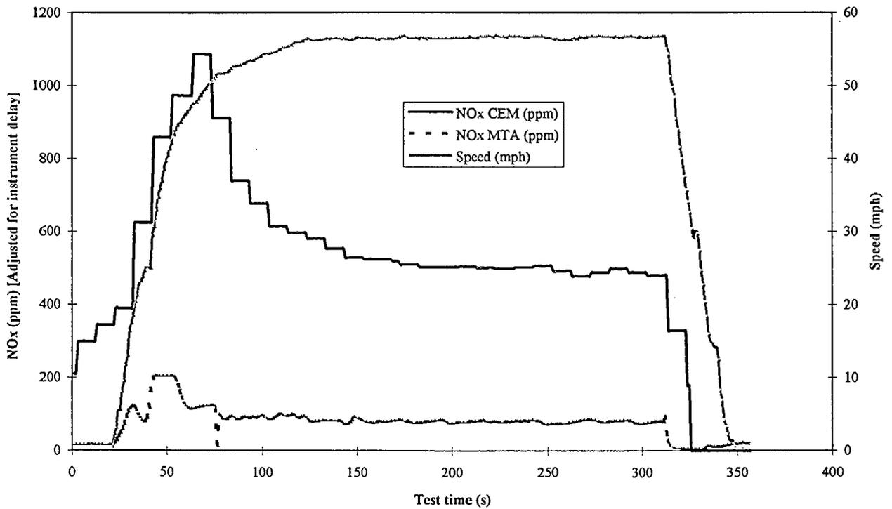
Figure 6-10. NO<sub>x</sub> ppm, Test 1063, Commuter, May 10, 1994, 10:57 a.m.
