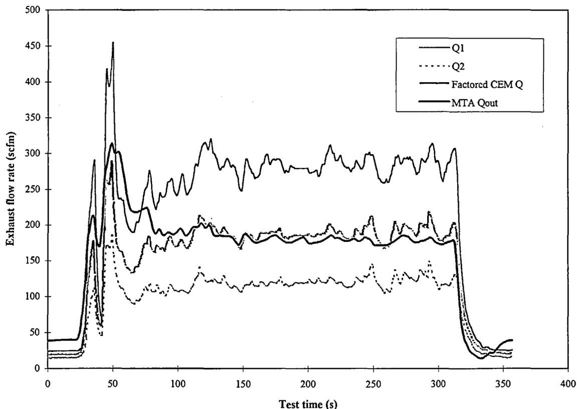
**Figure 6-7. Exhaust flowrate, Test 1063, Commuter, May 19, 1994, 10:57 a.m.**
