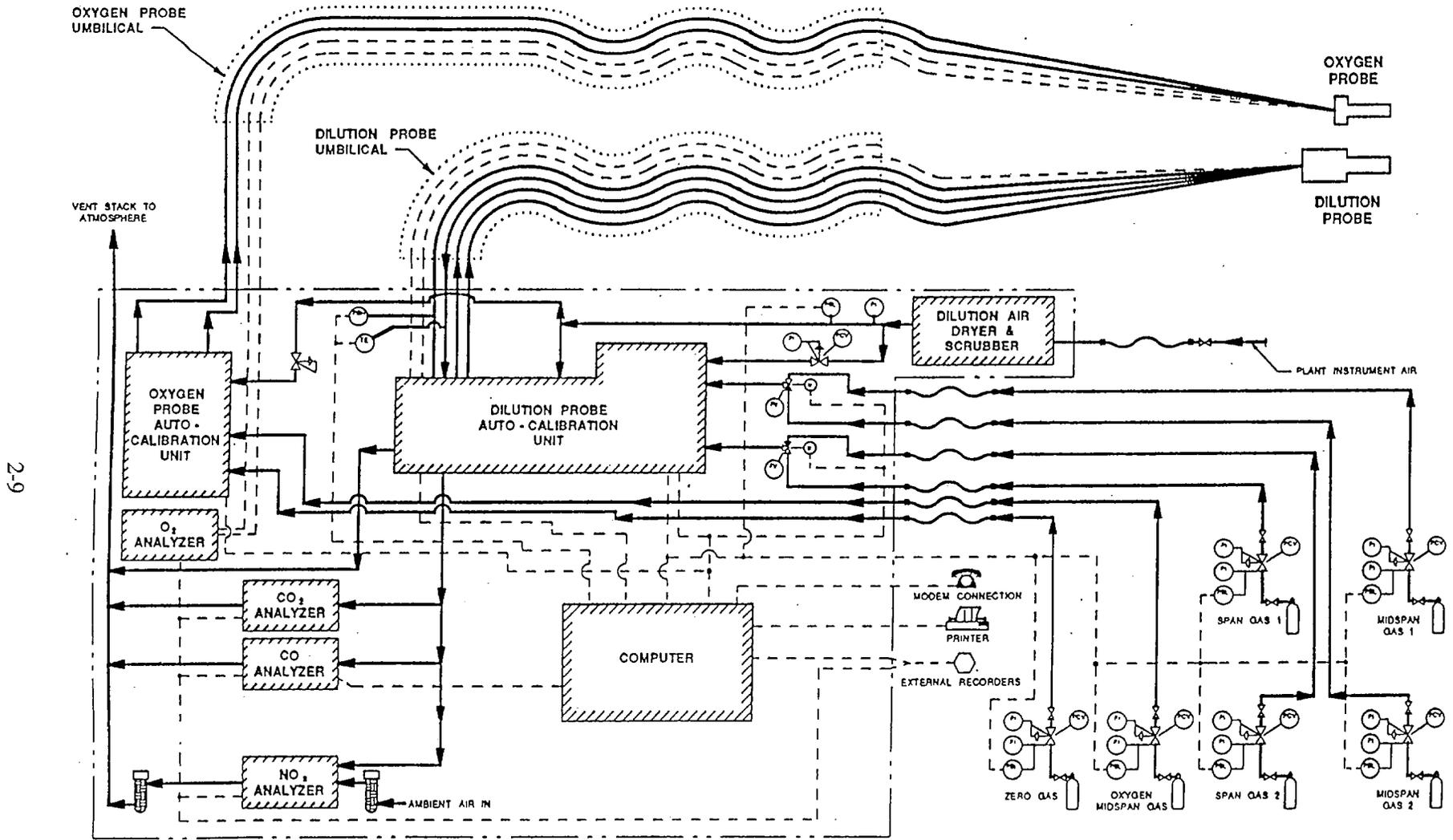
Figure 2-2. Process and instrumentation diagrams of the extractive filtration system
