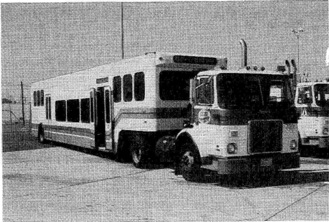
**Figure 3-1. OCTA Superbus #7001. The Superbus is a tractor-trailer configuration with the trailer providing passenger seating and the tractor servicing as the segregated power source to move the trailer**
