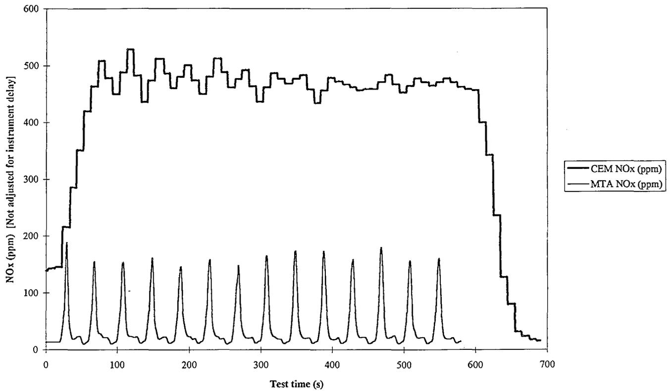
Figure 6-3. NO<sub>x</sub> ppm, Test 1055, CBD, May 9, 1994, 11:46 a.m. (not adjusted for time delay)
