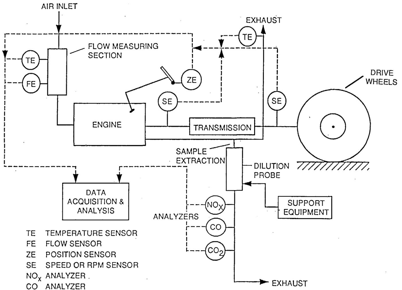
**Figure 2-1. Emission sampling system**
