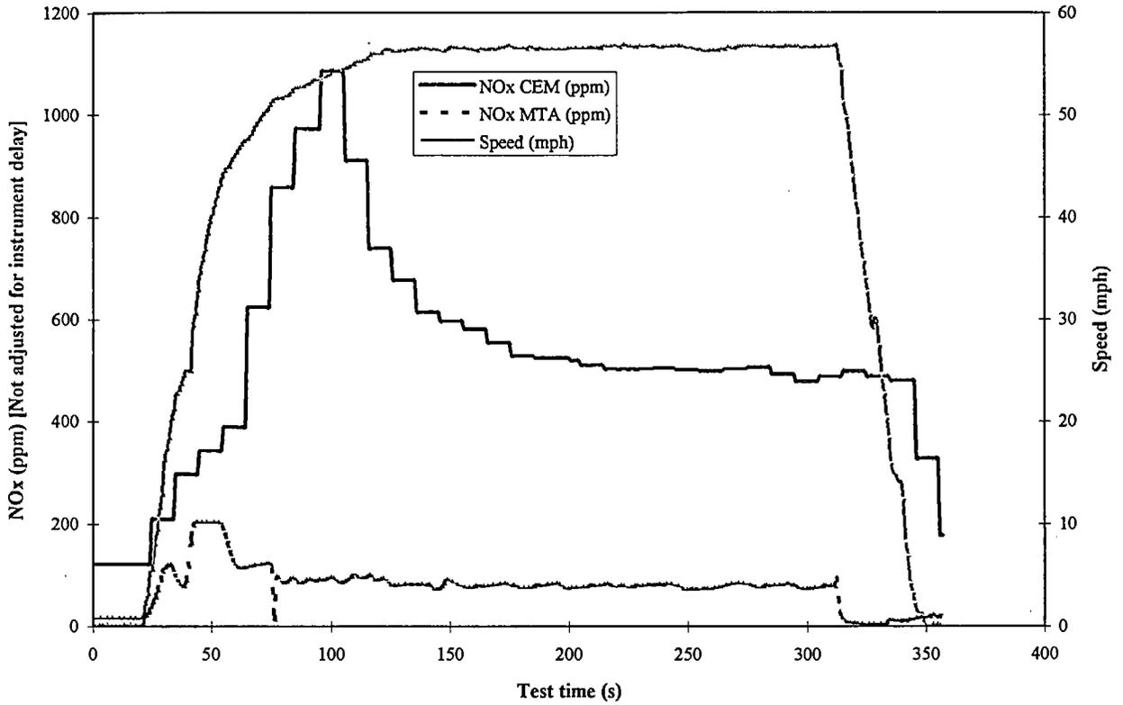
Figure 6-9. NO<sub>x</sub> ppm, Test 1063, Commuter, May 10, 1994, 10:57 a.m.
