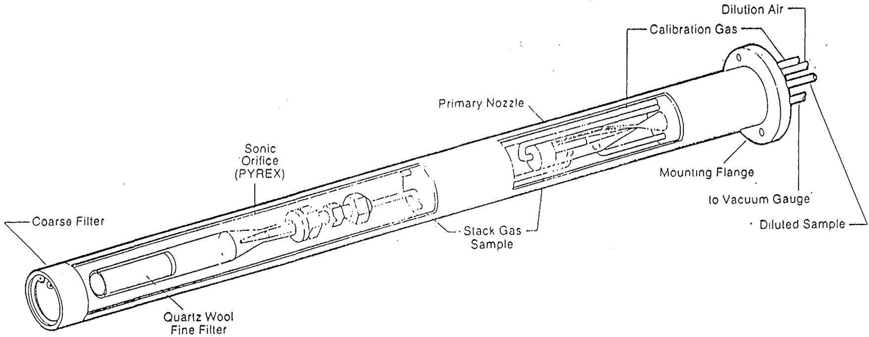
Figure 2-3. Dilution probe
