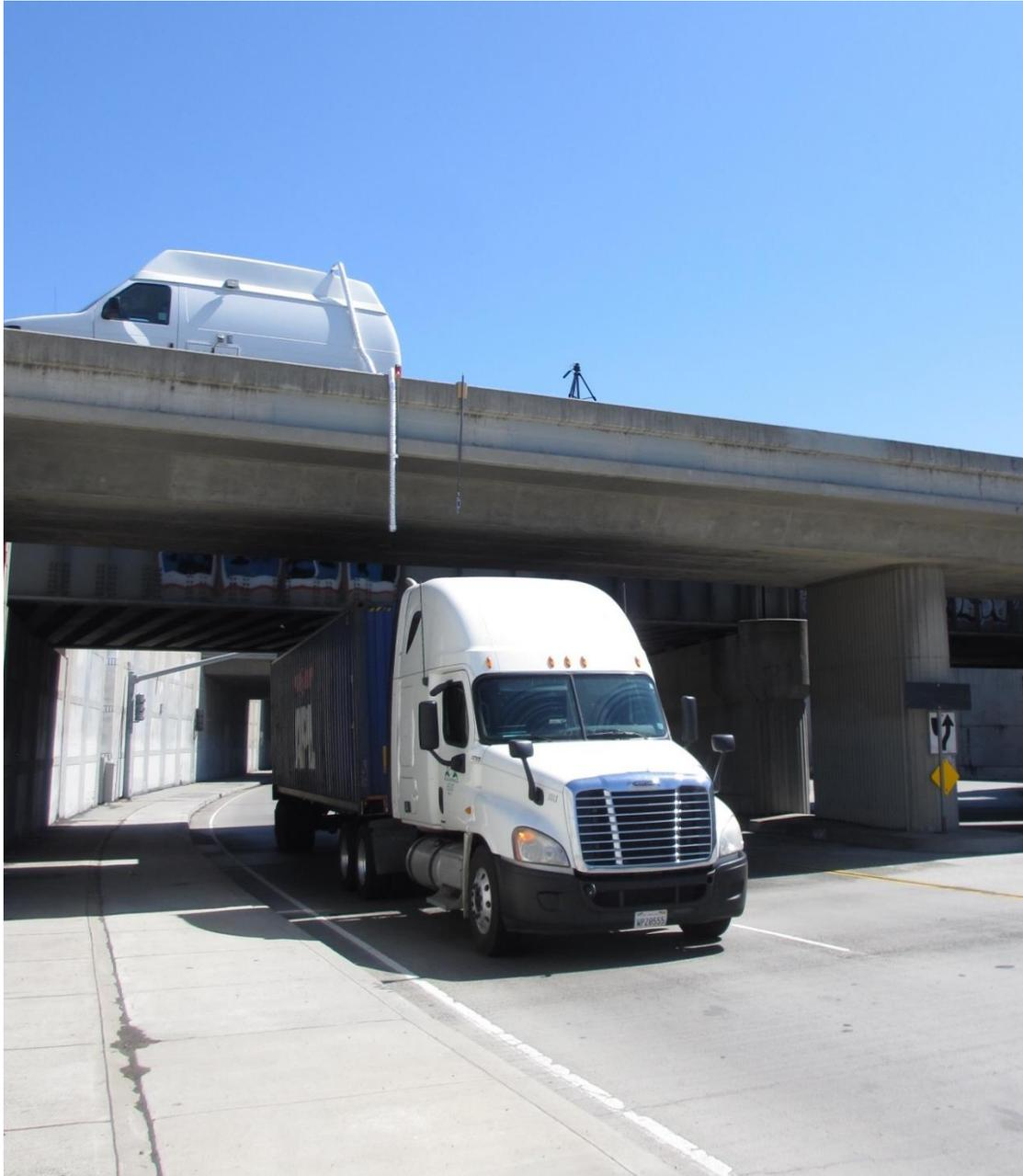
**Figure 1.** Instrumented van positioned on an overpass sampling the exhaust from a truck en route to the Port of Oakland.
