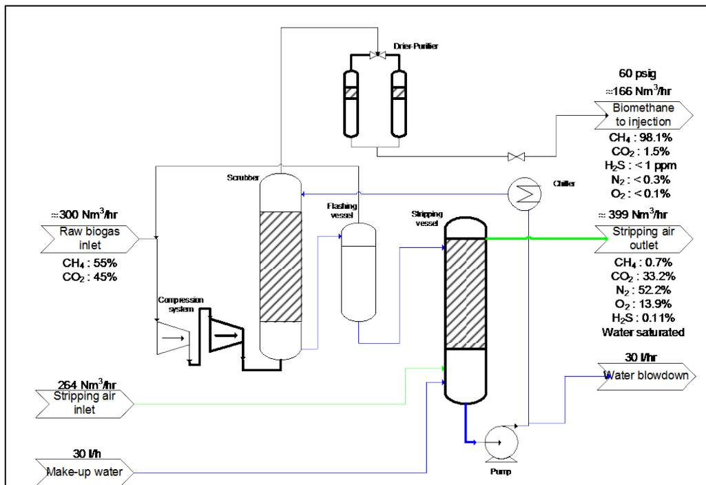
Figure 18. Upgrading schematic for dairy biogas from Electrigaz (2011)
