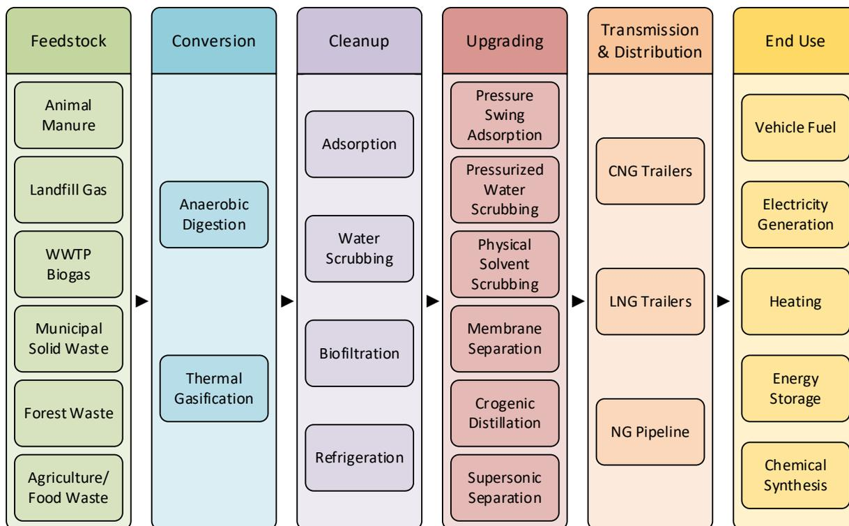
Figure 16: Schematic of RNG production from feedstock through to end use.
