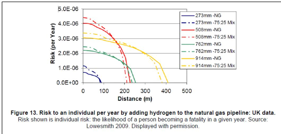
Figure 28. Risk to an individual per year by adding hydrogen to the natural gas pipeline: UK data.
