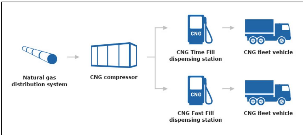
Figure 8. CNG supply pathway
