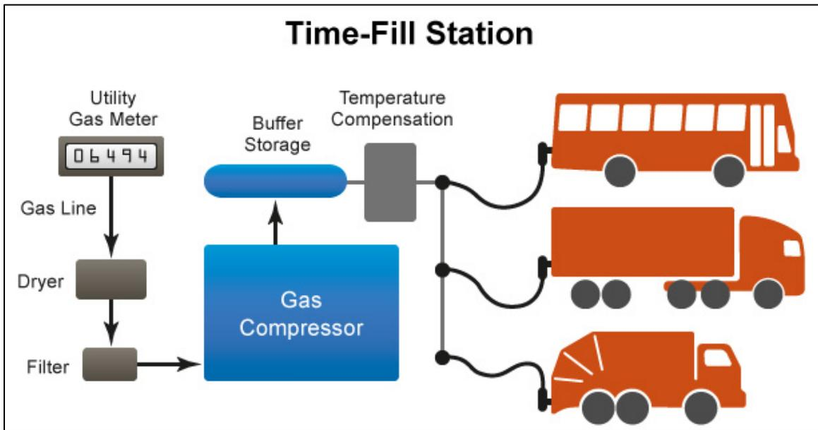
Figure 9. CNG Time fill station configuration
