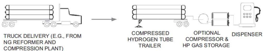
Figure 16c. Hydrogen station with compressed gas truck delivery
