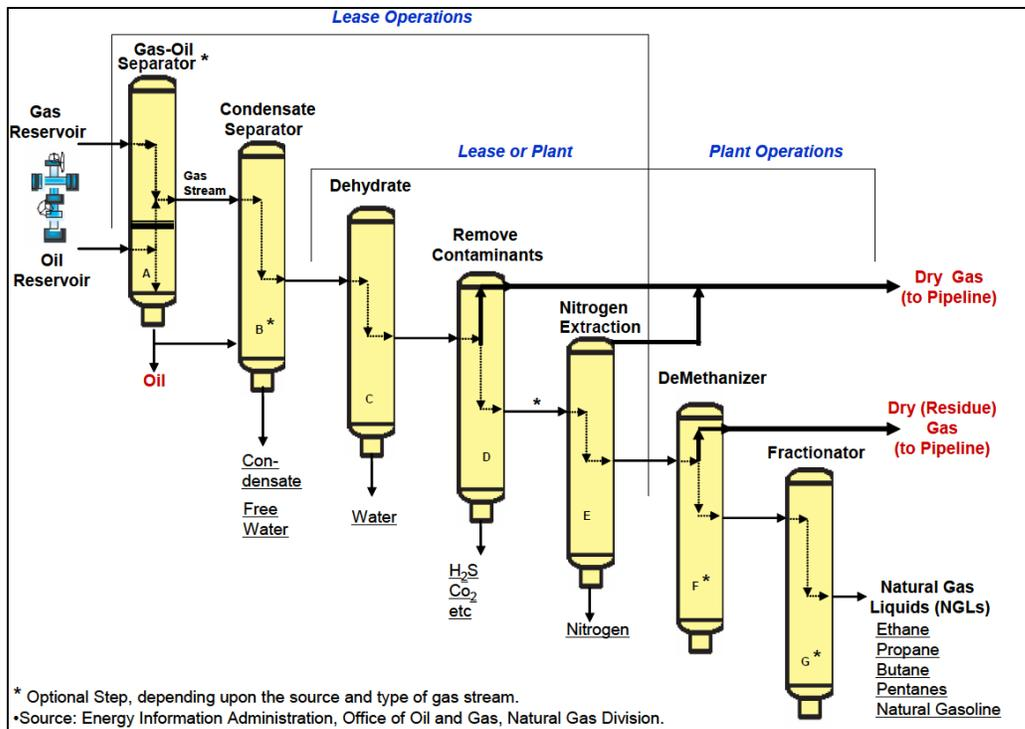
Figure 17. Generalized Natural Gas Processing Schematic from Electrigaz (2011)
