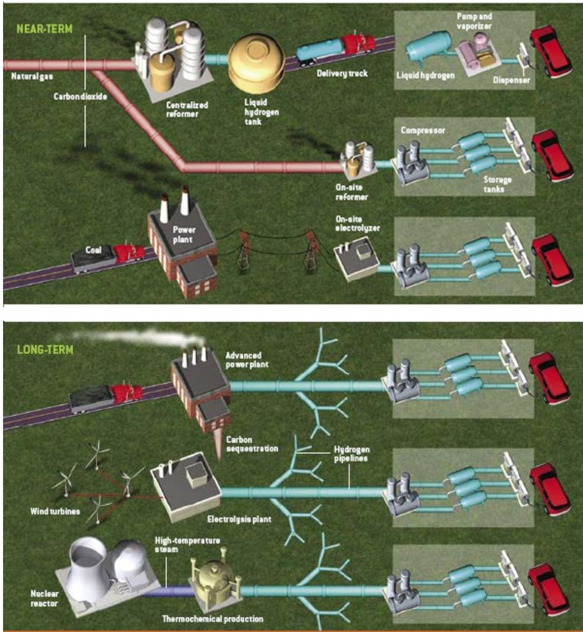
Figure 14. Near Term and Long Term Pathways for Hydrogen Production and Delivery to Vehicles. (It is also possible to deliver hydrogen via compressed gas truck.)
