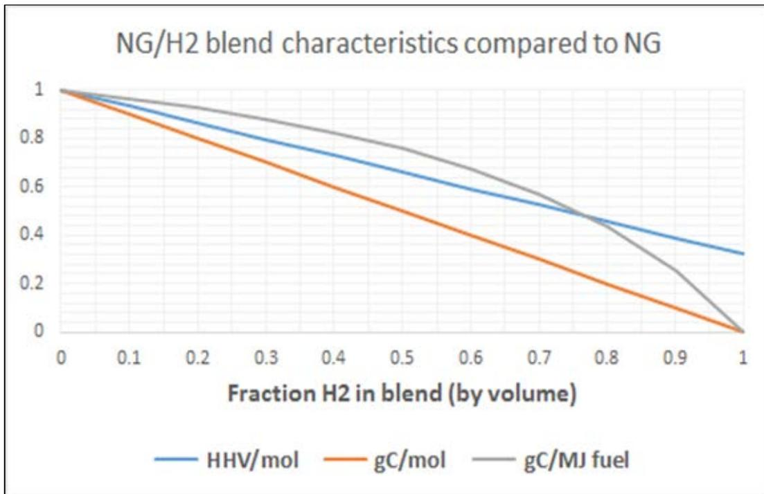
Figure 29. Effect of blending green hydrogen with natural gas on fuel gas energy and carbon content. The y-axis shows the fraction compared to pure natural gas.
