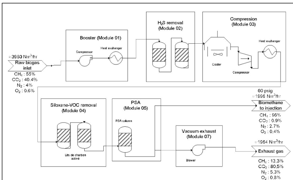
Figure 19. Upgrading schematic from LFG from Electricgaz (2011).
