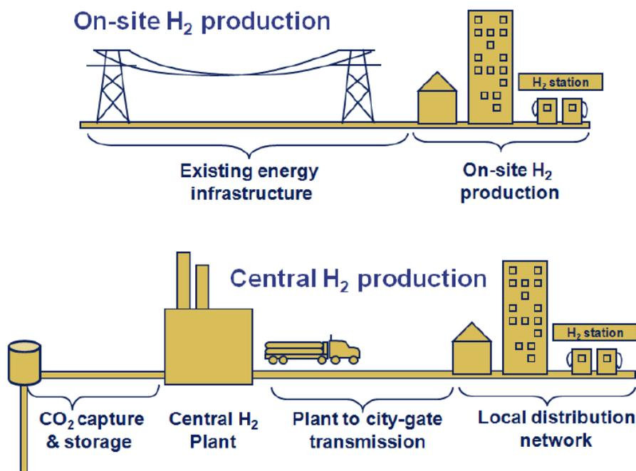
Figure 13. Centralized and onsite hydrogen infrastructure pathways for providing hydrogen transportation fuel.<sup>69</sup>
