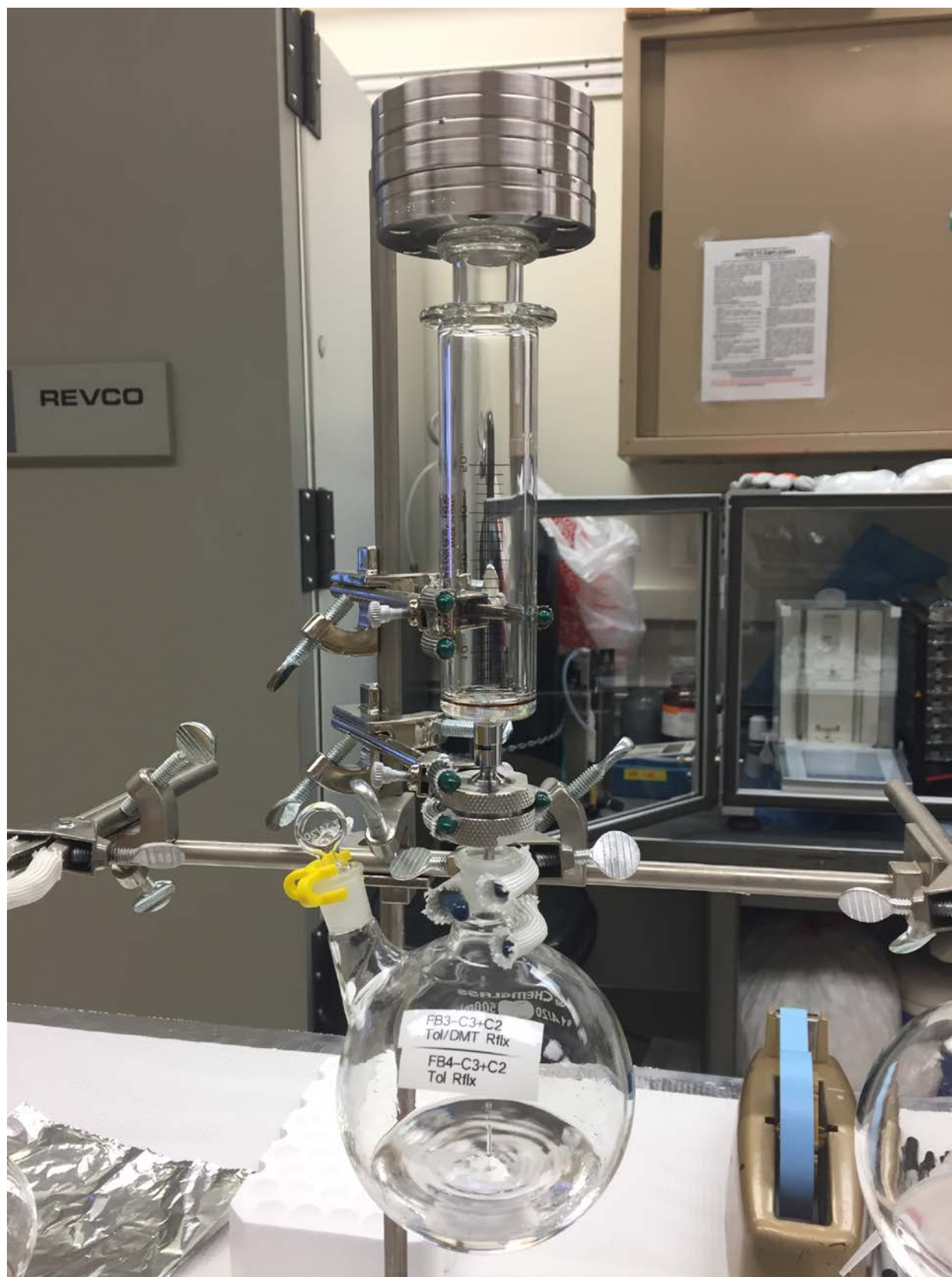
Figure 3. A picture of the syringe filtration apparatus; see text for details.
