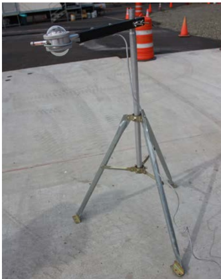
Figure 2. Albedo measurement system with a dual-pyranometer albedometer. Note that the albedometer is normally placed closer to pavement than shown here.
