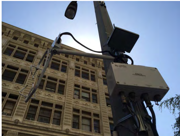
Figure A2: Sonic anemometer and AQMesh monitor mounted to light pole next to 8th St.
