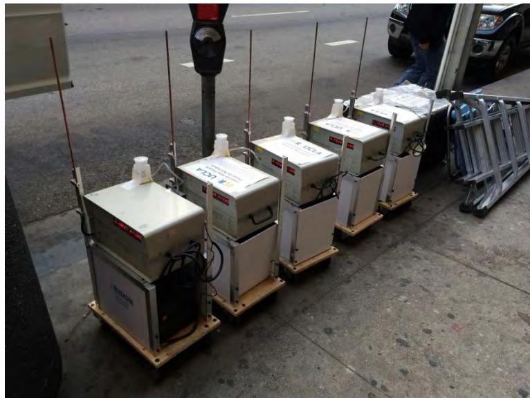
Figure A3: Co-location of CPCs before start of measurements on 8th St.
