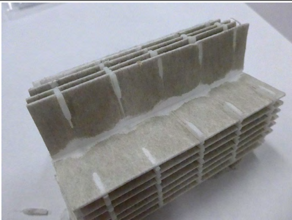
Figure 1: uniform soiling of very fine dust on the “EE” placebo filter
