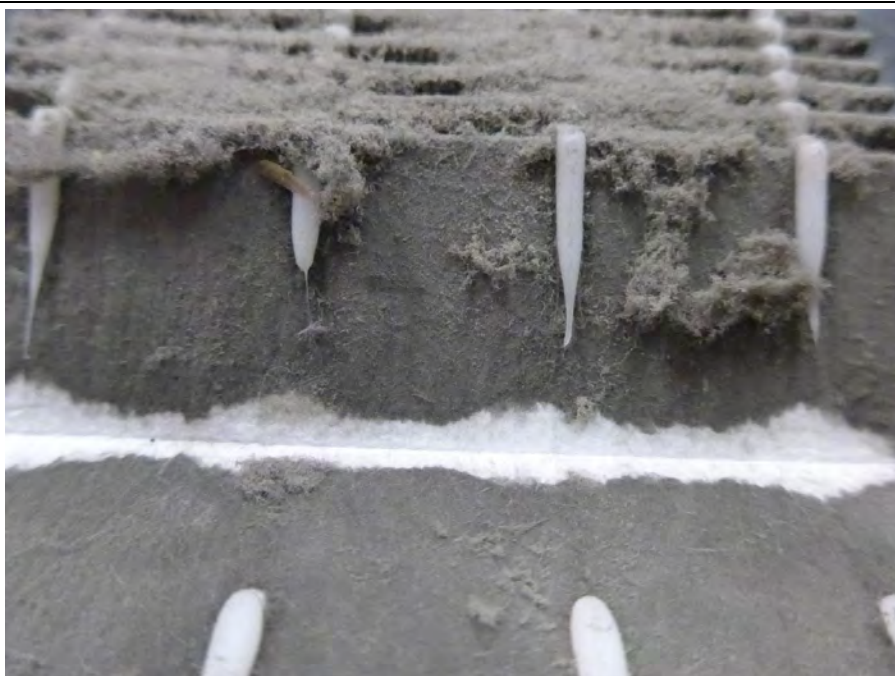
Figure 6: coarse dust found at the bottom of the pleats
