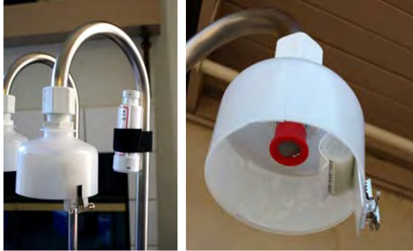
Figure 2. Position of Ogawa badge in the inlet stream.
