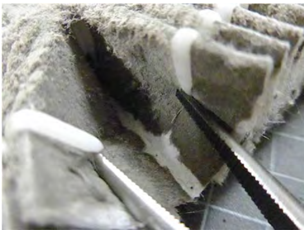
Figure 4.4 Coarse dust drawn down into the pleats due to airflow through the real filter.
