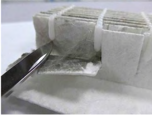
Figure 4.2 Dust on the surface of the sham filter.
