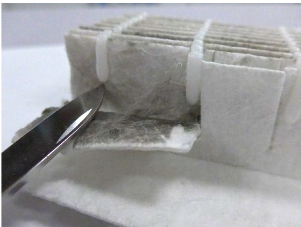
Figure 2: dust on the surface of the “EE” filter
