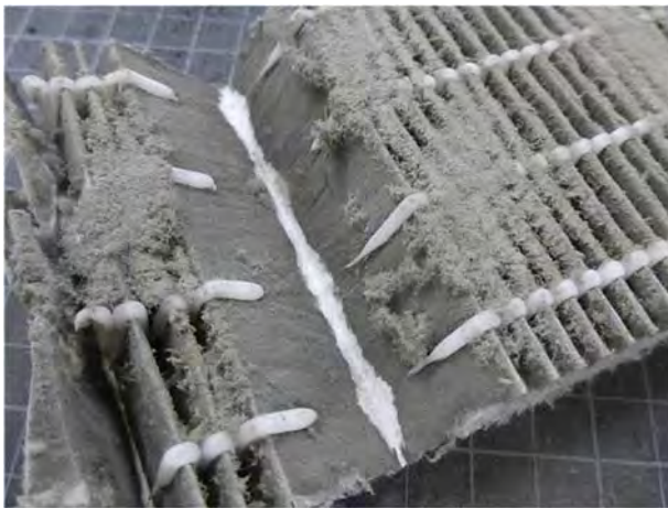
Figure 4.3 Dust piles are predominantly coarse dust on a used true filter.
