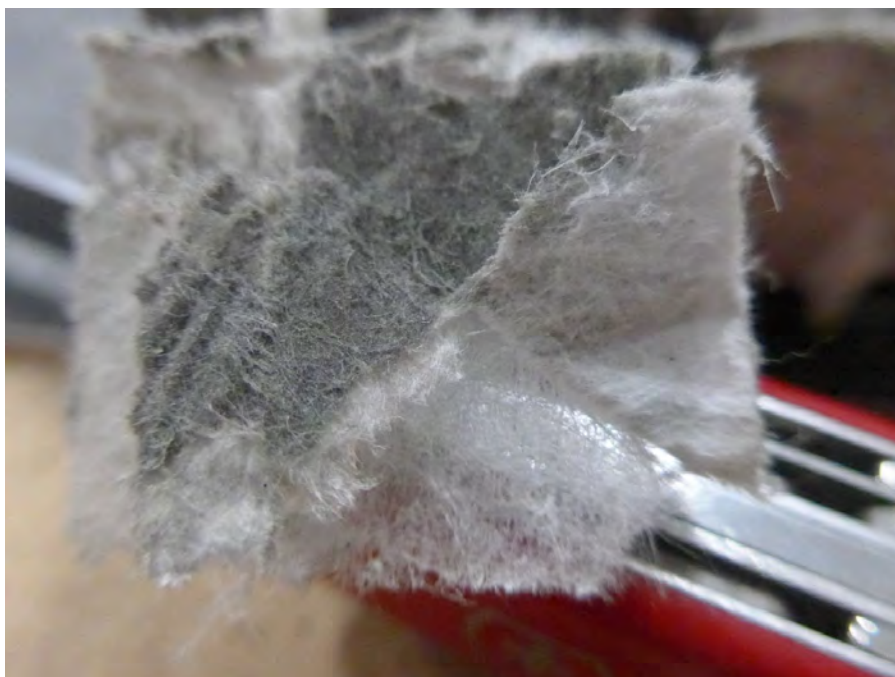
Figure 7: torn cross section of "E" filter media shows coarse as well as very fine dust
