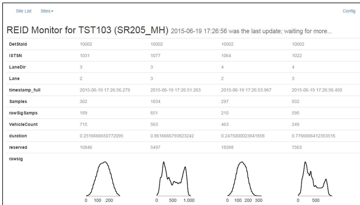
Figure 5-9 Graphical representation of signatures streaming live from SR-205 at Mountain House Parkway
