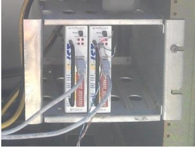
Figure 5-2 A modified 222 Input File fabricated for the IST-222 LSM Adapter
