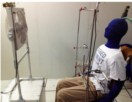
Figure 41 Convective heat transfer coefficient measurement with manikin 'Newton'
