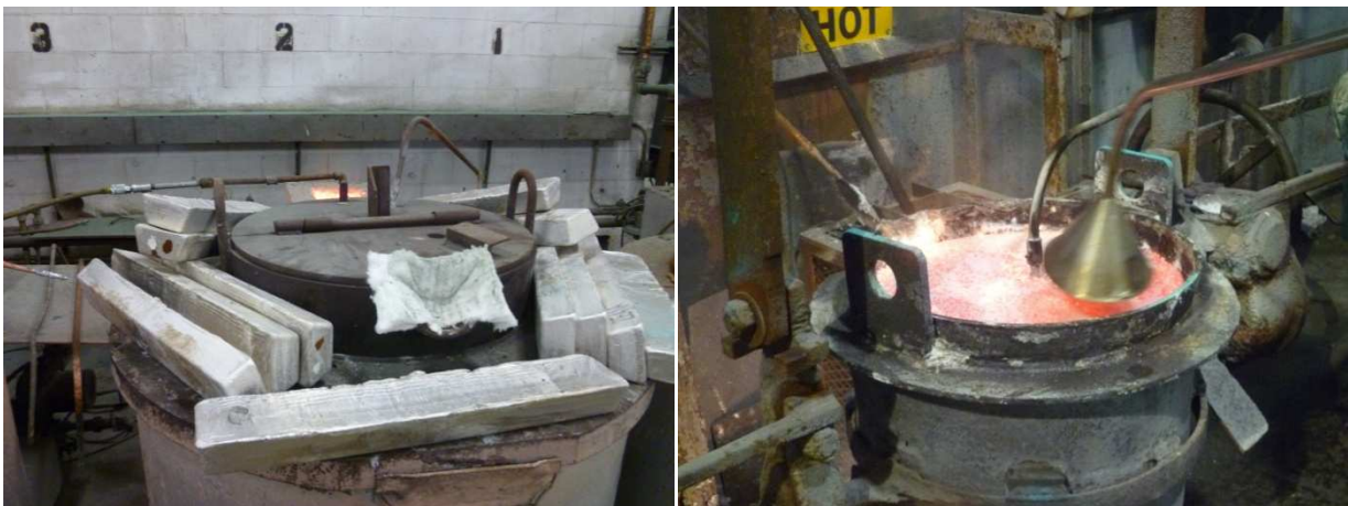
Figure 14: Crucible with hinged lid and open crucible with inverted funnel and diffuser.
