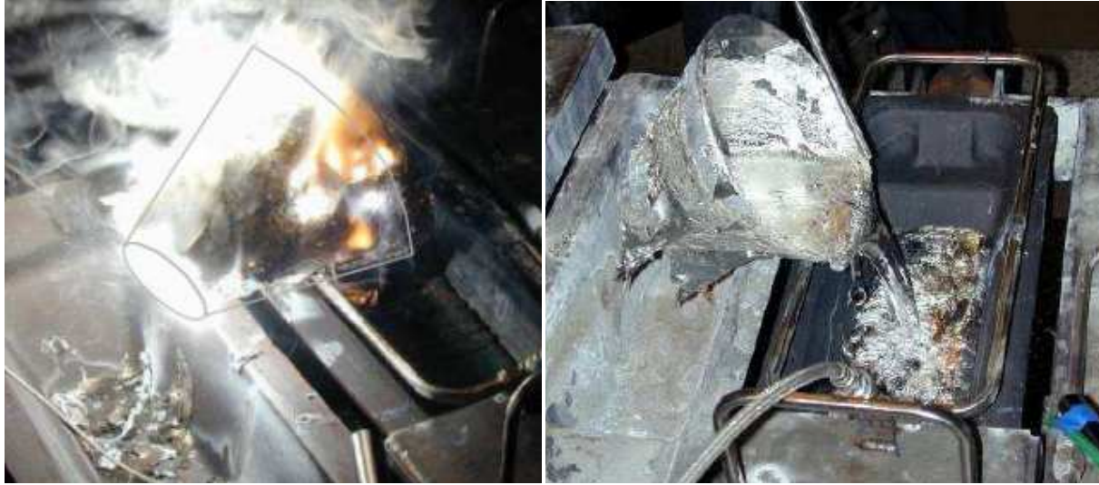
Figure 3: Examples of unprotected and protected magnesium pouring. The figure on the left has significant amounts of magnesium oxide formation (smoke and flaring) and the figure on the right shows properly protected pouring. Courtesy Dean Milbrath.
