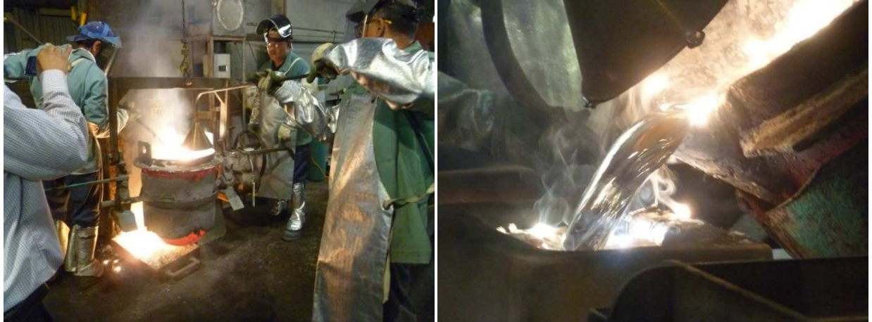
Figure 18: Open crucible with inverted funnels with diffusers. On the left, note the smoke emanating from the molten metal indicating less than optimal coverage. On the right, pouring the metal in the mold. Note the bright spots indicating oxidation on the surface of the metal.
