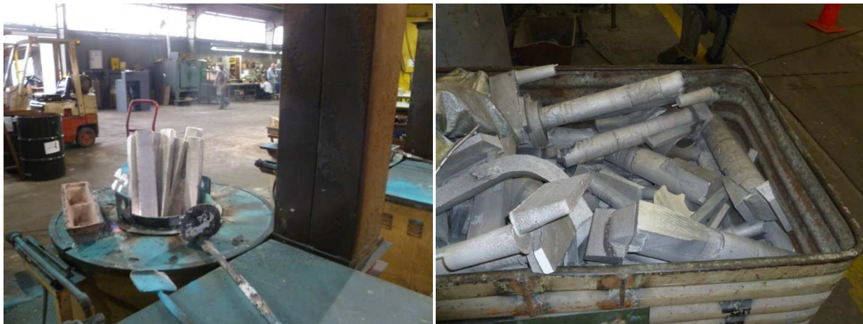
Figure 12: Furnace charged with ingot and remelt alloy ready to load in furnace.
