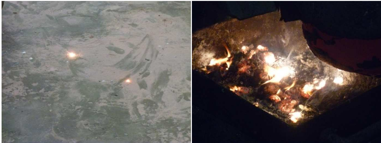
Figure 4: Surfaces of molten magnesium showing oxidation. On left, surface film on molten magnesium with bright spots indicating minor oxidation. On the right, molten magnesium without protection in a small pan.
