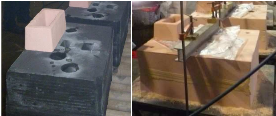
Figure 10: Sand molds used in the experiment. Green (the black ones in color) sand molds on the left and dry sand (tan in color) molds on the right.
