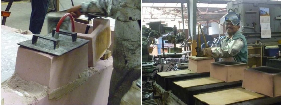
Figure 15: Molds being purged with cover gas. When only one or few molds are poured at one time, it is possible to flush the molds shortly before pouring.
