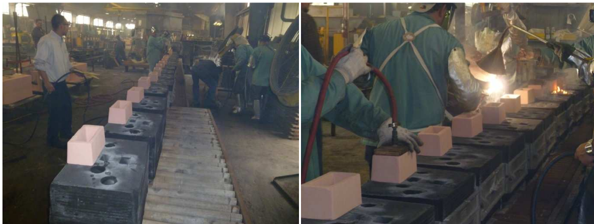
Figure 16: A row of 18 molds being poured from a single heat. Note that the mold flushing was done just ahead of the pour.
